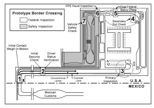
At the exit from the secondary (detailed) inspection area, the status of all inspections is checked electronically at this station. The vehicle is tracked to ensure compliance and if it has <u>not</u> been cleared to exit, signing at Station 4 will instruct the driver to return for further processing. This station will ensure that vehicles routed into the secondary inspection area have had their record cleared by those inspectors sent to examine that vehicle.
