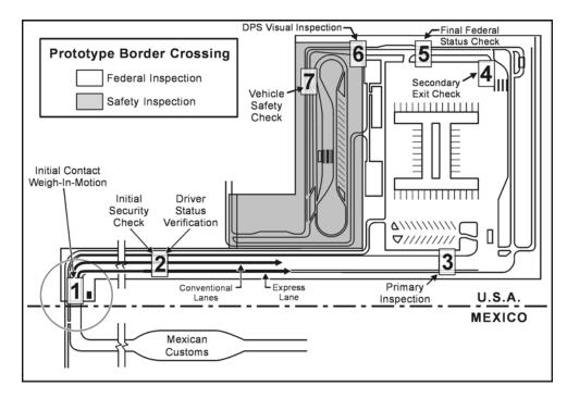
Initial contact with the vehicle is made at the station, the vehicle is identified and its electronic file activated, the vehicle is weighed by a weigh-in-motion system. If overweight the file is flagged for further processing by appropriate agencies. (Ideally, this station would be upstream of the Mexican export station to screen out overloaded vehicles before they cross the border.)
