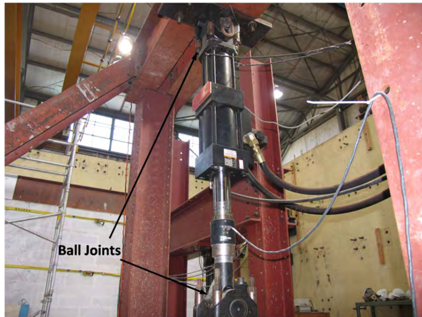
Figure 2.4: MTS 55-kip Hydraulic Actuator
