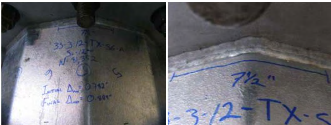
Figure 7.4: Crack Length at Bend 5 on the Galvanized Specimen after 81,326 Cycles
