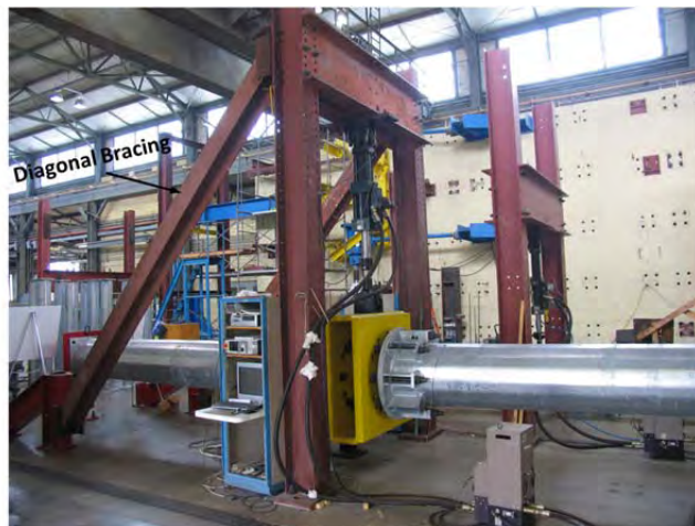
Figure 2.3: Portal Loading Frame High-mast and Mast Arm Tests
