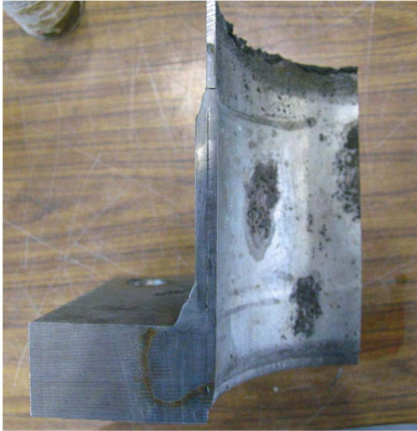
Figure 3.8: A Cross Section of a Typical External Collar Detail
