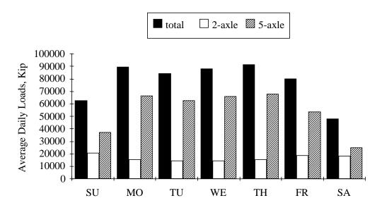
Figure 6.3 Axle Loads by Day of Week, South Site, Right Lane 1 kip = 0.4536 Mg
