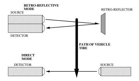
**Figure 2.1 Infrared Sensing Modes**
