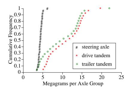
Figure 6.17 Cumulative Frequency Distribution for 3S2 Axle-group Loads, 12 March 1993, North Site, Right Lane
