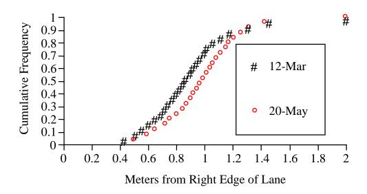
Figure 7.7 Lateral Position of Five-axle Vehicles, Right Lane 1 ft = 0.3048 m
