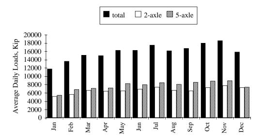
Figure 6.6 Axle Load by Month, North Site, Left Lane 1 kip = 0.4536 Mg
