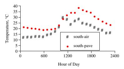
Figure 8.4 Hourly Temperature, 21 May 1993, South Site  ${}^{\circ}F = 32 + 1.8 {}^{\circ}C$
