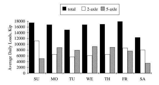
Figure 6.4 Axle Loads by Day of Week, South Site, Left Lane 1 kip = 0.4536 Mg
