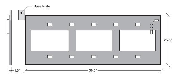
Figure 3.3 Weighpad Frame with Base Plate for Infrared Source
