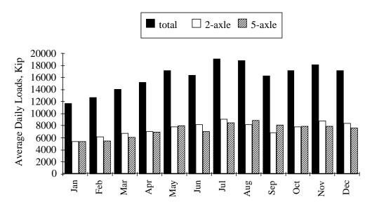
Figure 6.8 Axle Load by Month, South Site, Left Lane 1 kip = 0.4536 Mg
