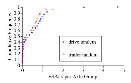
Figure 6.18 Cumulative Frequency Distribution for 3S2 Axle-group ESALs, 12 March 1993, North Site, Right Lane
