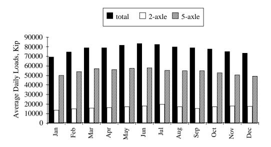
Figure 6.7 Axle Load by Month, South Site, Right Lane 1 kip = 0.4536 Mg
