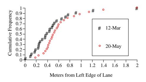
Figure 7.8 Lateral Position of Five-axle Vehicles, Left Lane  $1\ \mathrm{ft} = 0.3048\ \mathrm{m}$
