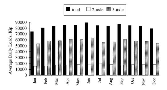
Figure 6.5 Axle Loads by Month, North Site, Right Lane 1 kip = 0.4536 Mg
