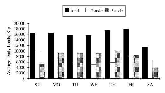
Figure 6.2 Axle Load by Day of Week, North Site, Left Lane 1 kip = 0.4536 Mg
