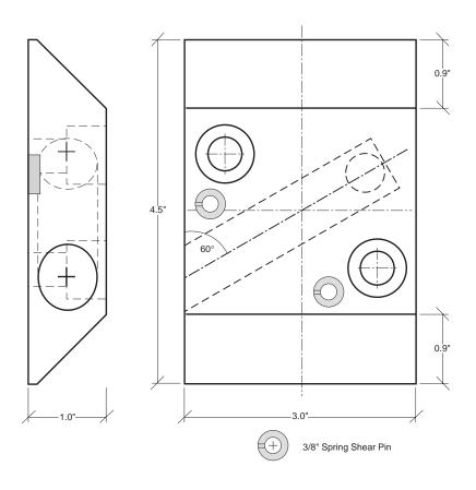
**Figure 3.1 Housing for Infrared Source**
