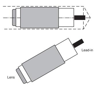
Figure 3.2 Infrared Source/Receiver Unit
