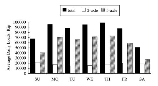
Figure 6.1 Axle Load by Day of Week, North Site, Right Lane 1 kip = 0.4536 Mg
