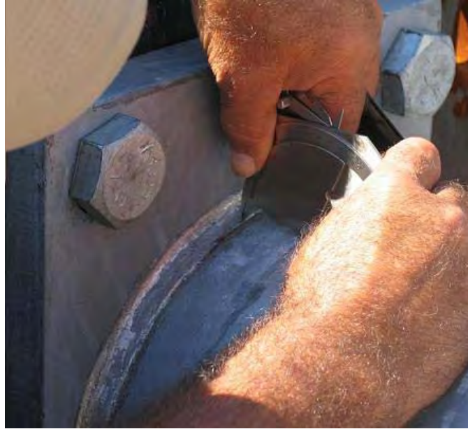
Figure 14 Measurement of UIT Application Groove Using an Undercut Measuring Device
