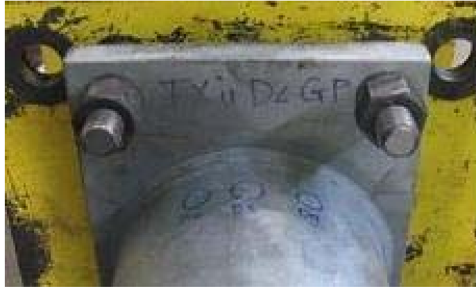
Figure 2: Location of the Middle-Most Temperature Reading Locations (Circles Labeled D2, D3, and D4; The Endmost Temperature Reading Locations are Not Visible in this Picture)
