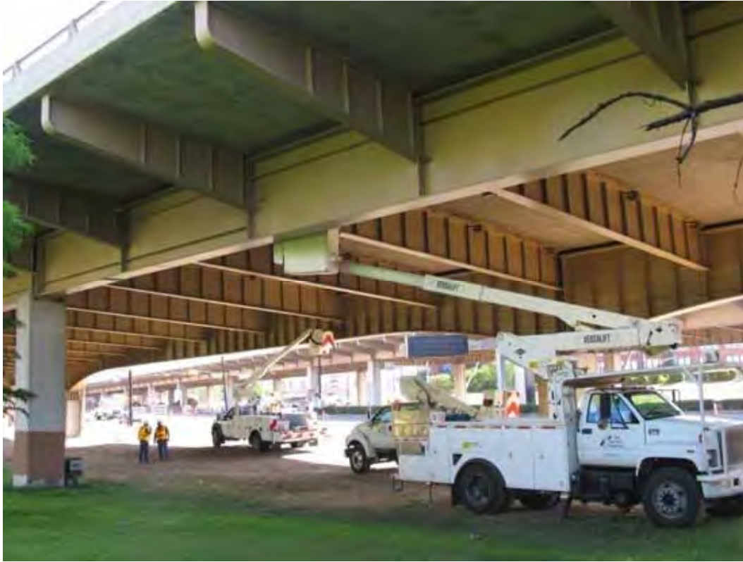
Figure 2.4: Bucket Trucks used to Place Strain Gages
