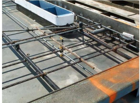
IButton temperature instrumentation (chain of three IButtons) cast into a Central Stressing Panel
