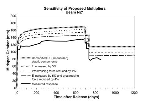
Figure 6.57 Sensitivity of camber prediction for Beam N21 using the proposed multipliers with creep based on Eq. 6.24
