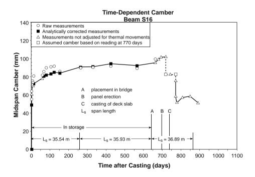
Figure 5.18 Measured midspan camber and deflection response for Beam S16
