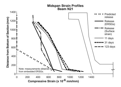
Figure 5.40 Measured strain profiles at midspan for Beam N21
