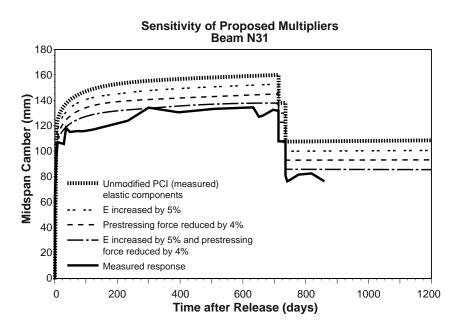
Figure 6.61 Sensitivity of camber prediction for Beam N31 using the proposed multipliers with creep based on Eq. 6.24
