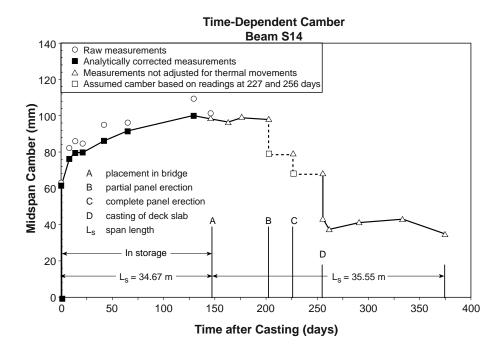
Figure 5.16 Measured midspan camber and deflection response for Beam S14
