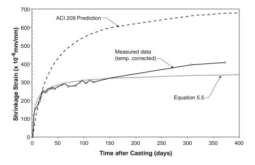
Figure 5.9 ACI prediction and proposed equation for shrinkage strain
