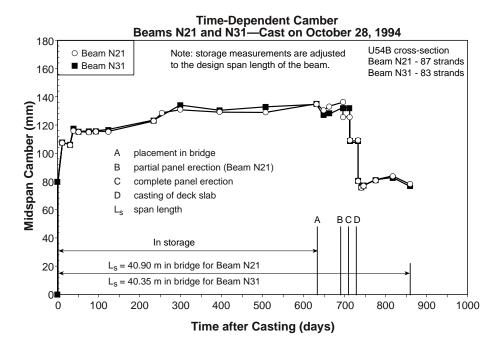
Figure 5.55 Comparison of the measured camber and deflection responses of Beams N21 and N31
