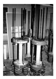
Figure 3.19 Creep test specimens sustaining applied load
