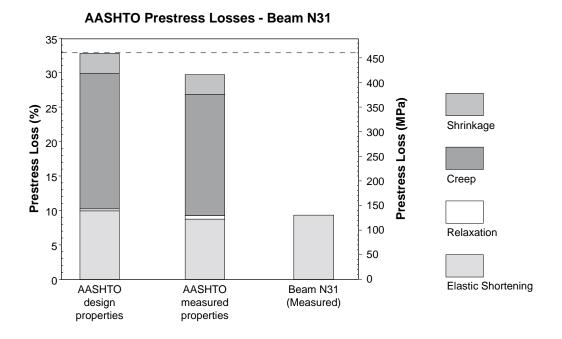
Figure 6.7 AASHTO predicted prestress losses for Beam N31
