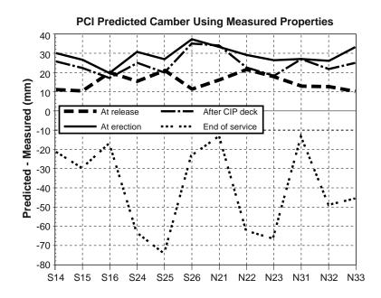
*Figure 6.30 Differences in measured and predicted long-term camber and deflection (based on measured parameters)*
