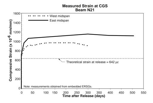
Figure 5.32 Measured prestressing strand strain at the midspan of Beam N21
