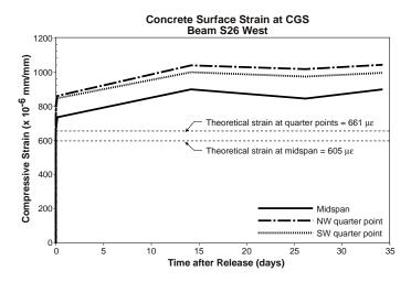
Figure 5.22 Measured surface strain at the CGS on the west side of Beam S26
