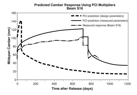
Figure 6.24 Comparison of measured and predicted camber responses for Beam S16 using the PCI Design Handbook procedures
