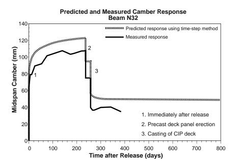
Figure 6.50 Predicted camber for Beam N32 using the time-step method
