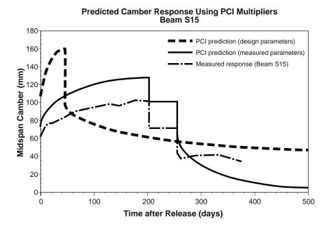
Figure 6.23 Comparison of measured and predicted camber responses for Beam S15 using the PCI Design Handbook procedures
