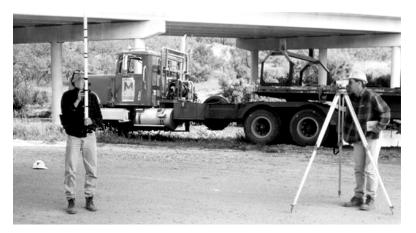
*Figure 3.17 Precise surveying system for measuring beam camber*
