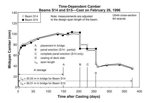
Figure 5.53 Comparison of the measured camber and deflection responses of Beams S14 and S15
