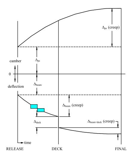
Figure 1.2 Components of time-dependent camber and deflection
