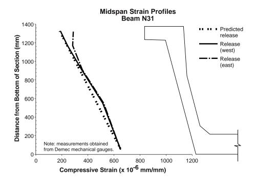
Figure 5.42 Measured strain profiles at midspan for Beam N31
