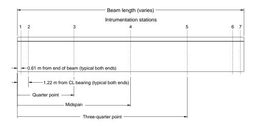
Figure 3.15 Horizontal locations for beam instrumentation
