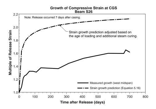
Figure 5.68 Strain growth ratio at the CGS up to panel erection for Beam S26
