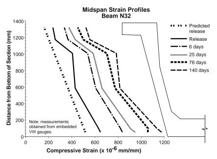
Figure 5.43 Measured strain profiles at the midspan of Beam N32
