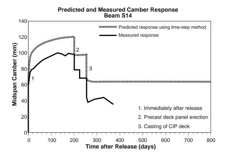
Figure 6.40 Predicted camber for Beam S14 using the time-step method
