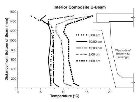
Figure 5.49 Temperature distributions at midspan for an interior composite U-beam on January 30, 1997
