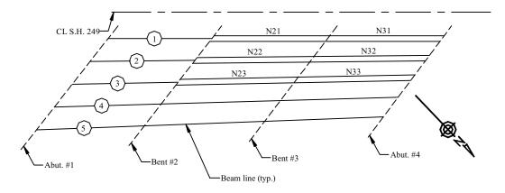
Figure 3.3 Instrumented beams in the northbound main lanes bridge
