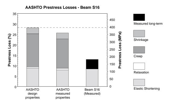
Figure 6.2 AASHTO predicted prestress losses for Beam S16
