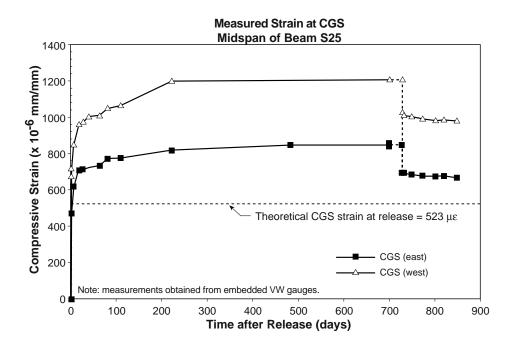
Figure 5.26 Measured prestressing strand strain at the midspan of Beam S25
