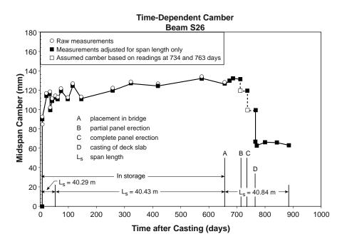
Figure 5.21 Measured midspan camber and deflection response for Beam S26
