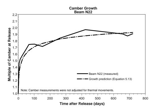
Figure 5.60 Camber growth ratios up to panel erection for Beam N22
