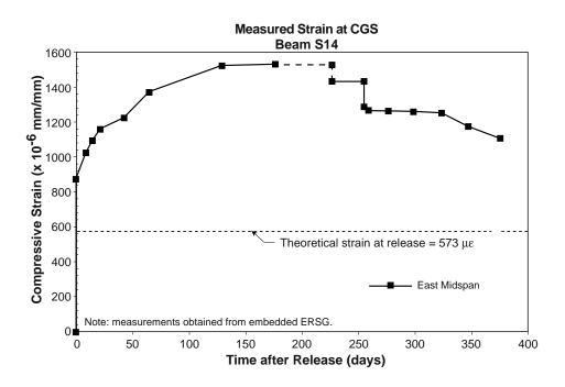
Figure 5.29 Measured prestressing strand strain at the midspan of Beam S14
