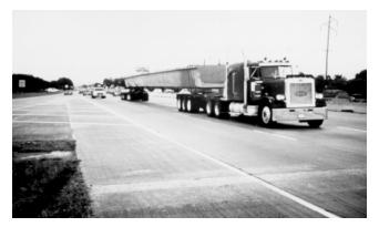
Figure 4.6 U-beam being transported to the job site
