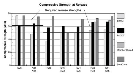
Figure 5.1 Compressive strength at release for HPC U-beams
