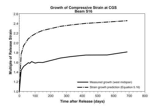
Figure 5.66 Strain growth ratio at the CGS up to panel erection for Beam S16
