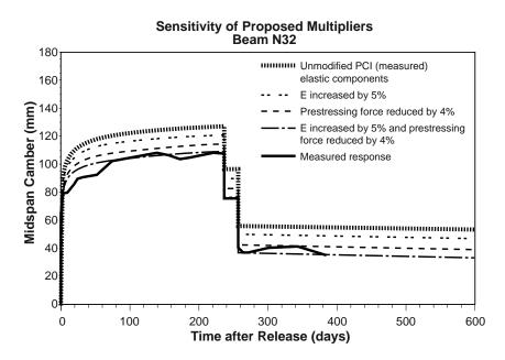
Figure 6.63 Sensitivity of camber prediction for Beam N32 using the proposed multipliers with creep based on Eq. 6.24
