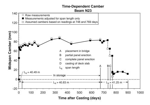
Figure 5.12 Measured midspan camber and deflection response for Beam N23
