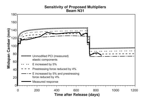
Figure 6.62 Sensitivity of camber prediction for Beam N31 using the proposed multipliers with creep based on Eq. 6.38
