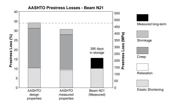
Figure 6.5 AASHTO predicted prestress losses for Beam N21
