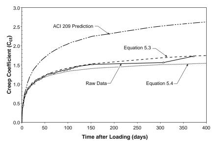
Figure 5.8 ACI prediction and proposed equations for creep coefficient
