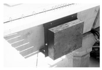
Figure 4.9 Data acquisition system (DAS) box mounted in the bridge
