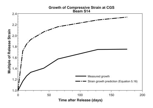
Figure 5.64 Strain growth ratio at the CGS up to panel erection for Beam S14
