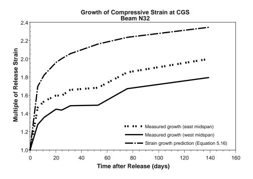
Figure 5.69 Strain growth ratio at the CGS up to panel erection for Beam N32
