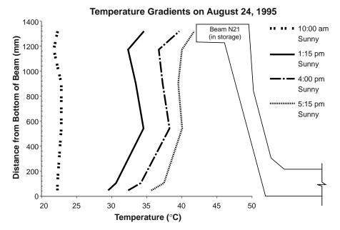
*Figure 5.45 Temperature distributions at midspan on a hot summer day*
