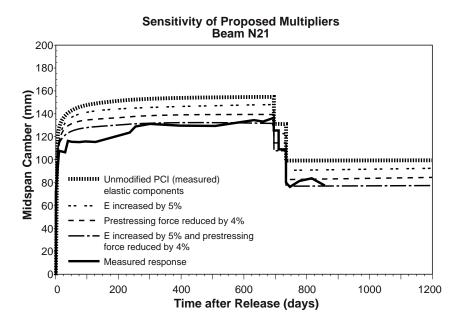
Figure 6.58 Sensitivity of camber prediction for Beam N21 using the proposed multipliers with creep based on Eq. 6.38
