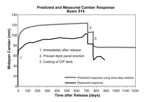
Figure 6.42 Predicted camber for Beam S16 using the time-step method
