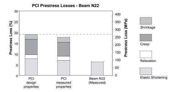
Figure 6.16 PCI predicted prestress losses for Beam N22
