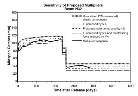
Figure 6.64 Sensitivity of camber prediction for Beam N32 using the proposed multipliers with creep based on Eq. 6.38
