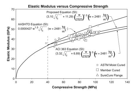
Figure 5.6 Proposed equation for elastic modulus for HPC U-beams
