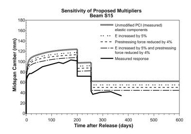
Figure 6.53 Sensitivity of camber prediction for Beam S15 using the proposed multipliers with creep based on Eq. 6.24
