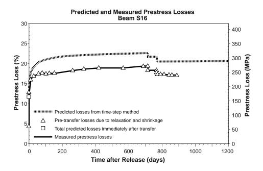
Figure 6.33 Predicted prestress losses for Beam S16 (time-step method)
