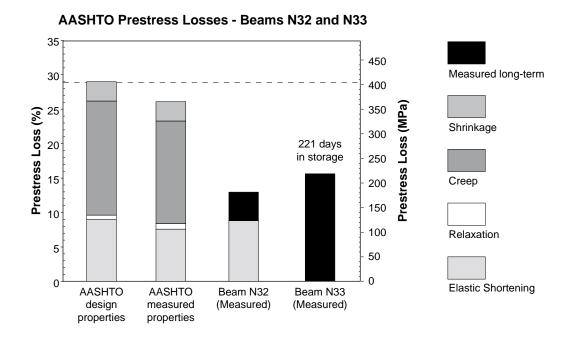
Figure 6.8 AASHTO predicted prestress losses for Beams N32 and N33
