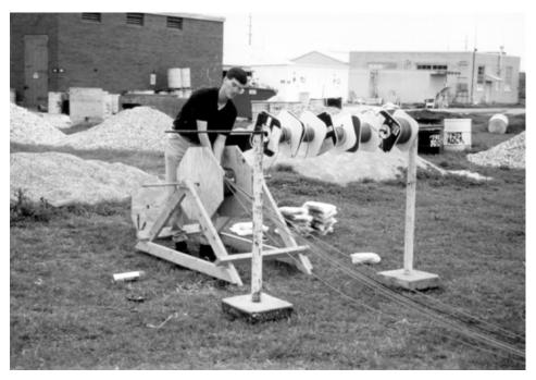
Figure 4.1 Spooling system used to gather gage lead wires
