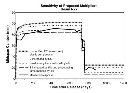
Figure 6.60 Sensitivity of camber prediction for Beam N22 using the proposed multipliers with creep based on Eq. 6.38
