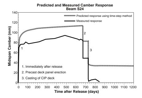
Figure 6.43 Predicted camber for Beam S24 using the time-step method
