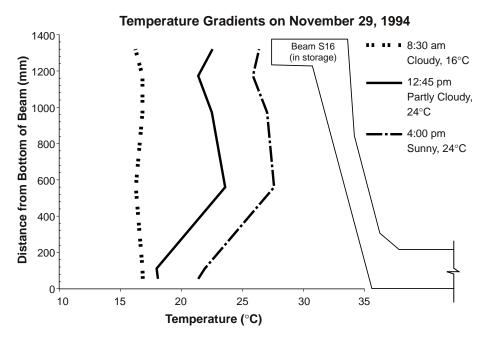
Figure 5.44 Temperature distributions at midspan on a mostly cloudy fall day
