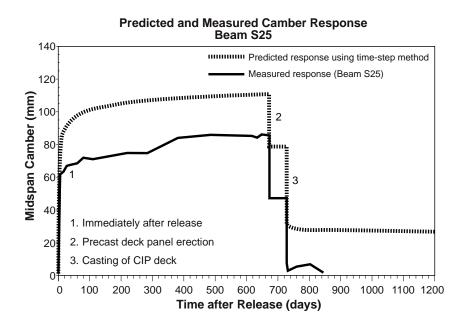
Figure 6.44 Predicted camber for Beam S25 using the time-step method
