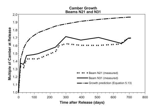
Figure 5.56 Camber growth ratios up to panel erection for Beams N21 and N31
