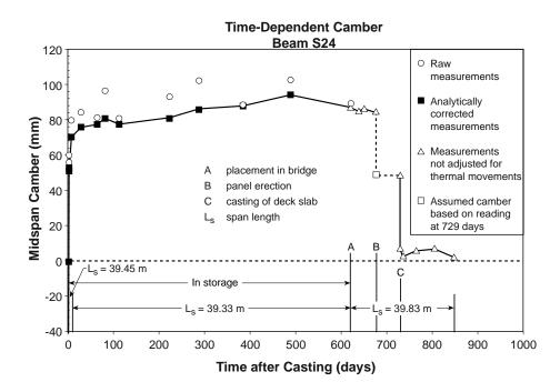
Figure 5.19 Measured midspan camber and deflection response for Beam S24
