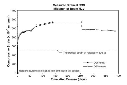
Figure 5.28 Measured prestressing strand strain at the midspan of Beam N32
