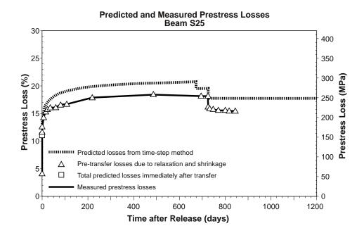
Figure 6.34 Predicted prestress losses for Beam S25 (time-step method)
