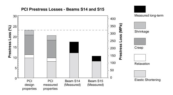
Figure 6.11 PCI predicted prestress losses for Beams S14 and S15
