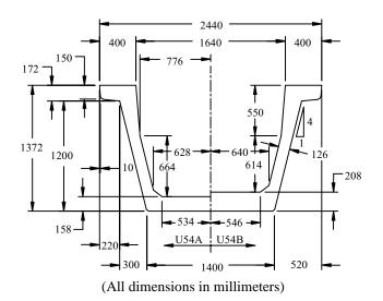
Figure 3.4 Cross-section dimensions for Texas U54 beam
