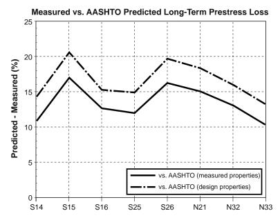
Figure 6.10 Summary of the differences in measured and AASHTO predicted long-term prestress losses
