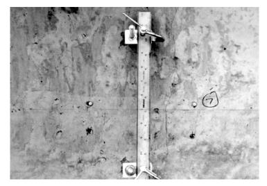
Figure 4.3 External instrumentation placed at midspan of a beam
