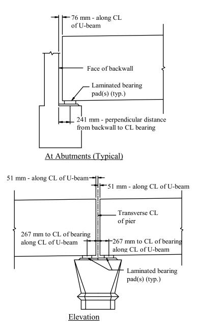
*Figure 3.8 Typical bearing details for instrumented beams in both bridges*
