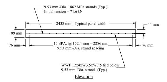
Figure 3.7 Precast deck panel details
