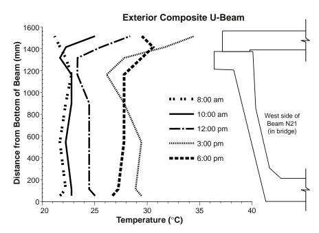
Figure 5.46 Temperature distributions at midspan for an exterior composite U-beam on March 10, 1997
