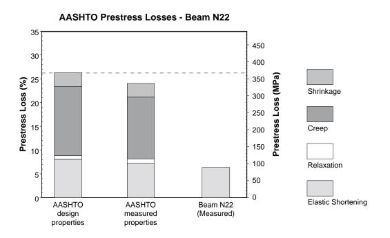
Figure 6.6 AASHTO predicted prestress losses for Beam N22
