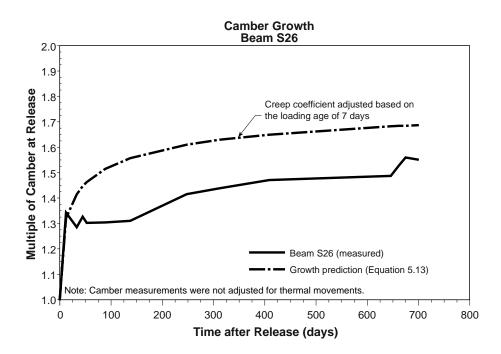
Figure 5.63 Camber growth ratios up to panel erection for Beam S26
