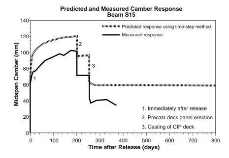
Figure 6.41 Predicted camber for Beam S15 using the time-step method
