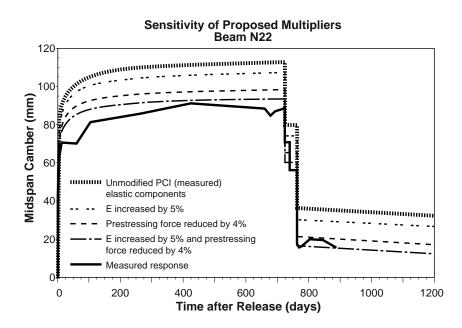
Figure 6.59 Sensitivity of camber prediction for Beam N22 using the proposed multipliers with creep based on Eq. 6.24
