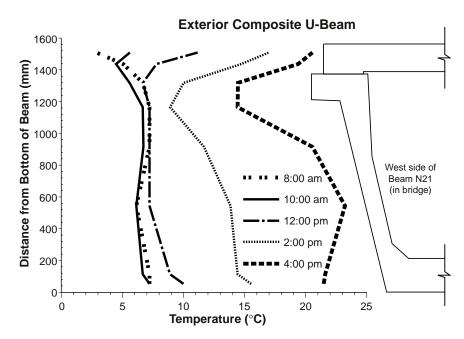
Figure 5.48 Temperature distributions at midspan for an exterior composite U-beam on January 30, 1997
