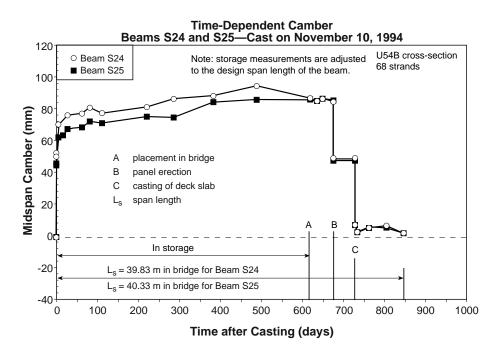
Figure 5.54 Comparison of the measured camber and deflection responses of Beams S24 and S25
