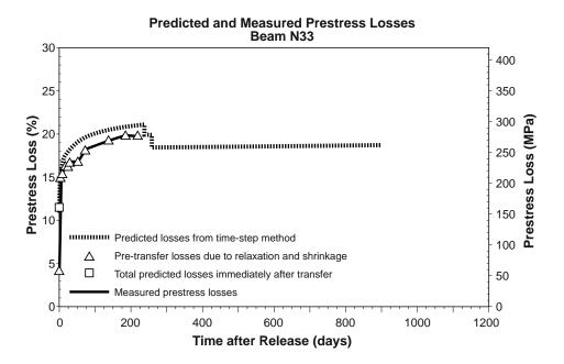
Figure 6.38 Predicted prestress losses for Beam N33 (time-step method)
