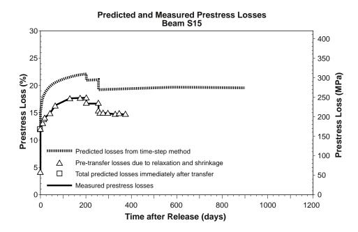
Figure 6.32 Predicted prestress losses for Beam S15 (time-step method)
