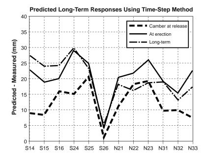
*Figure 6.52 Summary of differences between measured and predicted long-term camber and deflection based on the time-step method*
