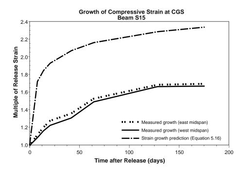
Figure 5.65 Strain growth ratio at the CGS up to panel erection for Beam S15
