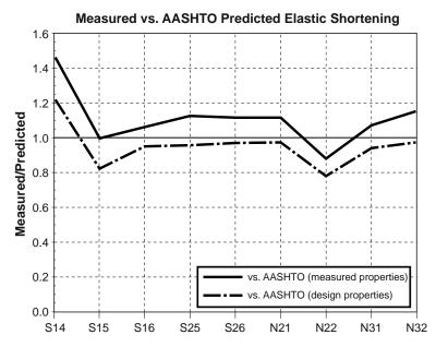
Figure 6.9 Summary of the ratios of measured to AASHTO predicted prestress losses at release
