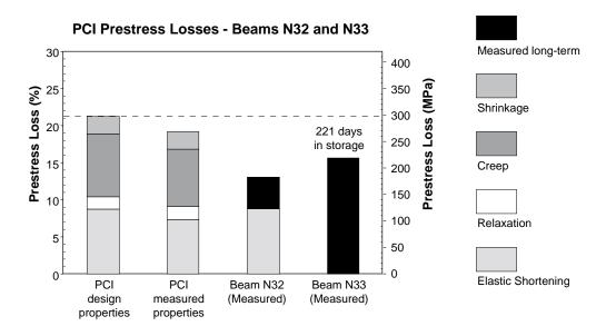
Figure 6.18 PCI predicted prestress losses for Beams N32 and N33
