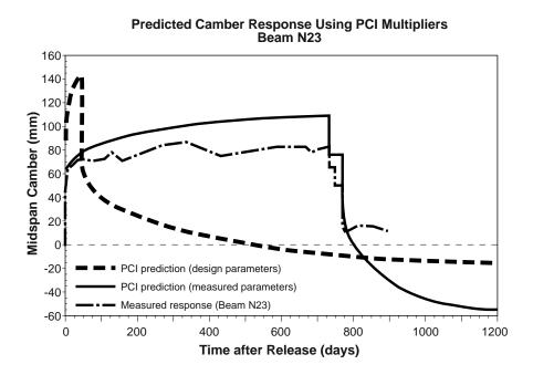
Figure 6.27 Comparison of measured and predicted camber responses for Beam N23 using the PCI Design Handbook procedures
