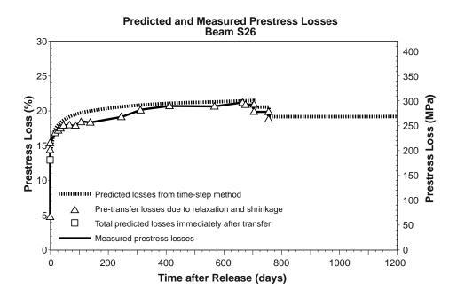
Figure 6.35 Predicted prestress losses for Beam S26 (time-step method)
