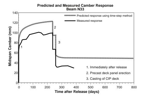
Figure 6.51 Predicted camber for Beam N33 using the time-step method
