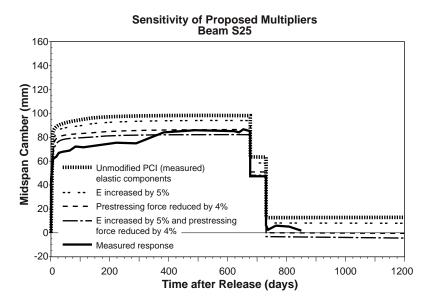
Figure 6.56 Sensitivity of camber prediction for Beam S25 using the proposed multipliers with creep based on Eq. 6.38
