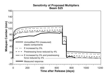
Figure 6.55 Sensitivity of camber prediction for Beam S25 using the proposed multipliers with creep based on Eq. 6.24
