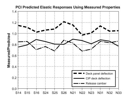
Figure 6.22 Summary of measured elastic response ratios based on PCI Design Handbook predictions using measured properties
