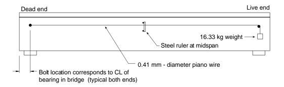
Figure 3.16 Schematic of tensioned piano wire camber and deflection measuring system
