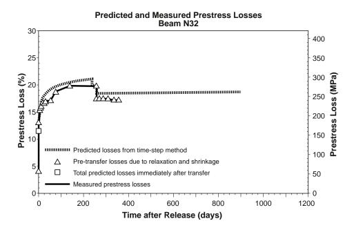
Figure 6.37 Predicted prestress losses for Beam N32 (time-step method)
