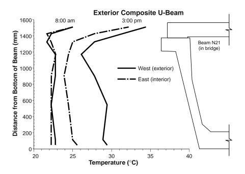
Figure 5.50 Comparison of temperature distributions at midspan for both sides of an exterior composite U-beam on March 10, 1997
