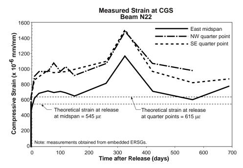
Figure 5.33 Measured prestressing strand strain at midspan and quarter points of Beam N22
