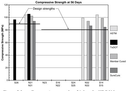
Figure 5.3 Compressive strength at 56 days for HPC U-beams
