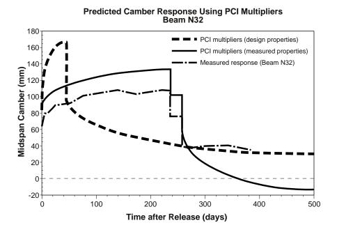
Figure 6.28 Comparison of measured and predicted camber responses for Beam N32 using the PCI Design Handbook procedures
