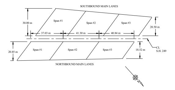
Figure 3.1 Plan view of Louetta Road Overpass
