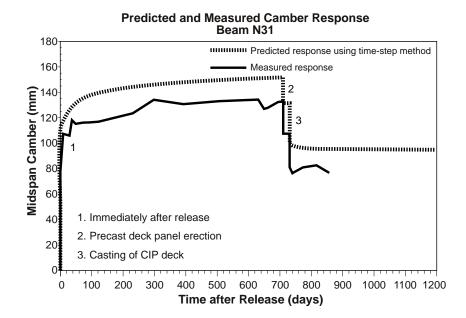
Figure 6.49 Predicted camber for Beam N31 using the time-step method
