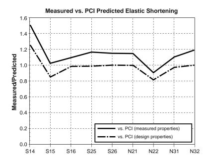
Figure 6.19 Summary of the ratios of measured to PCI predicted prestress losses due to elastic shortening
