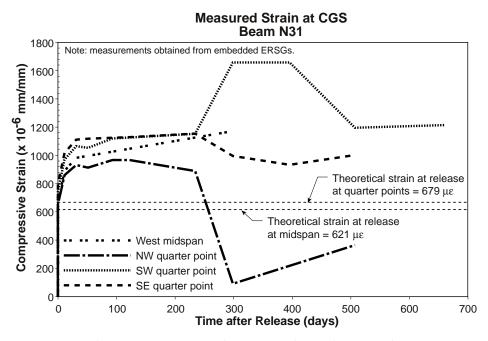
Figure 5.34 Measured prestressing strand strain at the midspan and quarter points of Beam N31
