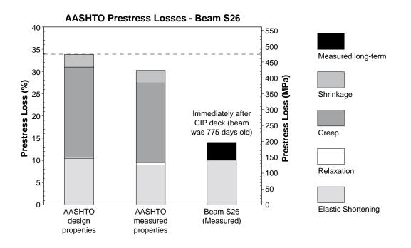
Figure 6.4 AASHTO predicted prestress losses for Beam S26
