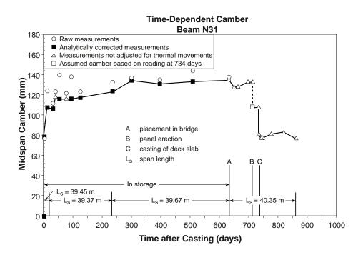
Figure 5.13 Measured midspan camber and deflection response for Beam N31
