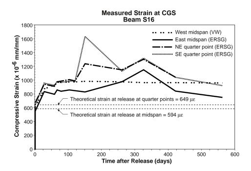
Figure 5.30 Measured prestressing strand strain at the midspan and quarter points of Beam S16
