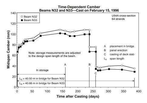
Figure 5.52 Comparison of the measured camber and deflection responses of Beams N32 and N33
