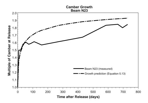
Figure 5.61 Camber growth ratios up to panel erection for Beam N23
