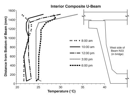
Figure 5.47 Temperature distributions at midspan for an interior composite U-beam on March 10, 1997
