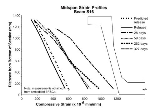
Figure 5.37 Measured strain profiles at midspan for Beam S16
