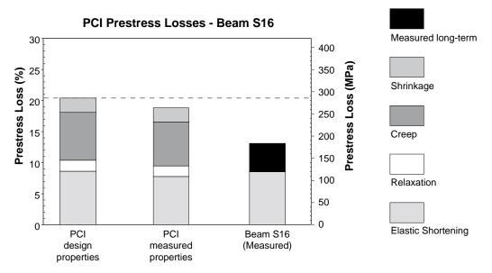
Figure 6.12 PCI predicted prestress losses for Beam S16
