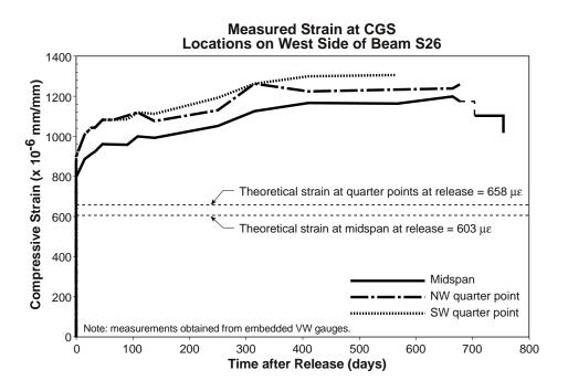
Figure 5.27 Measured prestressing strand strain at the midspan and quarter points of Beam S26
