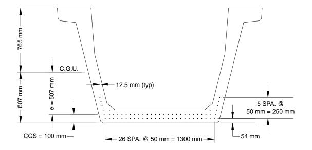
Figure 3.9 Instrumented U-beam strand pattern – 64 strands
