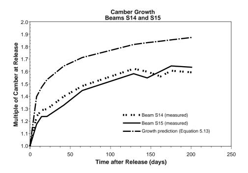
Figure 5.58 Camber growth ratios up to panel erection for Beams S14 and S15
