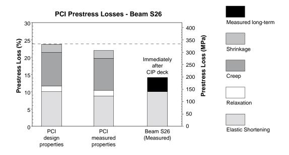
Figure 6.14 PCI predicted prestress losses for Beam S26
