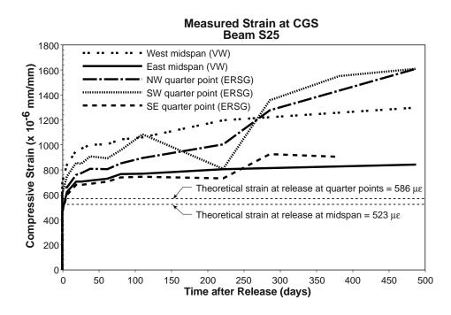
Figure 5.31 Measured prestressing strand strain at midspan and quarter points of Beam S25
