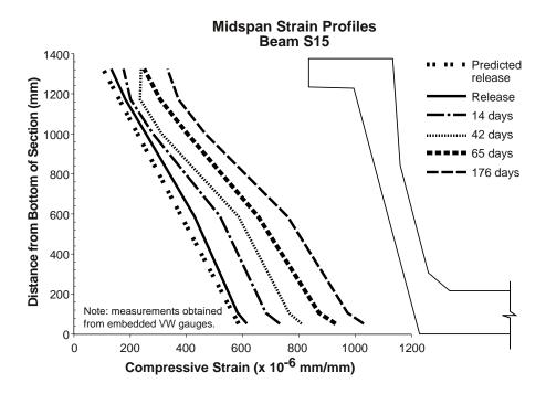
Figure 5.36 Measured strain profiles at midspan for Beam S15
