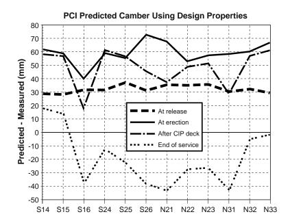
*Figure 6.29 Differences in measured and predicted long-term camber and deflection (based on design parameters)*
