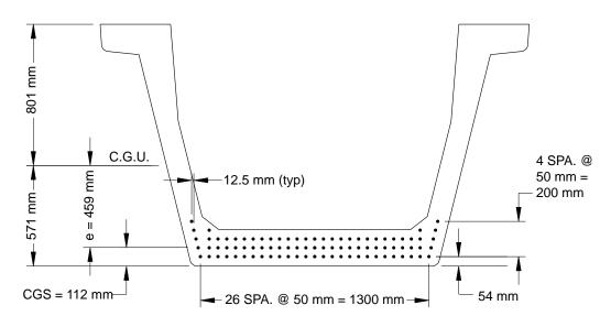
Figure 3.12 Instrumented U-beam strand pattern – 87 strands
