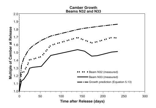
Figure 5.57 Camber growth ratios up to panel erection for Beams N32 and N33
