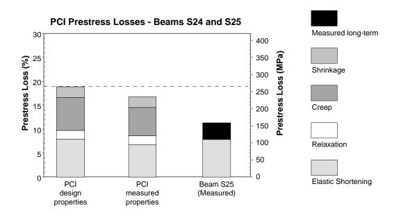
Figure 6.13 PCI predicted prestress losses for Beams S24 and S25
