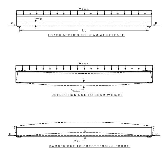
Figure 1.1 Elastic components of beam camber and deflection immediately after release
