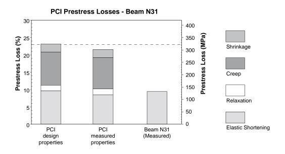
Figure 6.17 PCI predicted prestress losses for Beam N31
