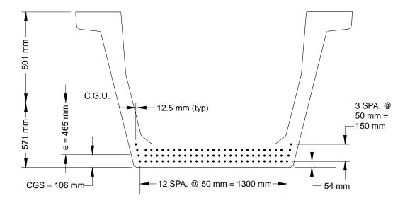
Figure 3.11 Instrumented U-beam strand pattern – 83 strands
