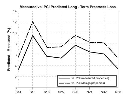
Figure 6.20 Summary of the differences in measured and PCI predicted long-term prestress losses
