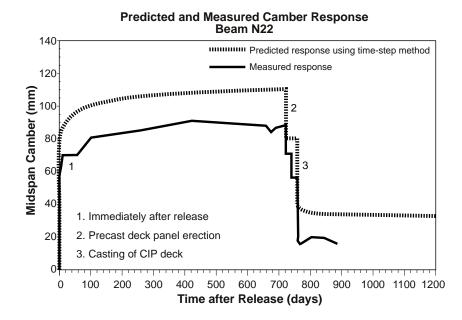
Figure 6.47 Predicted camber for Beam N22 using the time-step method
