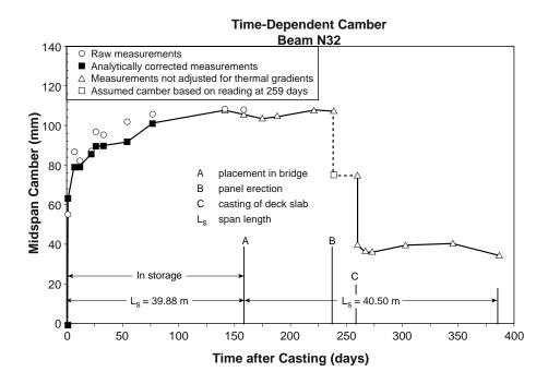
Figure 5.14 Measured midspan camber and deflection response for Beam N32
