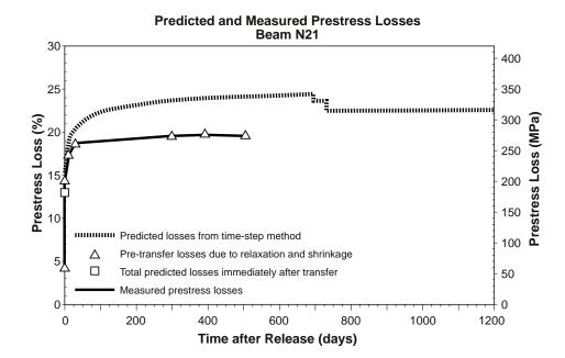
Figure 6.36 Predicted prestress losses for Beam N21 (time-step method)
