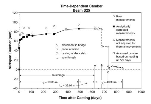
Figure 5.20 Measured midspan camber and deflection response for Beam S25
