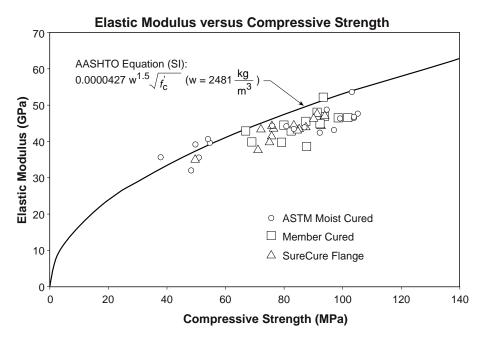
Figure 5.5 Elastic modulus versus compressive strength for HPC U-beam mix
