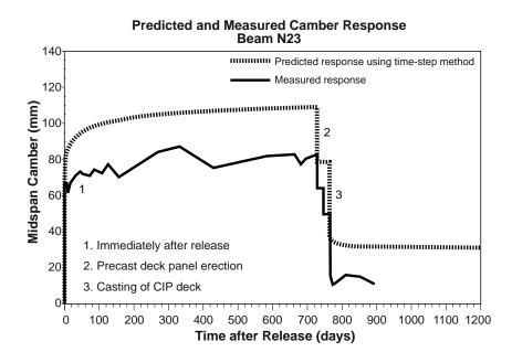
Figure 6.48 Predicted camber for Beam N23 using the time-step method
