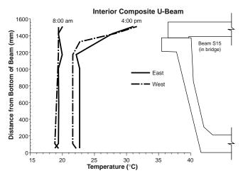
Figure 5.51 Comparison of temperature distributions at midspan for both sides of an interior composite U-beam on March 9, 1997
