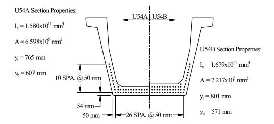
Figure 3.5 Maximum prestressing strand patterns for Texas U54 beam
