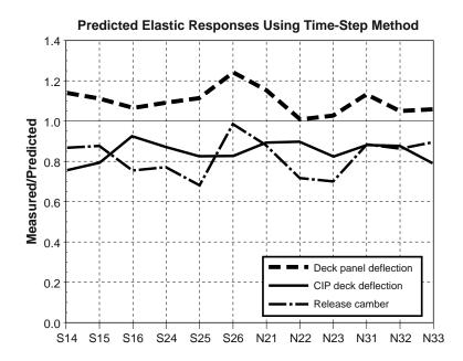
Figure 6.39 Summary of the ratios of measured to predicted elastic responses using the time-step method
