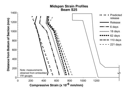
Figure 5.38 Measured strain profiles at midspan for Beam S25
