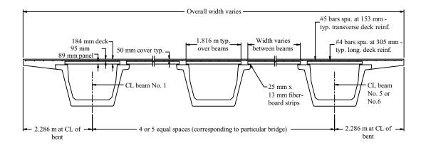
Figure 3.6 Composite U-beam cross-section details
