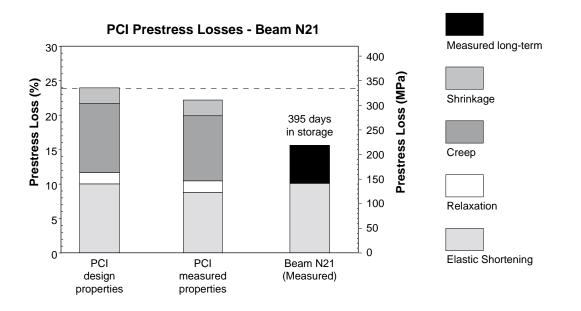
Figure 6.15 PCI predicted prestress losses for Beam N21
