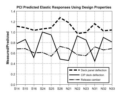
Figure 6.21 Summary of measured elastic response ratios based on PCI Design Handbook predictions using design properties
