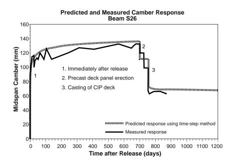
Figure 6.45 Predicted camber for Beam S26 using the time-step method
