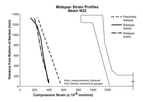
Figure 5.41 Measured strain profiles at midspan for Beam N22
