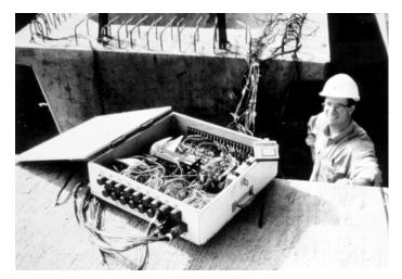
Figure 4.4 Measurements being gathered with the data acquisition system (DAS) box
