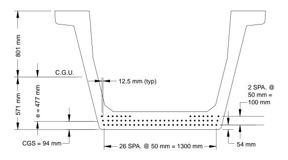
Figure 3.10 Instrumented U-beam strand pattern – 68 strands
