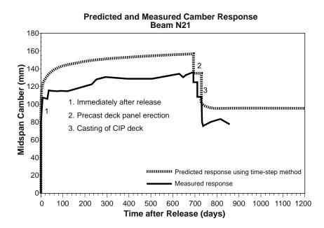
Figure 6.46 Predicted camber for Beam N21 using the time-step method
