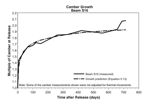
Figure 5.62 Camber growth ratios up to panel erection for Beam S16
