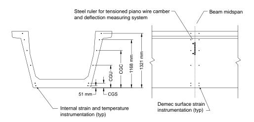
Figure 3.14 Vertical locations for beam instrumentation at midspan
