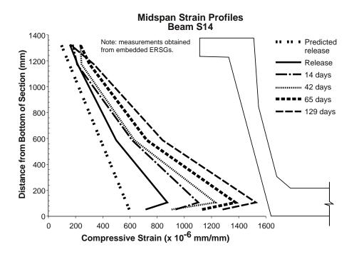
Figure 5.35 Measured strain profiles at midspan for Beam S14
