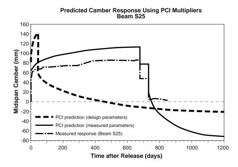
Figure 6.25 Comparison of measured and predicted camber responses for Beam S25 using the PCI Design Handbook procedures
