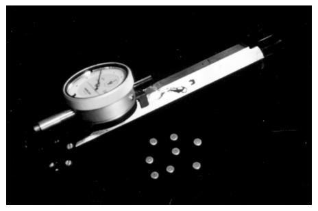
Figure 3.13 Demec surface strain measuring system
