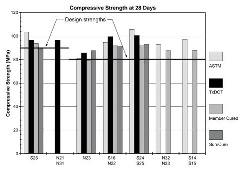
Figure 5.2 Compressive strength at 28 days for HPC U-beams
