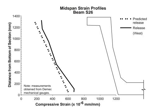
Figure 5.39 Measured strain profiles at midspan for Beam S26
