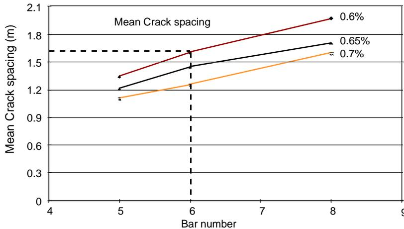
Figure 3.4 Longitudinal steel mean crack spacing sensitivity analysis
