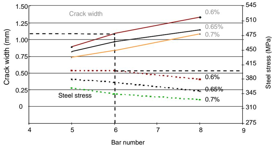
Figure 3.6 Longitudinal steel sensitivity analysis considering steel stress and crack width
