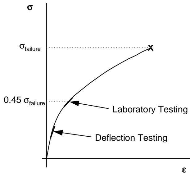
*Figure 2.1 Moduli of elasticity for coring and deflection testing*
