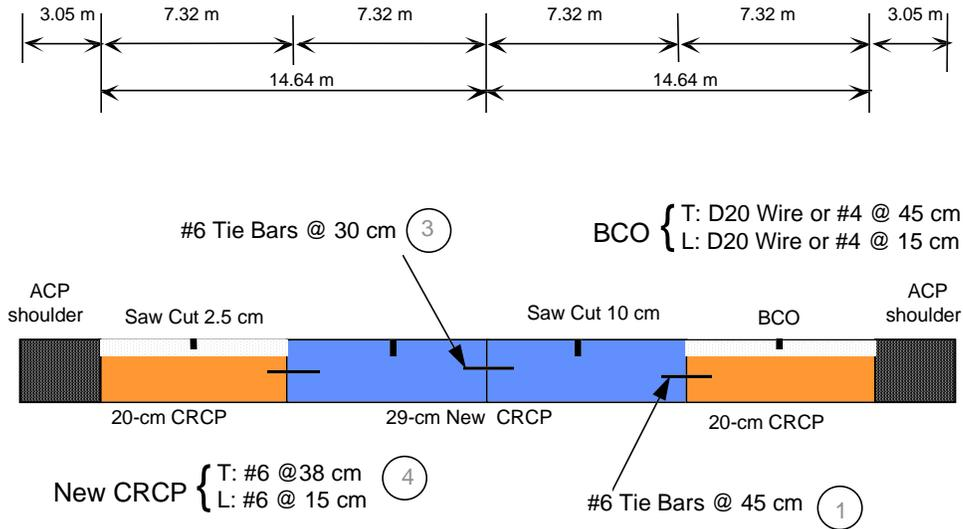
Figure 3.10 29.3-m section steel design results
