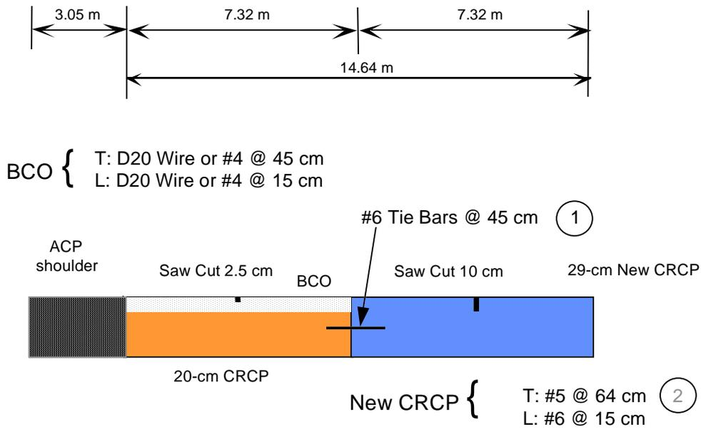
Figure 3.11 14.6-m section steel design results
