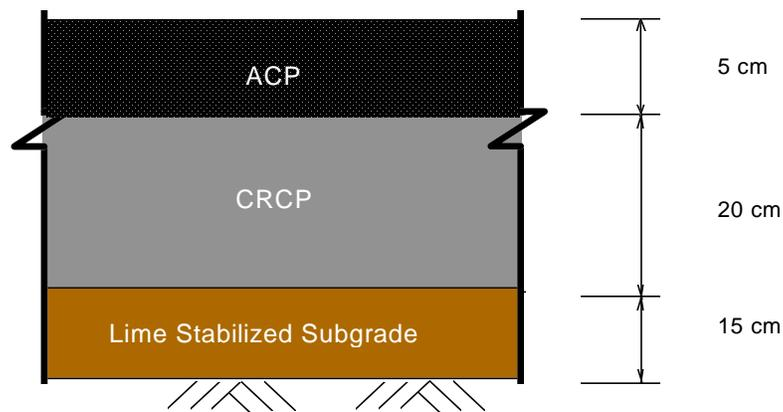
*Figure 1.1 Existing cross section*
