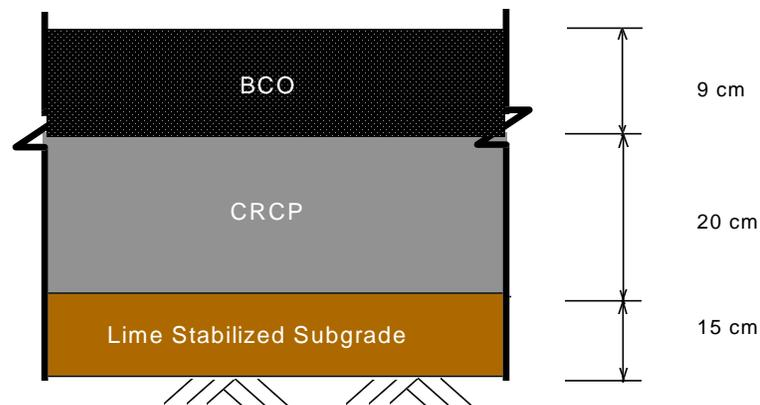
Figure 3.2 Proposed cross section for the BCO
