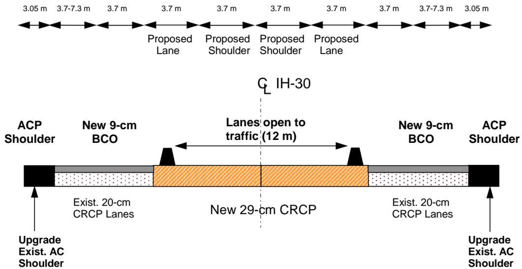
*Figure 4.3 Phase II — BCO Construction*
