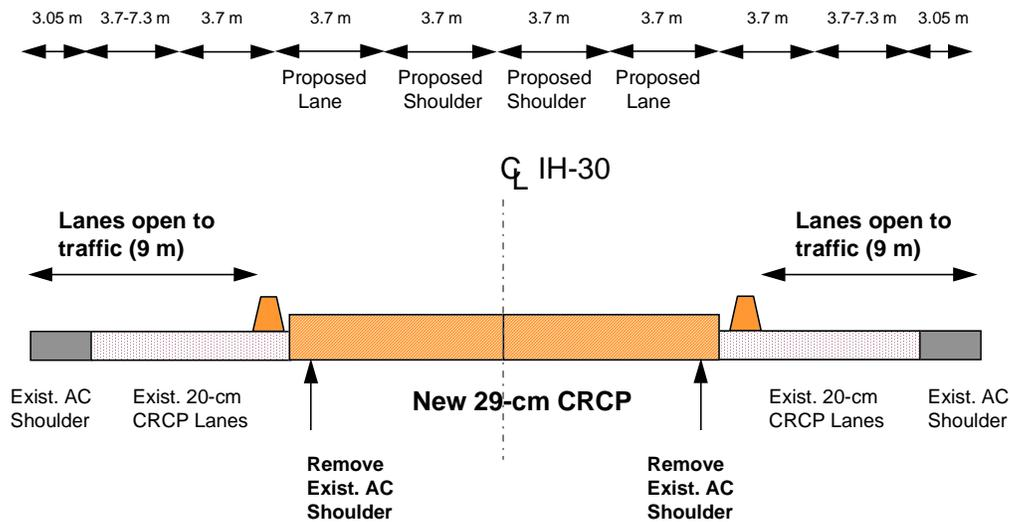
*Figure 4.2 Phase I — Construction of median section*
