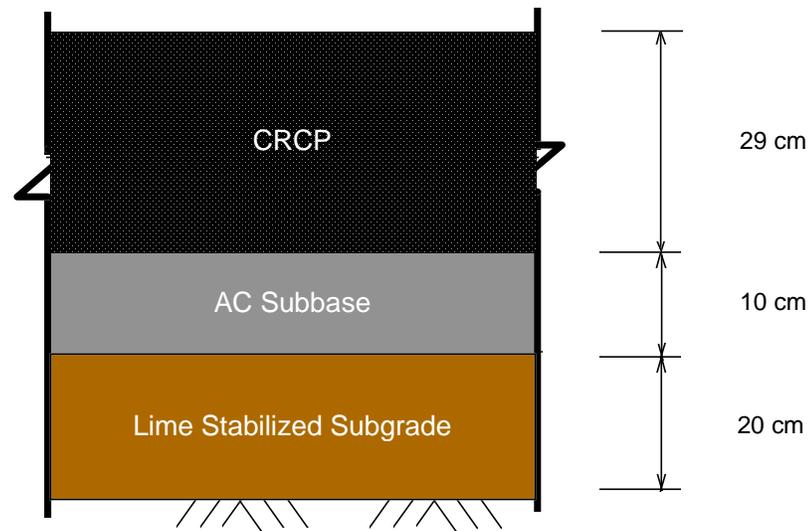
*Figure 3.3 Proposed cross section for the new CRCP*
