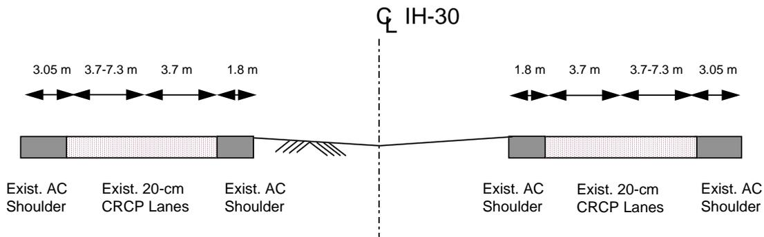
*Figure 4.1 Existing pavement cross section*
