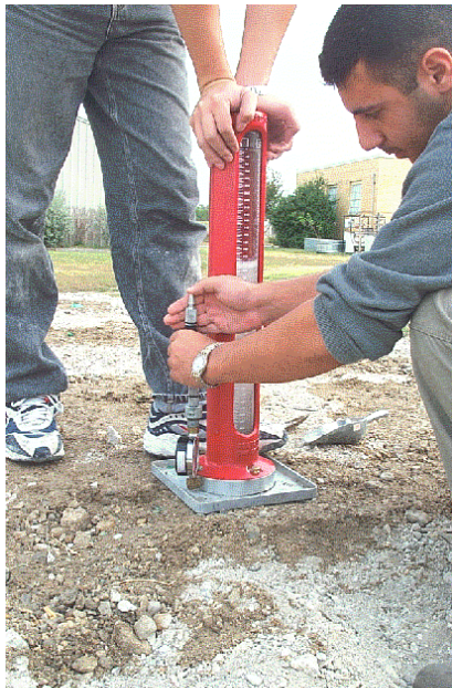
Figure 2.12 Rubber balloon test of material density.
