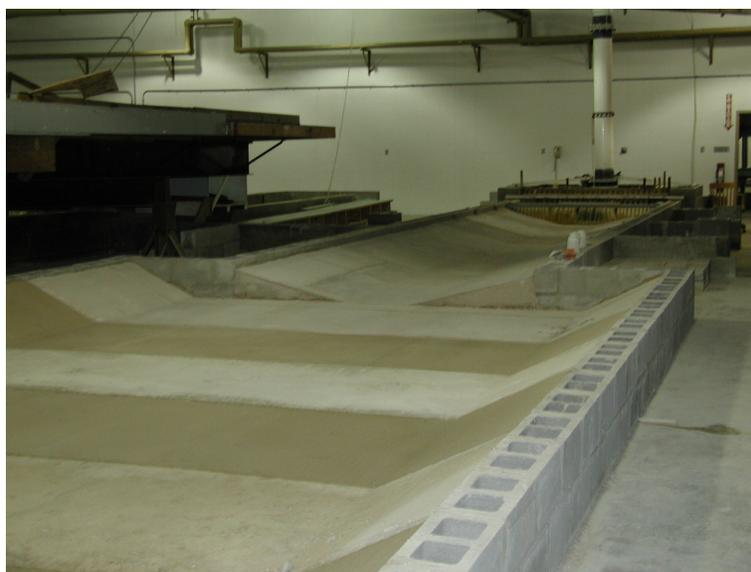
*Figure 3.4 Abrupt channel expansion looking upstream towards the headbox*
