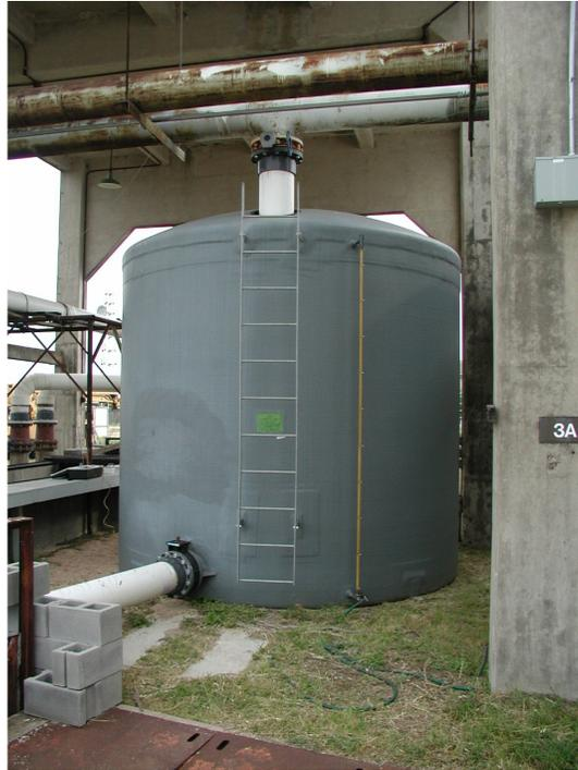
Figure 3.9 Large reservoir used for propeller meter calibration
