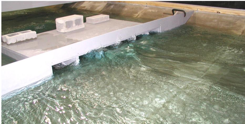
*Figure 4.11 Standing wave at culvert inlet*
