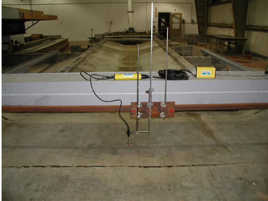
*Figure 3.7 Measurement trolley*
