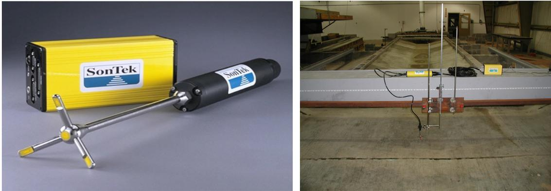
Figure 3.11 Down-looking ADV probe
