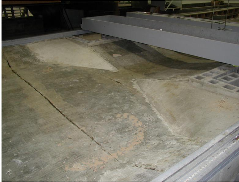
*Figure 3.5 Modified channel expansion*
