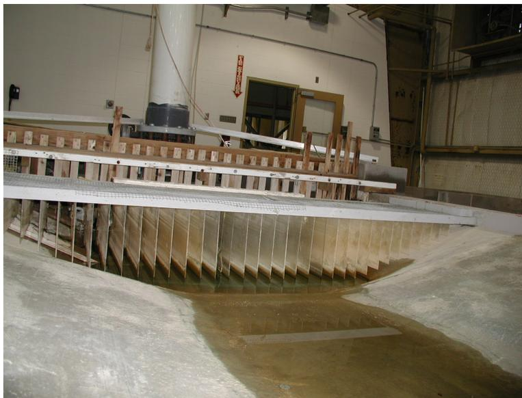
*Figure 3.3 Channel headbox and flow straighteners*
