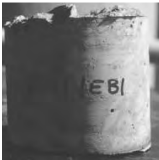
Figure 5.16 Permeability core taken from Structure #10
