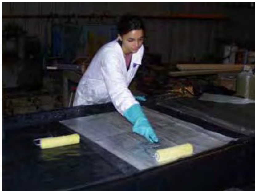
Figure 4.13 Saturating fabric with resin
