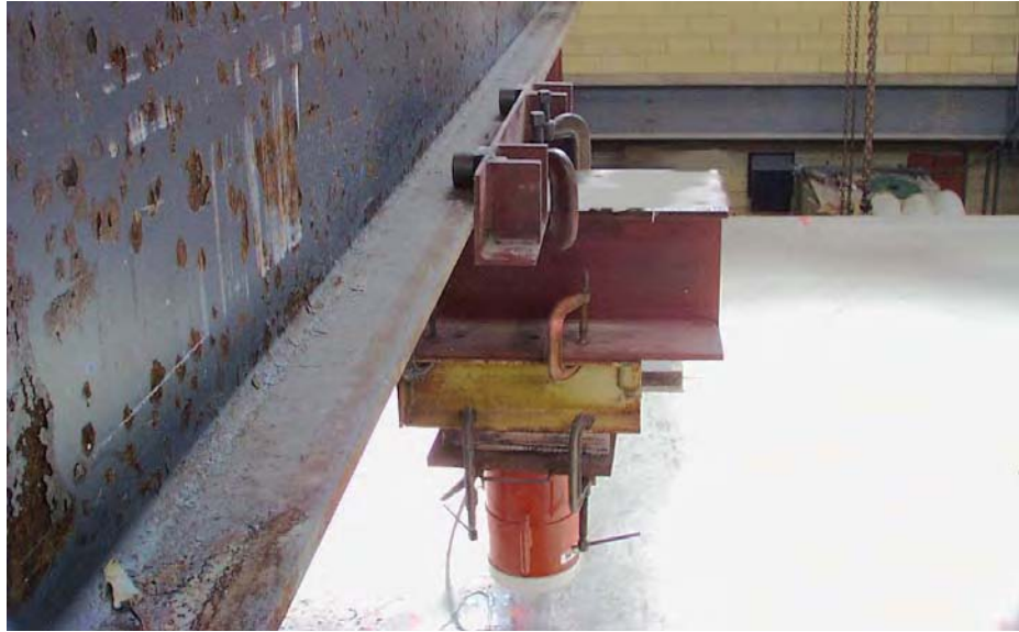
Figure 6.17 Roller attachment of actuators to load frame
