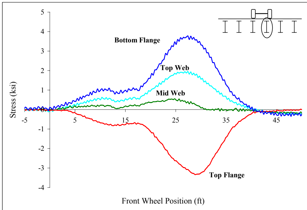
Figure B 37: Midspan stringer 3
