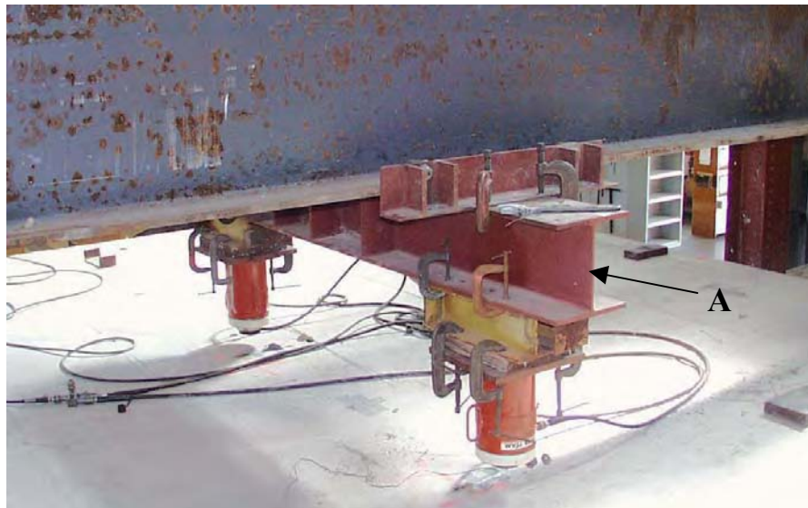
Figure 6.16 Attachment of actuators to load frame
