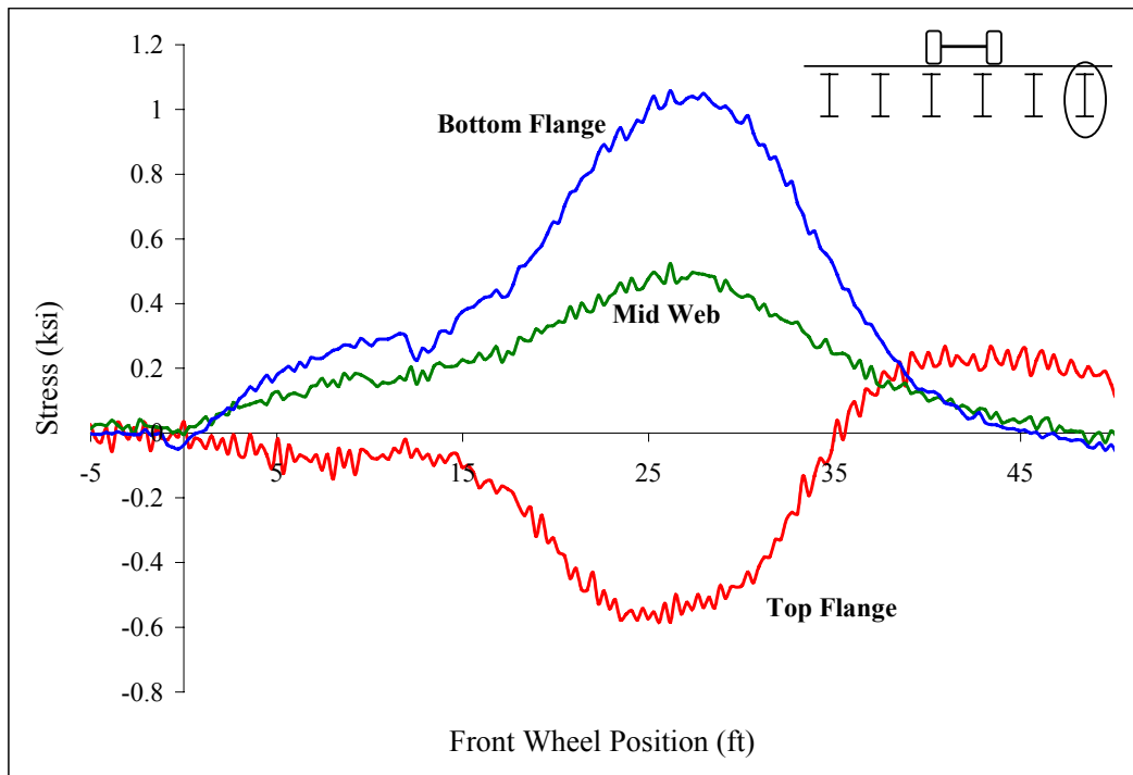
Figure A 31: Midspan stringer 1
