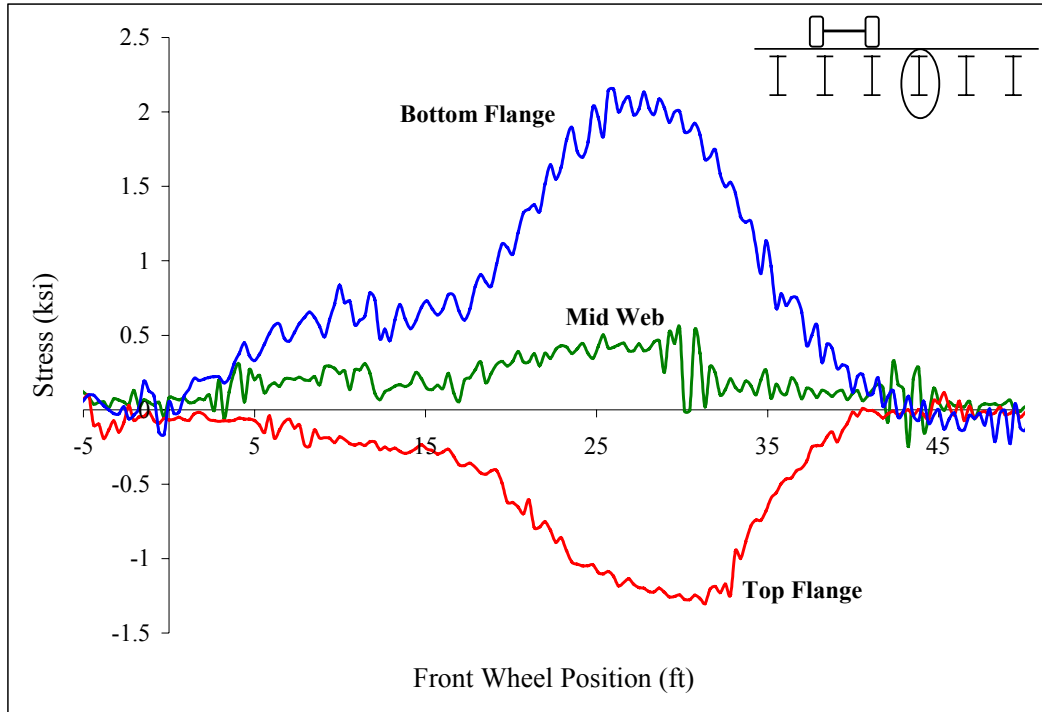
Figure B 26: Midspan stringer 3
