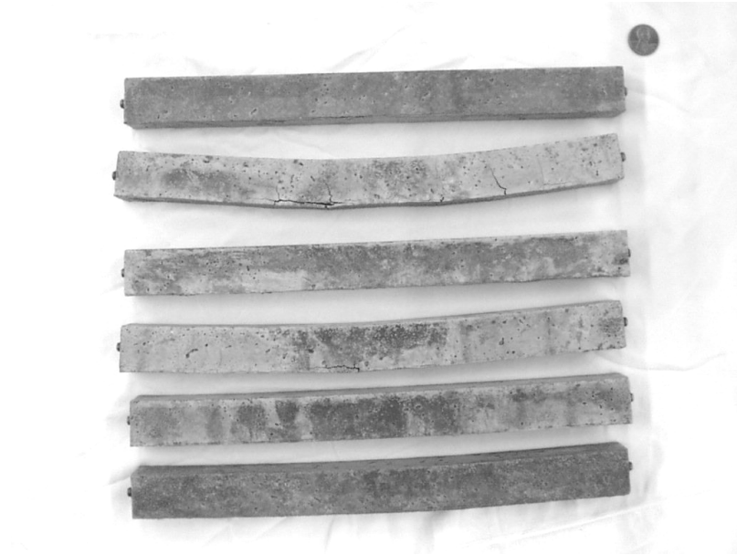
Figure 4.10 – 1FC-2 Mortar Bars after 13 Weeks of Sulfate Solution Soaking
