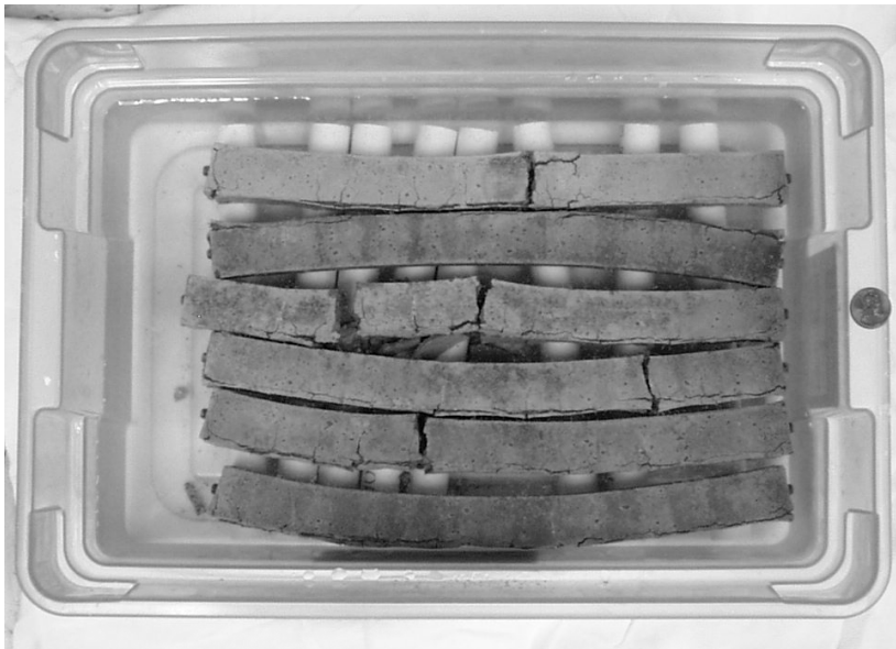
Figure 4.11 – 2FC-2 Mortar Bars after 13 Weeks of Sulfate Solution Soaking
