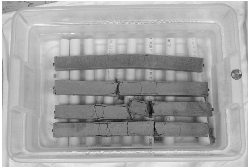
Figure 4.12 – 1C-2 Mortar Bars after 8 Weeks of Sulfate Solution Soaking
