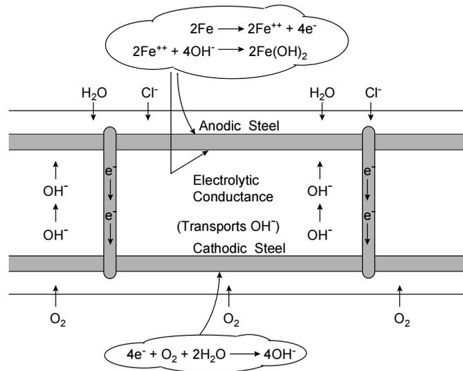
Figure 1.1 Macrocell corrosion cell in bridge deck.
