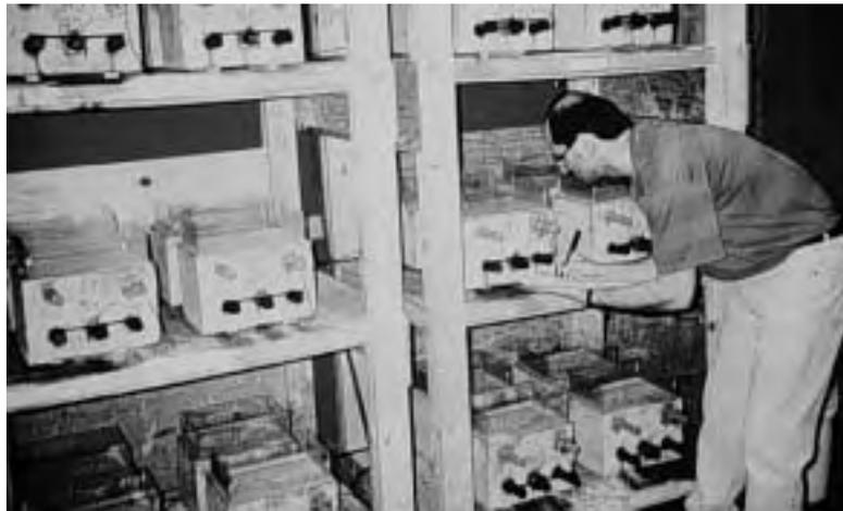
*Figure 1.4 Macrocell test setup.*
