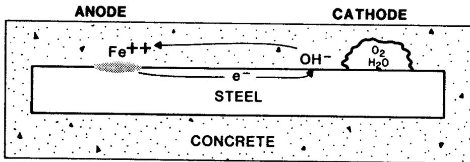
Figure 3.30 Steel depassivation at void formation in concrete.<sup>50</sup>
