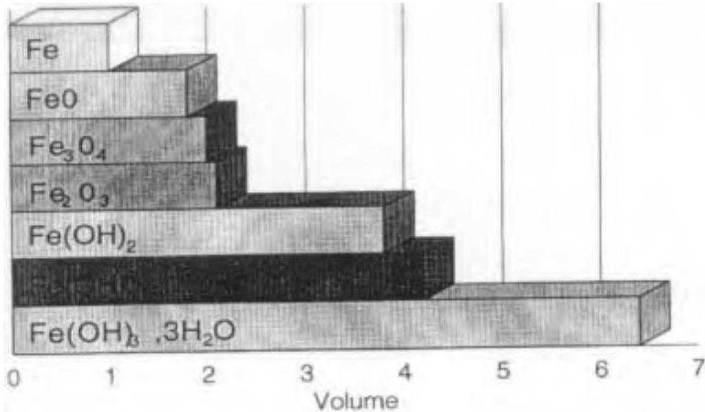
*Figure 3.22 Volume ratio of corrosion products.<sup>47</sup>*
