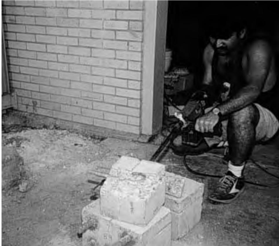
*Figure A.27 Demolishing macrocell specimens.*
