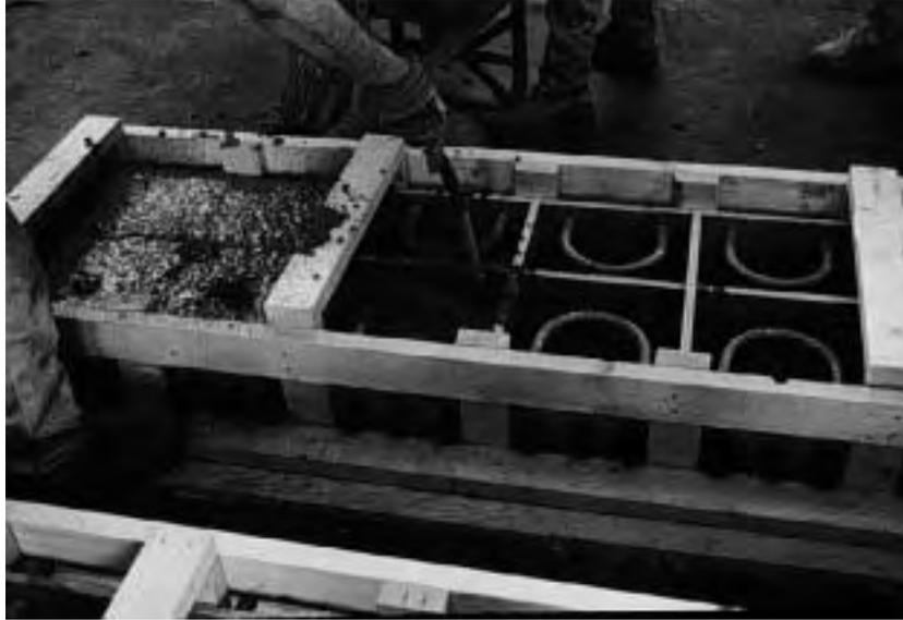
*Figure A.15 Casting macrocell specimens.*
