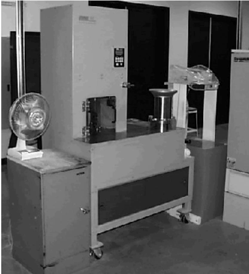
*Figure 3.2. Pine Superpave gyratory compactor model AFGC 125X*
