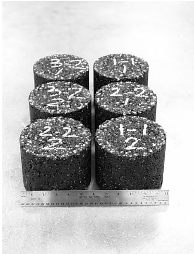
Figure 3.5. Superpave gyratory compactor specimens
