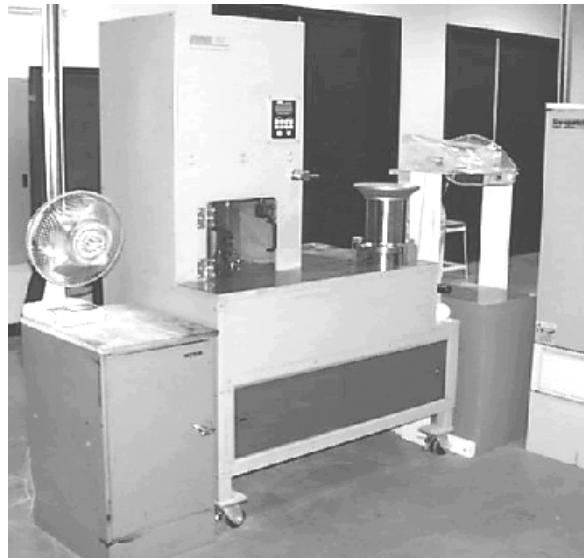
Figure 2.1. Pine Superpave Gyratory Compactor, Model AFGC125X
