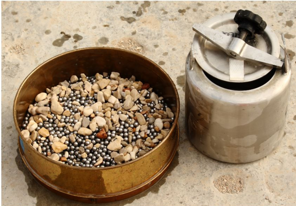
Figure 2: Sample Ready to be washed after Micro-Deval Test
