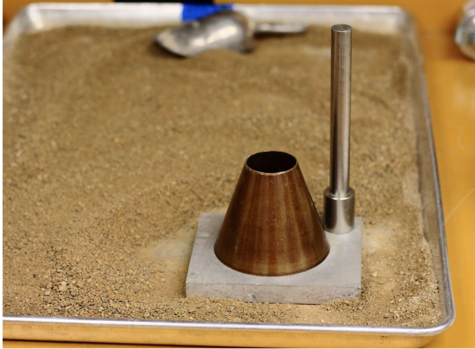
Figure 7: Testing a Sand for Specific Gravity and Absorption
