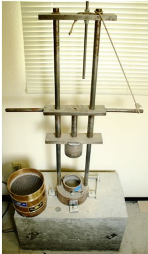
Figure 4: Aggregate Impact Value Test Setup
