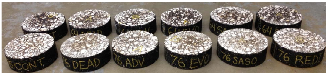
Figure 3.12: Test specimens using the PG64 (top row) and PG76 binders (bottom row); specimens with the PG64 binder suggest higher binder absorption
