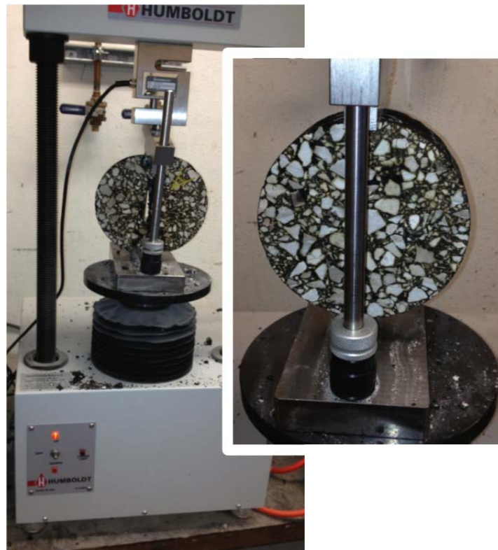
Figure 3.13: Setup to measure the indirect tensile strength of the WMA and HMA mixtures
