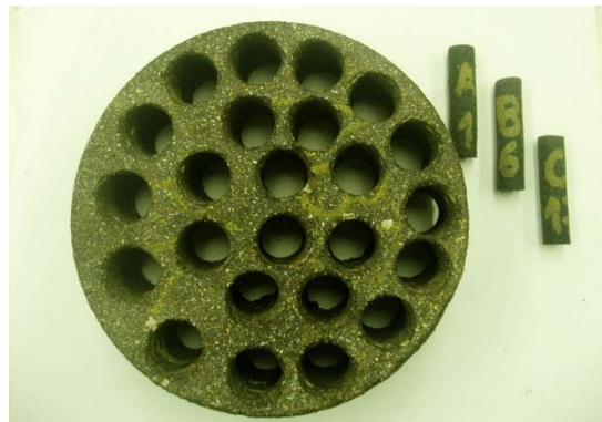
Figure 2.2: Typical FAM test specimens cored out of a Superpave gyratory compacted specimen
