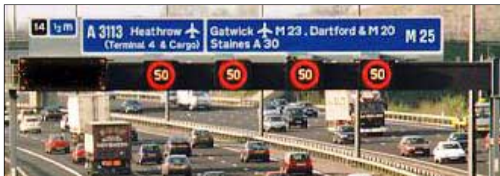
Figure 2.1: Speed harmonization on M25, UK (Warren, 2000)
