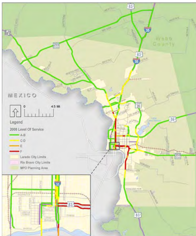
Figure G18: 2008 Laredo Level of Service
