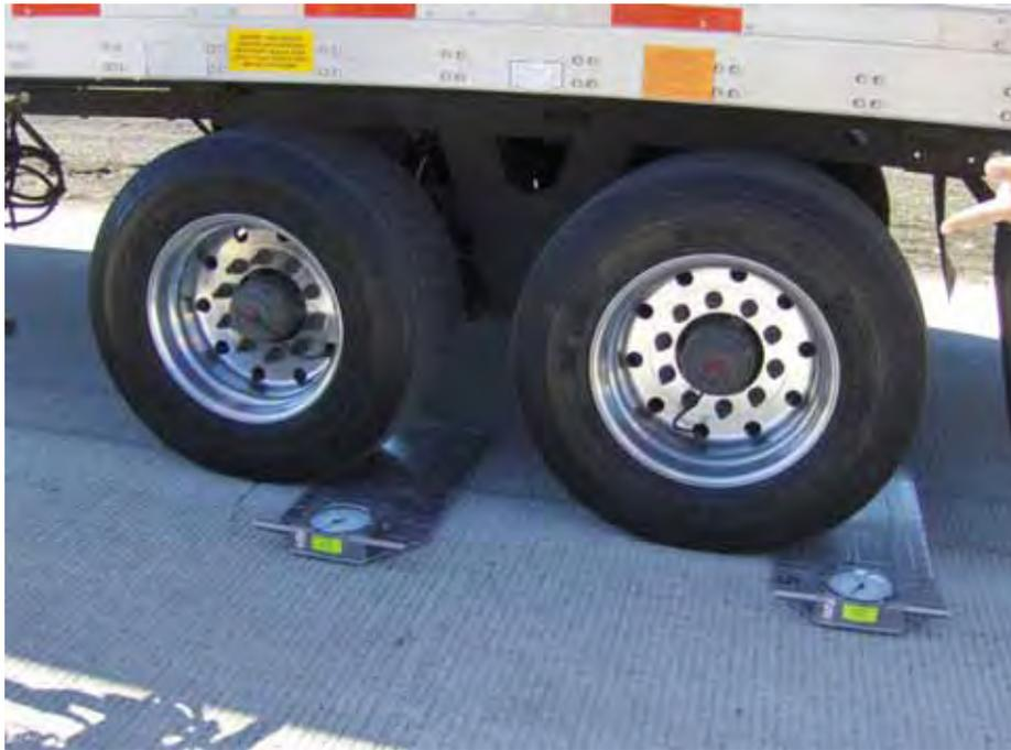
*Figure 5.12: Truck leaving scales after weighing two axles*
