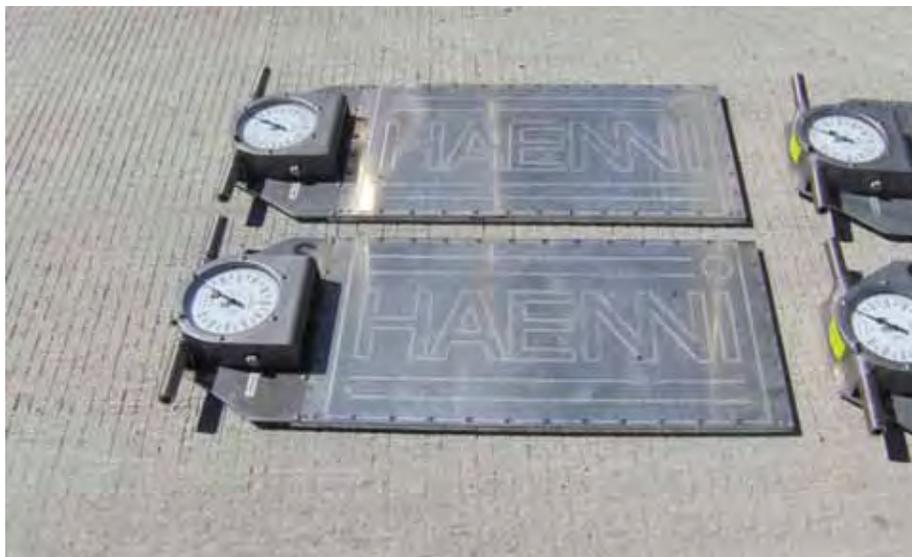
*Figure 5.10: TxDOT's portable scales*
