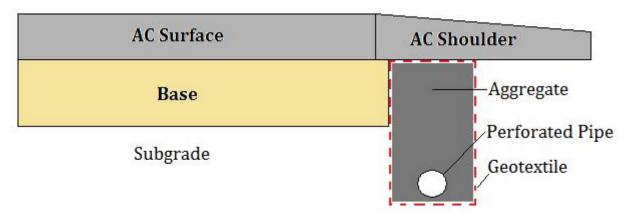
Figure 4.1: Typical trench drain
