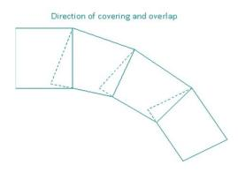
Figure A11. Appropriate direction of overlap when placing geotextile in curve
