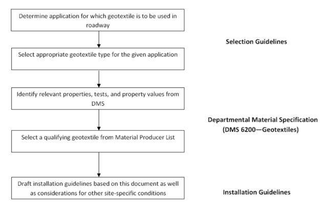
Figure 7.1: Design process flow chart
