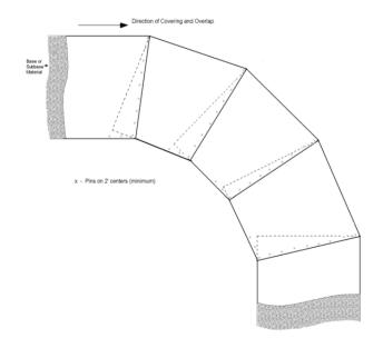
*Figure 2.7: Folded overlaps illustration in curve place (South Carolina Supplemental Specifications)*
