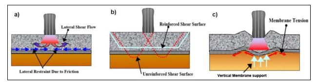
*Figure 2.4: Reinforcement mechanisms induced by a geotextile used for base reinforcement: (a) lateral restraint; (b) increased bearing capacity; (c) membrane-type support.*
