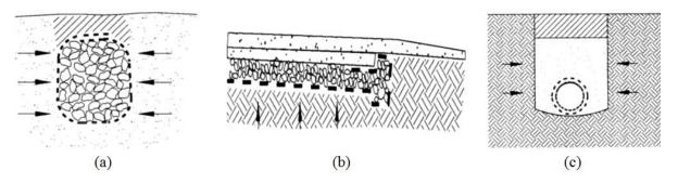
Figure 2.5: Subsurface drainage applications in a roadway structure cited in Holtz et al. 1998—(a) filters around trench and edge drains; (b) filters beneath pavement permeable bases, blanket drains and base courses; (c) geotextile wraps for slotted or jointed drain and well pipes (Holtz et al. 1998)
