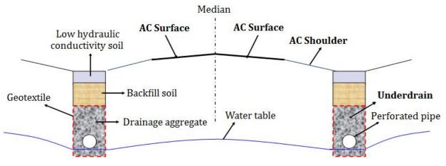
Figure C2. Typical underdrain
