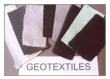
Figure A1: View of different types of geotextiles
