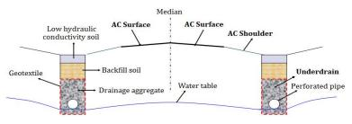
Figure A6. Typical underdrain
