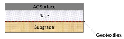
Figure A10. Location of geotextile in Pavement Structural Section applications
