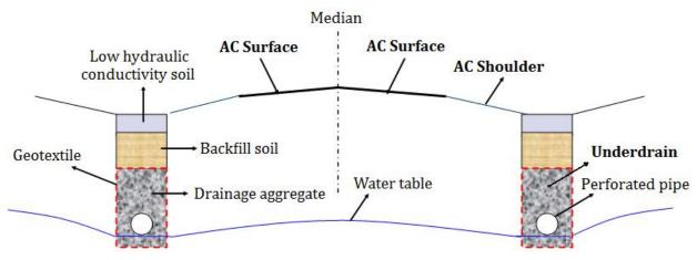
Figure 4.2: Typical underdrain
