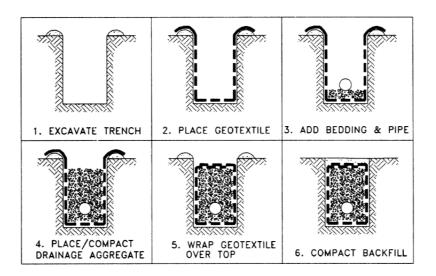
Figure 2.9: Construction procedures illustrations (Holtz et al. 1998)
