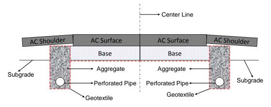
Figure 2.11: Geotextile used for base or subbase barrier for lateral flow in roadway (modified from AASHTO 2006)
