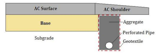
Figure C1: Typical trench drain
