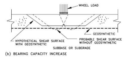
Figure 4.4: Increased load carrying capacity via bearing capacity increase with subgrade restraint (Holtz et al. 1998)
