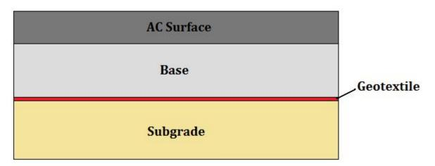
*Figure 4.3: Typical section with geotextile used as separator between base and subgrade Note: The same layout corresponds to a geotextile used as a stabilizer.*
