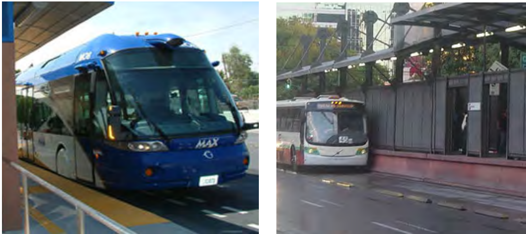
Figure 2.1: Low Floor BRT on Las Vegas “MAX” (Left) and High Floor on BRT Mexico City “Metrobus” (Right)
