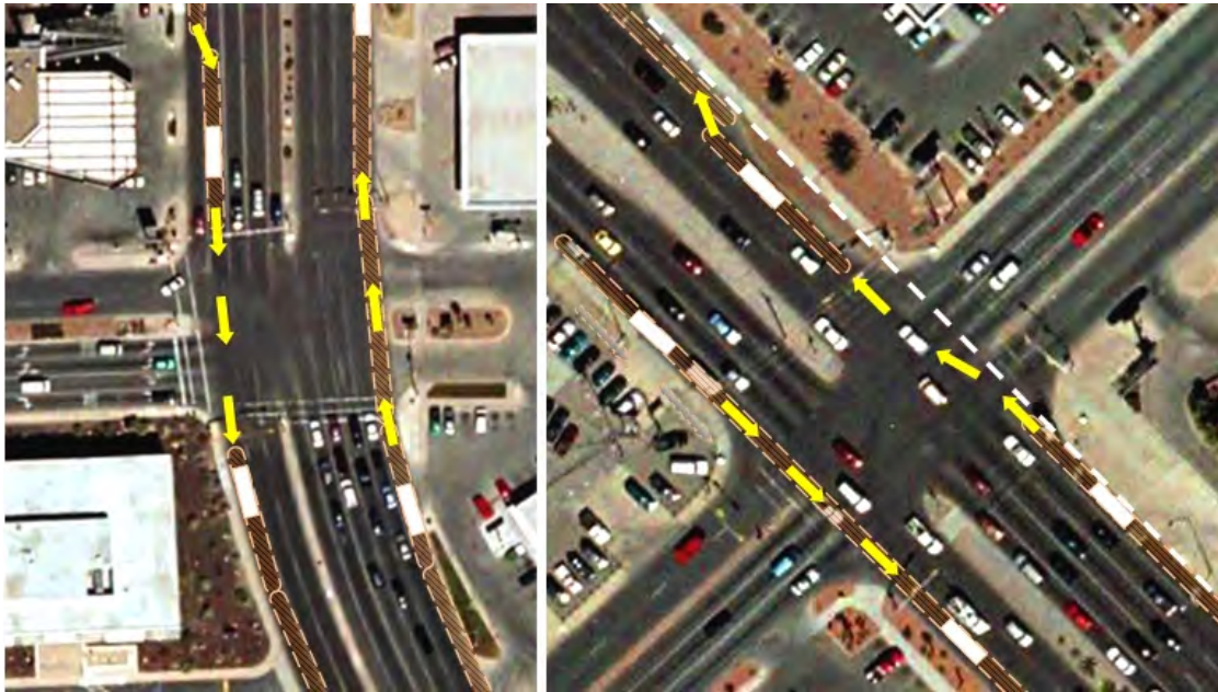
Figure 9.14: Queue jumper at the intersection of Mesa and Executive (left) and Mesa and Resler (right)
