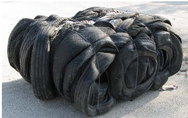
Figure 2.1: Photograph of a Traditional Scrap Tire Bale
