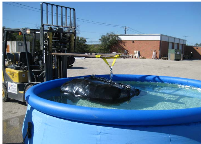
Figure 5.5: Submergence of a Wrapped Tire Bale
