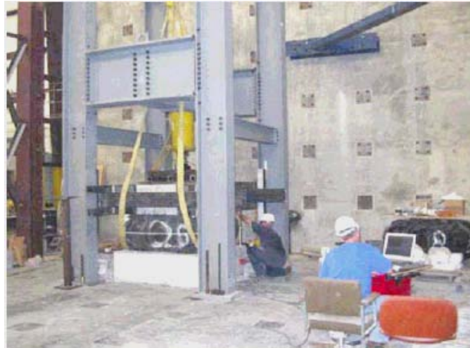
Figure 2.6: Large Compression Test Setup (Zornberg et al. 2005)
