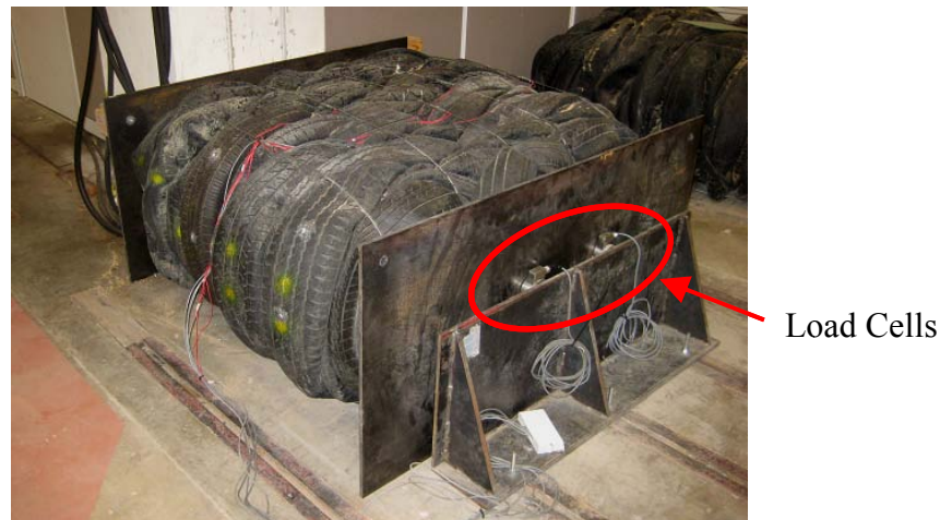
Figure 5.13: Photograph of the Horizontal Pressure Testing Setup
