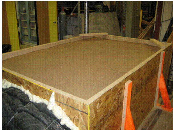
Figure 6.25: Photograph of the Thick Sand Interface
