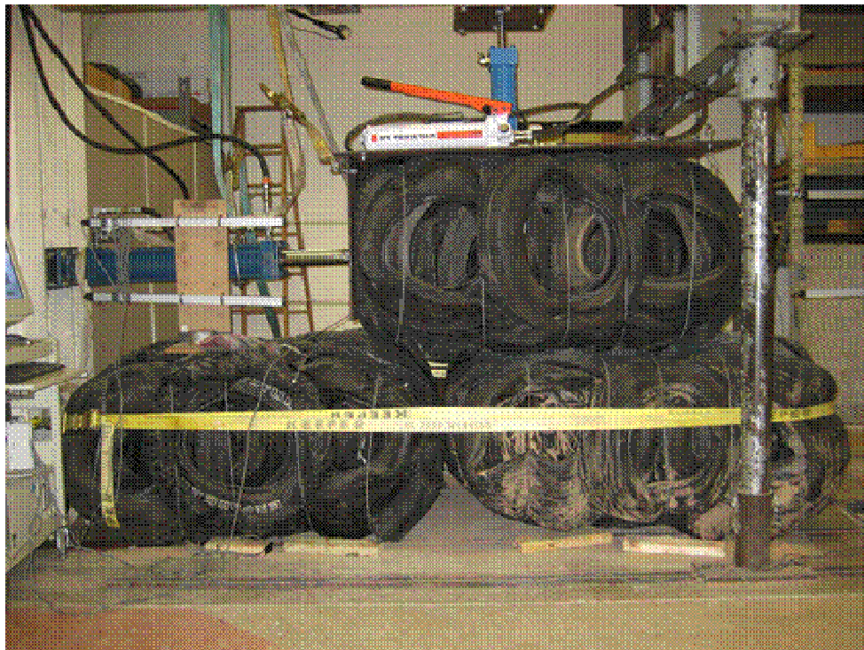
Figure 6.19: Anisotropic Tire Bale Direct Shear Testing Setup
