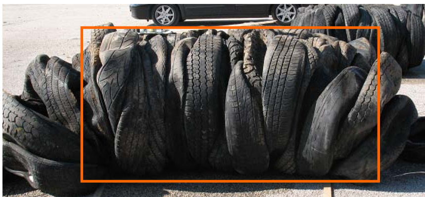
Figure 5.11: Photographs of Tire Bale 2 after Each Wire Breakage (Rapid Expansion Test)
