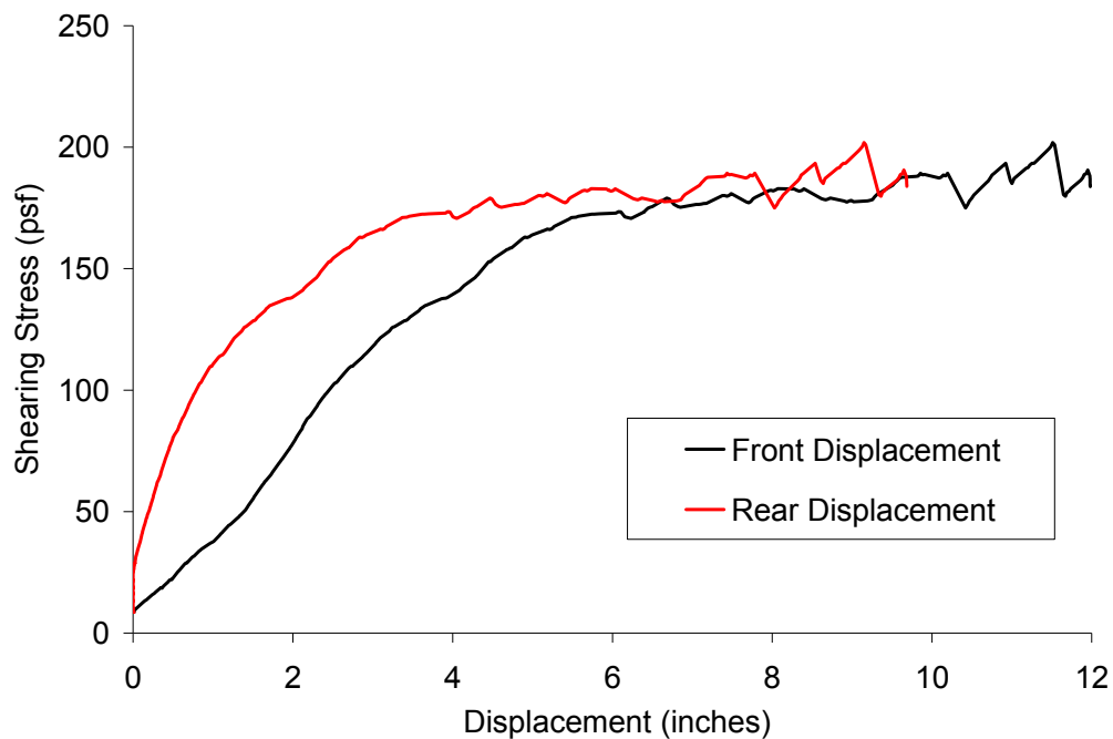
Figure 6.8: Interface Shearing Stress versus Tire Bale Displacement for the Dry Tire Bale Interface
