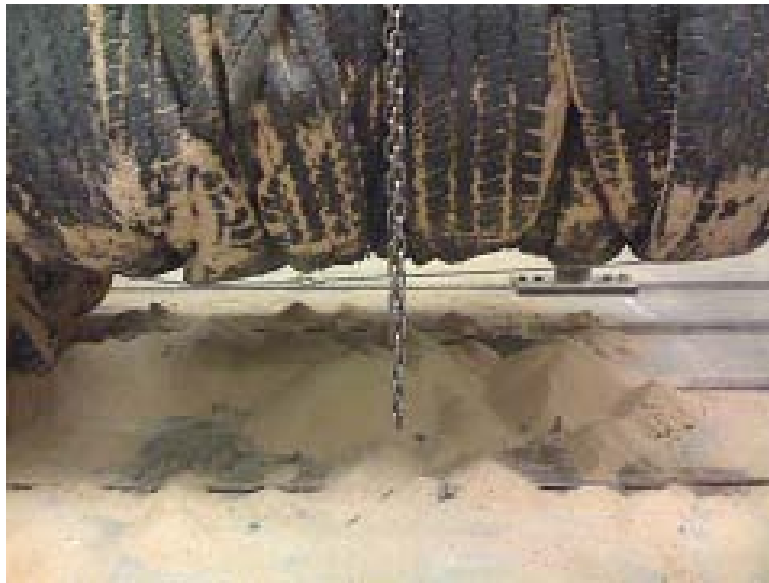
Figure 6.34: Total Sand Outflow from the Tire Bale
