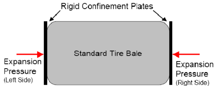
Figure 5.12: Illustration of the Horizontal Pressure Testing Setup
