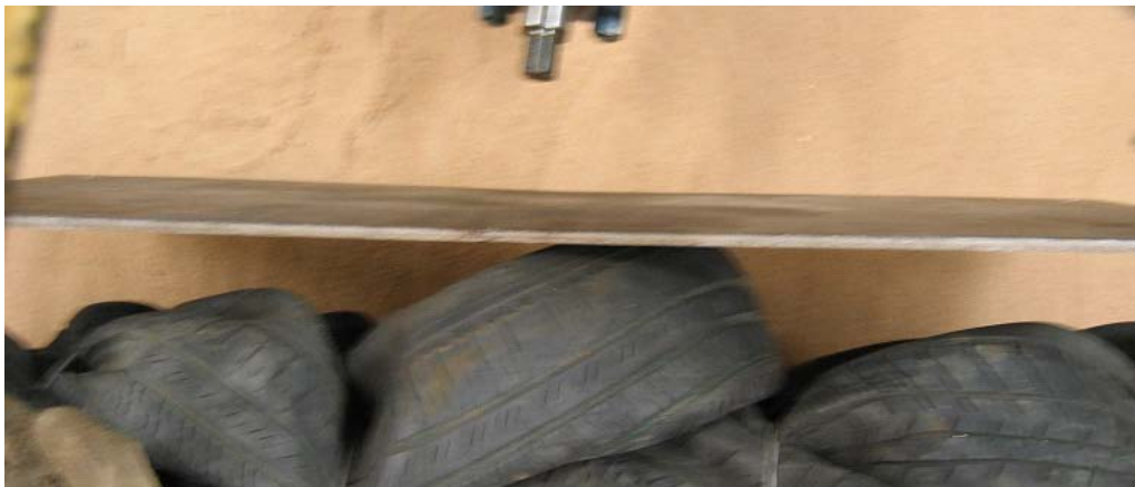
Figure 6.14: Irregular Loaded Bale Interface (Application of Shearing Load)
