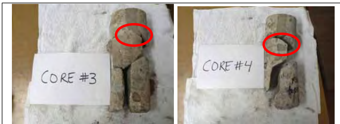
Figure 3.24: Absence of Backer Rod in Longitudinal Joint Cores
