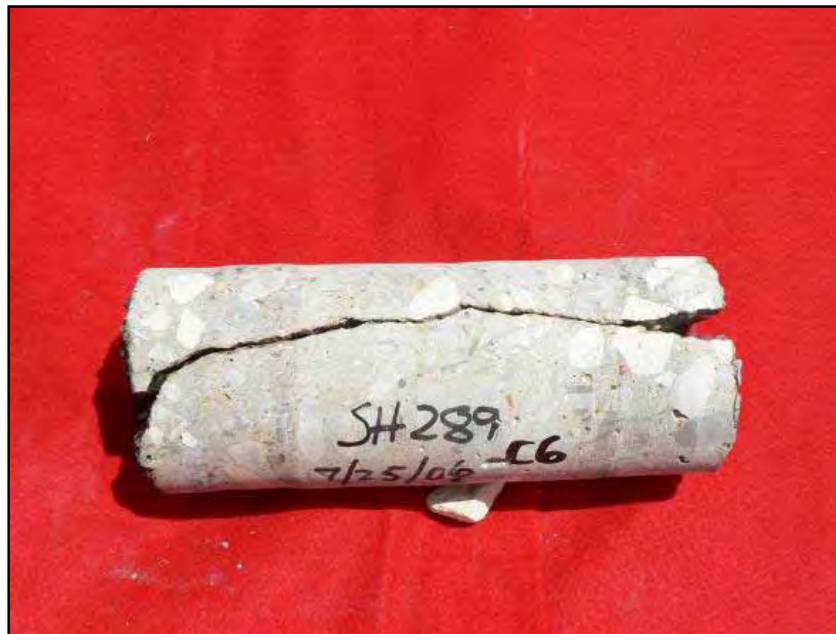
Figure 3.48: Core through Longitudinal Crack (2)
