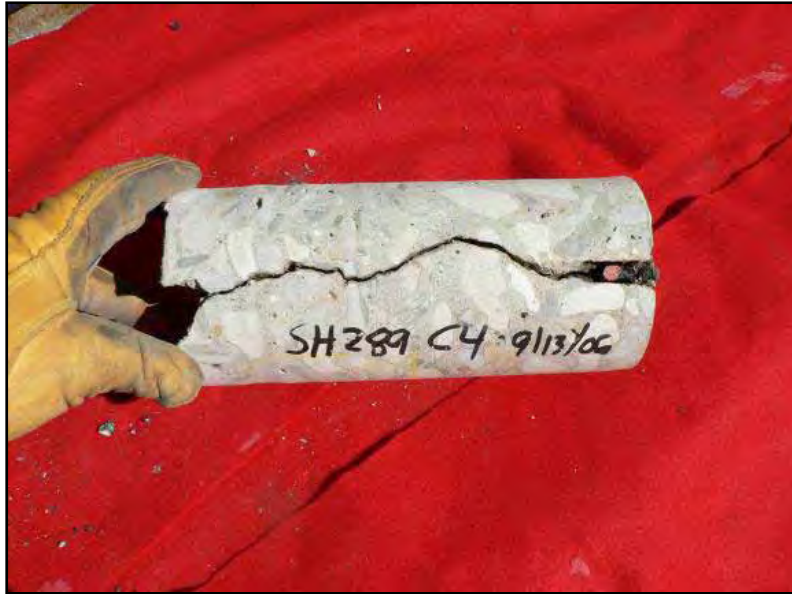
Figure 3.55: Core Through Contraction Joint (2)
