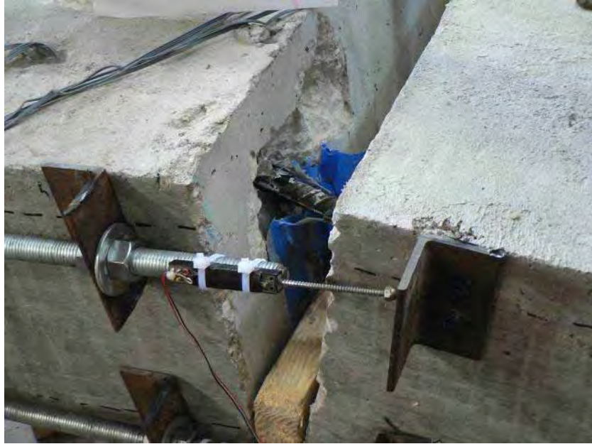
Figure 4.45: Left Cross Stitch Bar at End of Test
