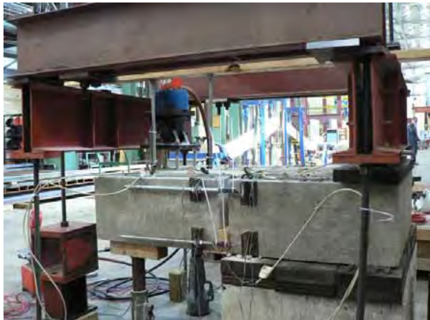
Figure 4.52: Slot Stitch Specimen Before Flexure Test
