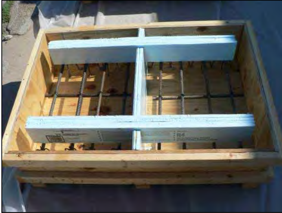
Figure 4.13: Slot Stitch Shear Specimen Before Casting
