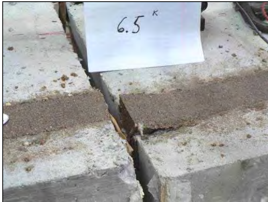
Figure 4.37: Repair Material Failure (Right Side)
