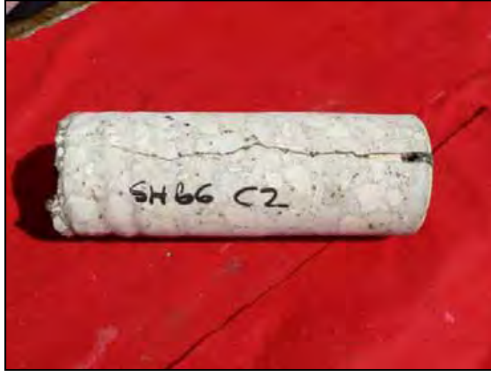
Figure 3.39: Core Through Contraction Joint Adjacent to Uncracked Slabs (2)
