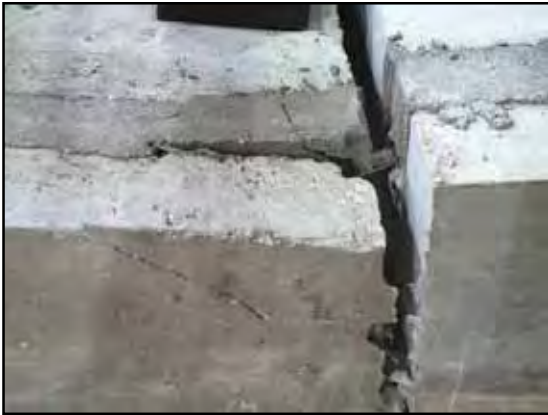
Figure 4.42: Left Side of Slot Stitch Specimen at End of Test
