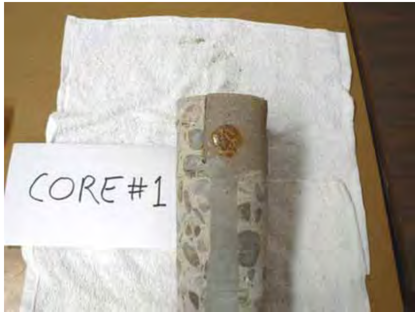
Figure 3.19: Staple Corrosion (Core #1)
