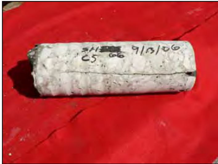
Figure 3.38: Core Through Contraction Joint Adjacent to Uncracked Slabs (1)
