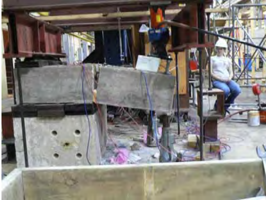
Figure 4.48: Staple Specimen at End of Flexure Test (1)
