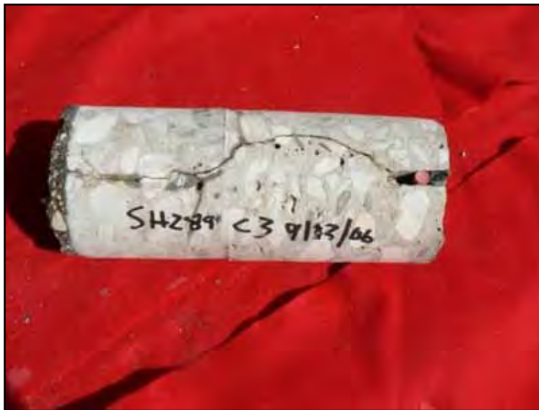
Figure 3.54: Core Through Contraction Joint (1)
