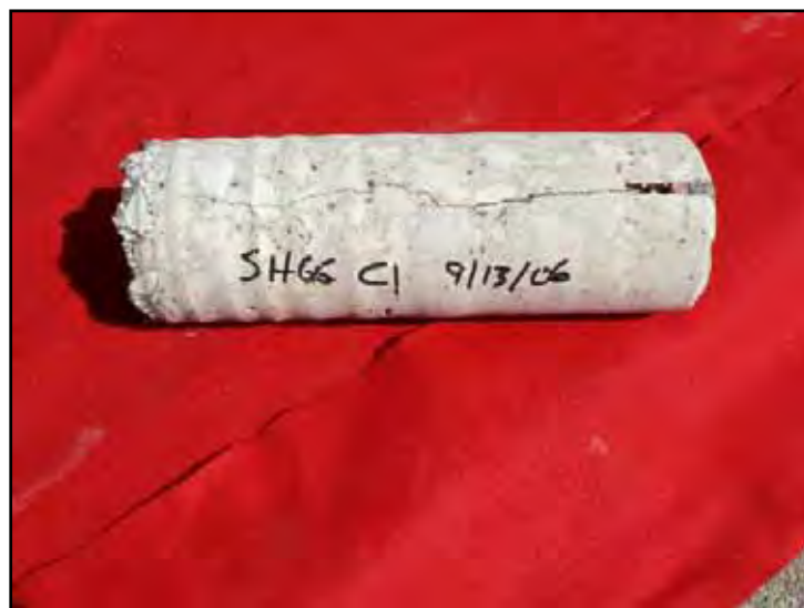
Figure 3.36: Core Through Contraction Joint Adjacent to Cracked Slabs (1)
