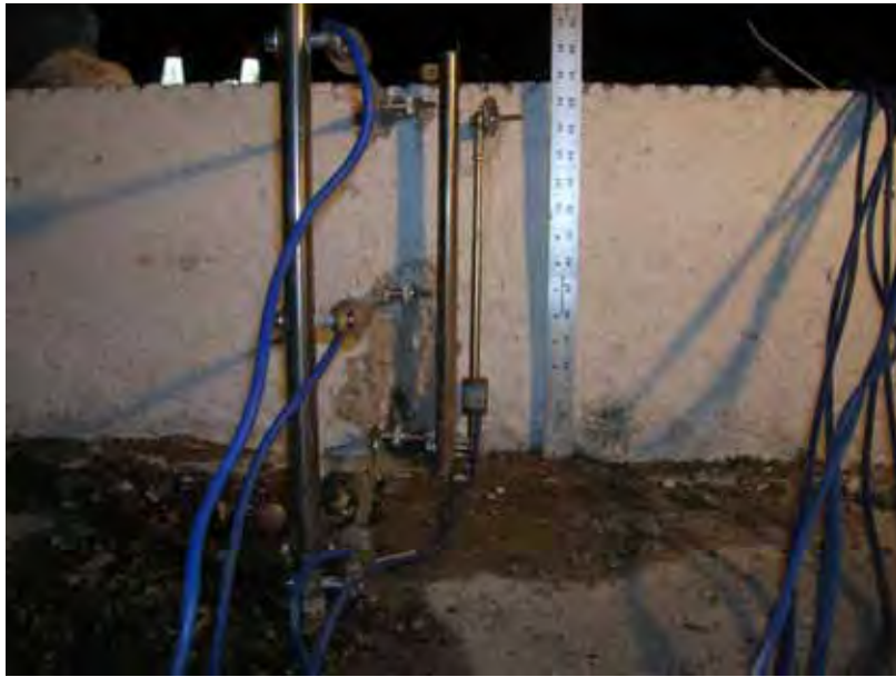
(a) Vertically installed crackmeter
