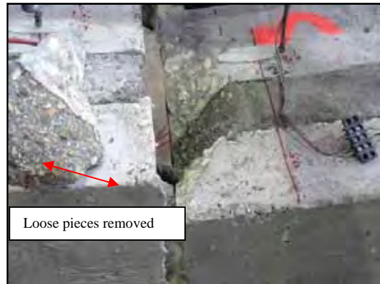
Figure 4.43: Right Side of Slot Stitch Specimen at End of Test
