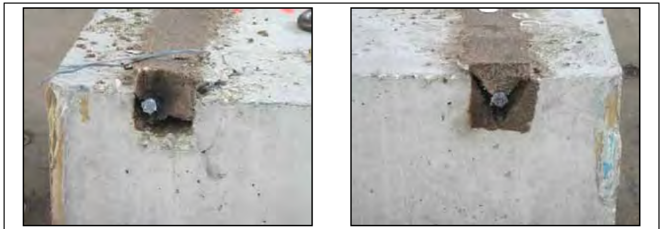
Figure 4.39: Left (L) and Right (R) Staple Bars After Testing
