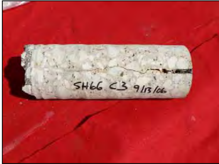
Figure 3.37: Core Through Contraction Joint Adjacent to Cracked Slabs (2)
