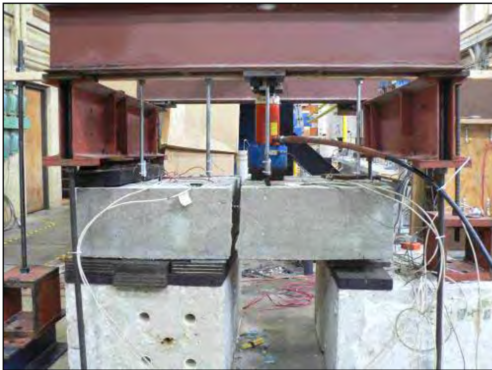
Figure 4.26: Shear Loading Test Frame (Side View)
