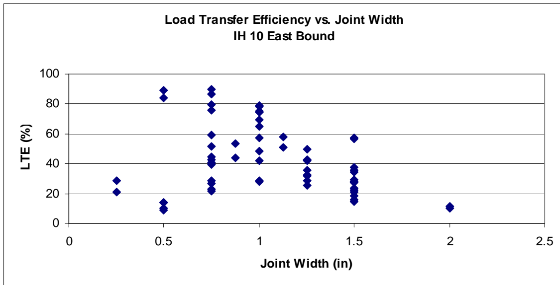
Figure 3.91: LTE vs. Joint Width (Eastbound)
