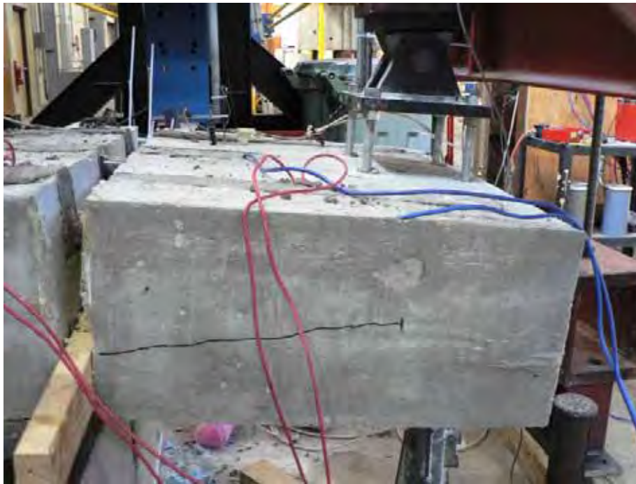
Figure 4.56: Right Side of Slot Stitch Specimen at Failure
