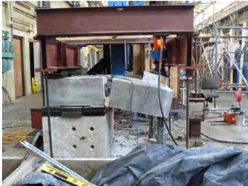
Figure 4.44: Cross Stitch Specimen at End of Test
