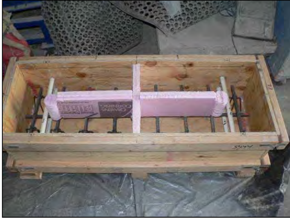
Figure 4.24: Headed Bar Specimen Before Casting
