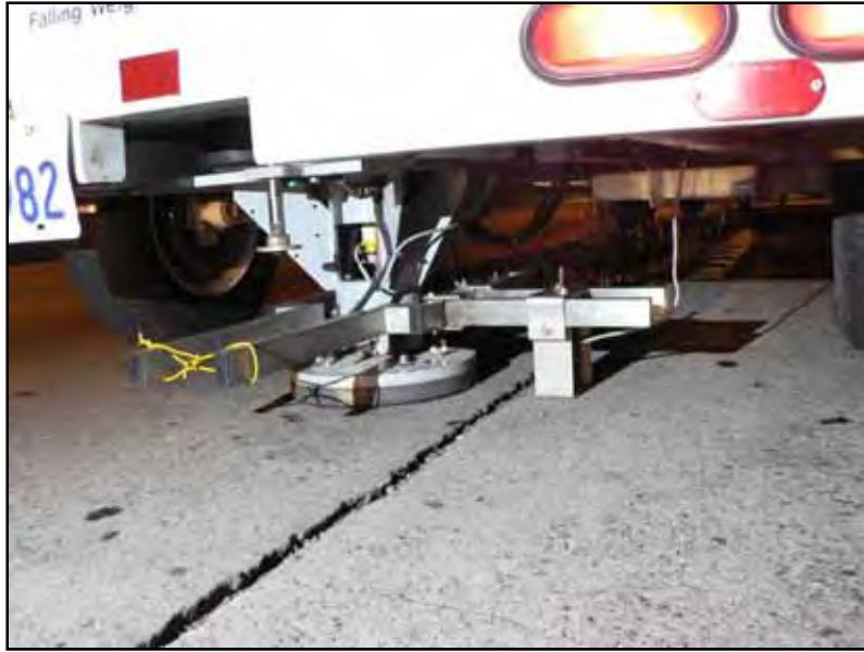
Figure A.4: New FWD Setup in the Field
