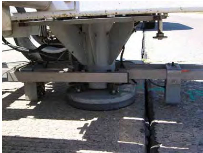
Figure A.1: Conventional FWD setup in the Field
