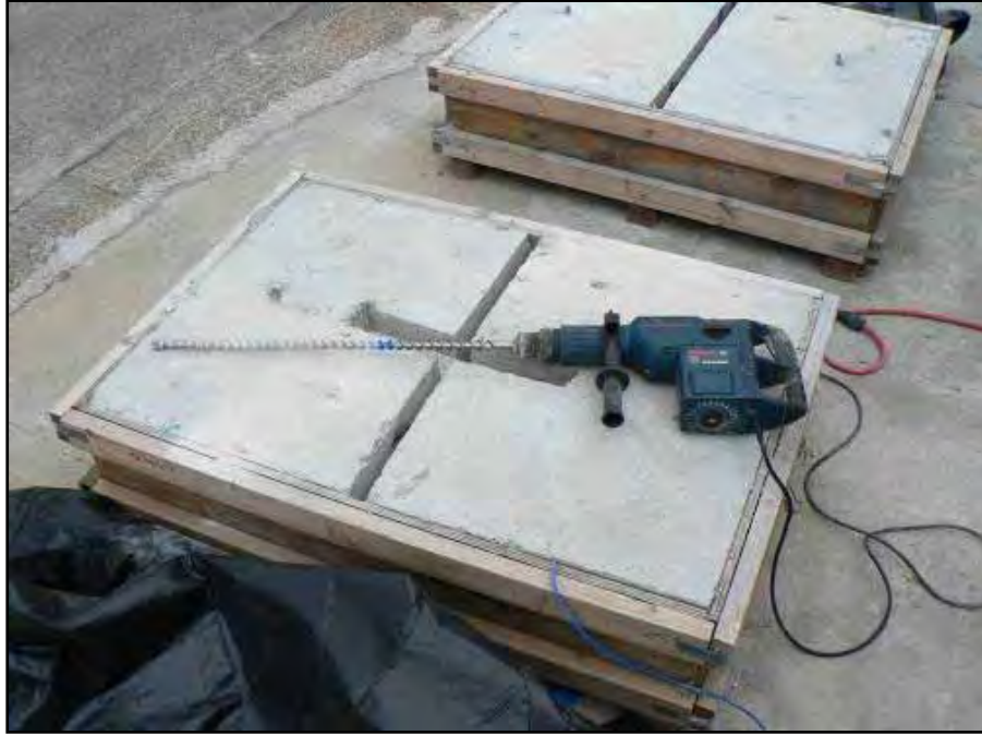
Figure 4.9: Cross Stitch Shear (Top) and Flexure (Bottom) Specimens
