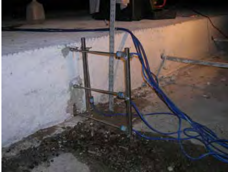
(a) Crackmeters for transverse movement
