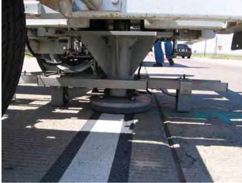
Figure 3.3: FWD Load Plate and Sensors
