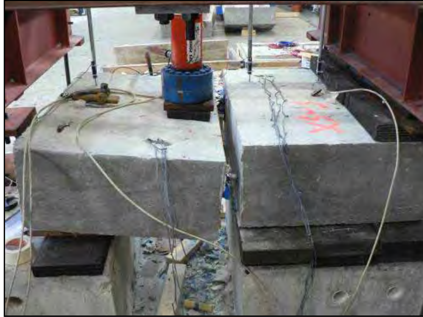
Figure 4.33: Cross Stitch Specimen at Failure Under Shear Load
