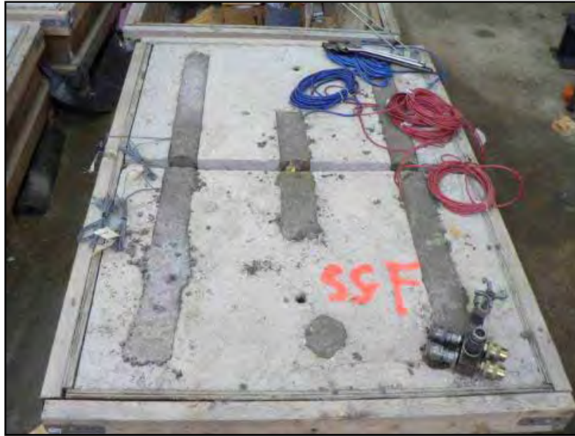
Figure 4.15: Slot Stitch Flexure Specimen After Casting
