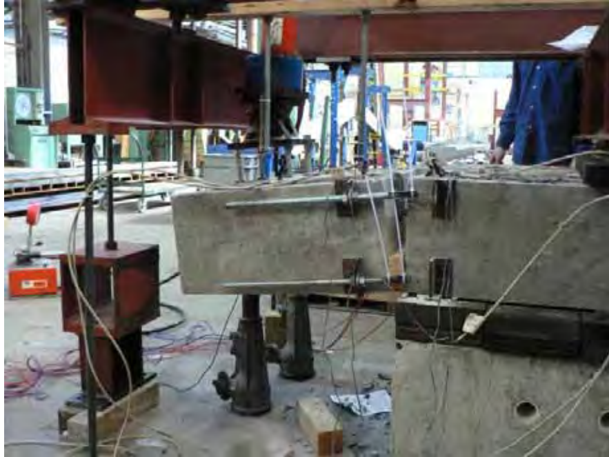
Figure 4.53: Slot Stitch Specimen at Failure
