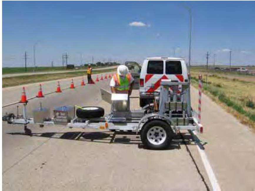
Figure 3.1: FWD Testing on Longitudinal Joint
