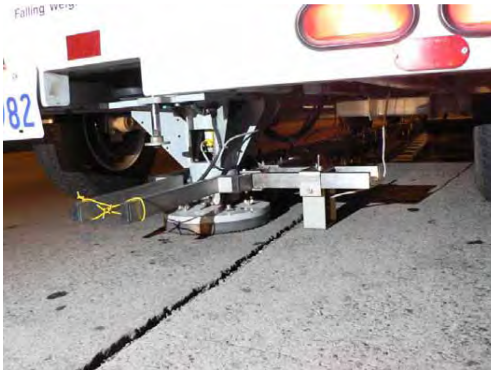
Figure 3.84: Modified FWD Setup
