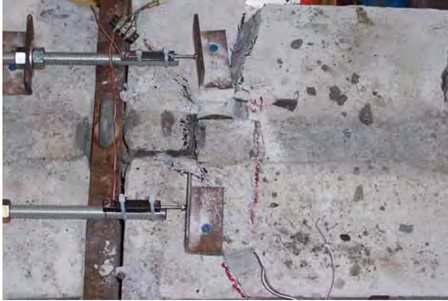
Figure 4.61: Headed bar Specimen at Failure
