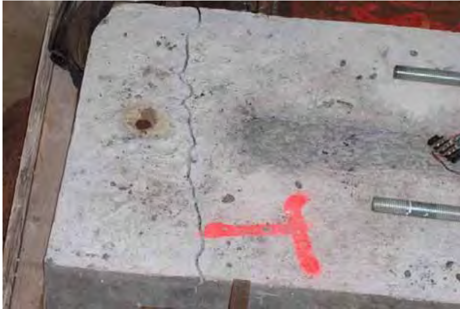
Figure 4.59: Cracking of Specimen at Loading Brackets
