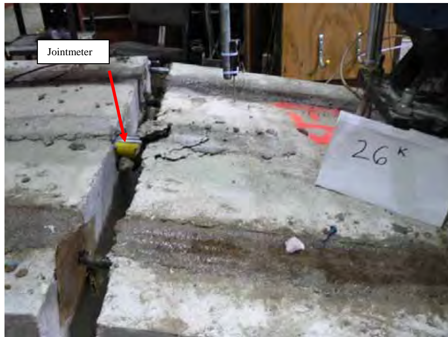
Figure 4.49: Staple Specimen at End of Flexure Test (2)
