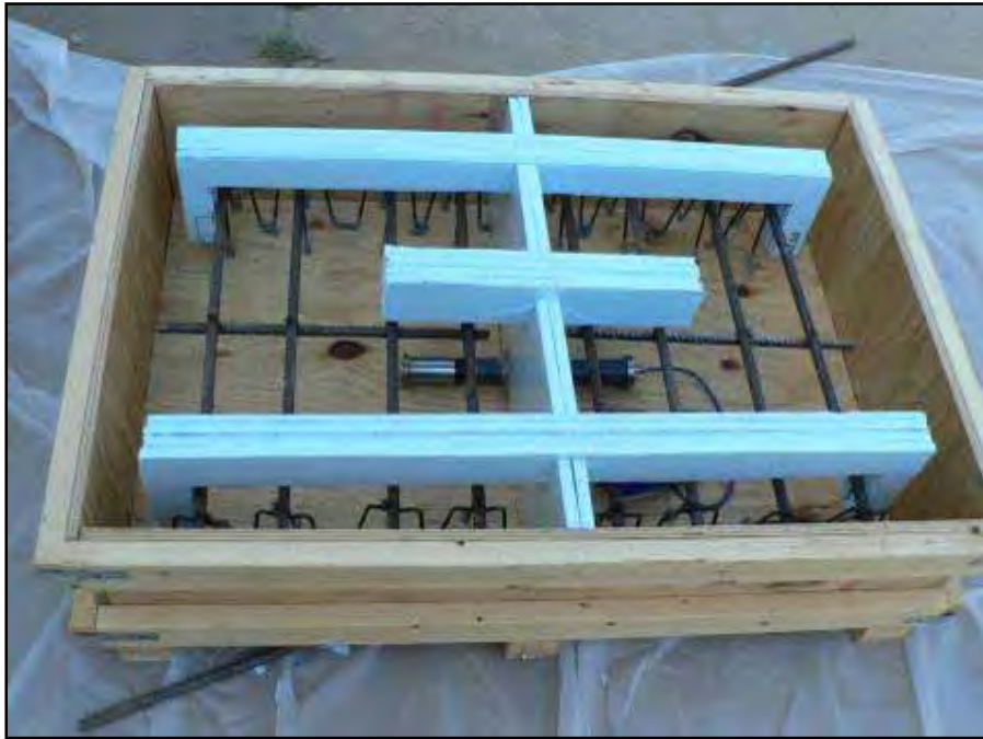
Figure 4.19: Staple Flexure Specimen Before Casting
