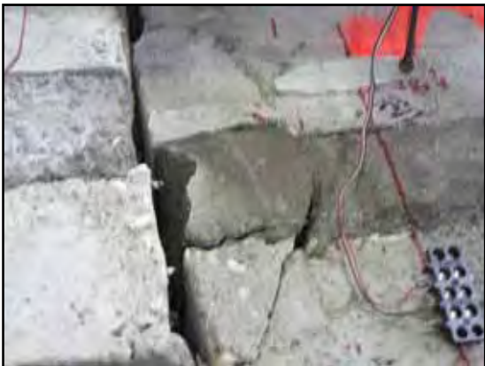
Figure 4.43: Right Side of Slot Stitch Specimen at End of Test
