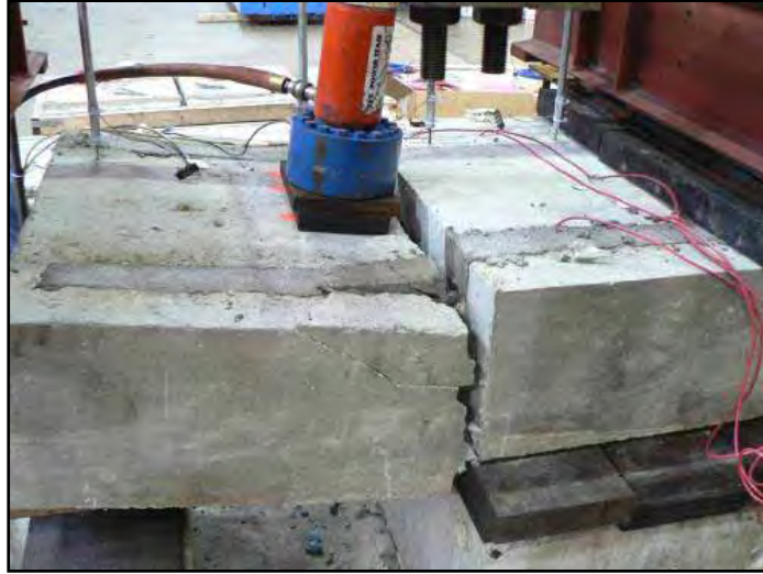
Figure 4.41: Slot Stitch Specimen at End of Shear Test
