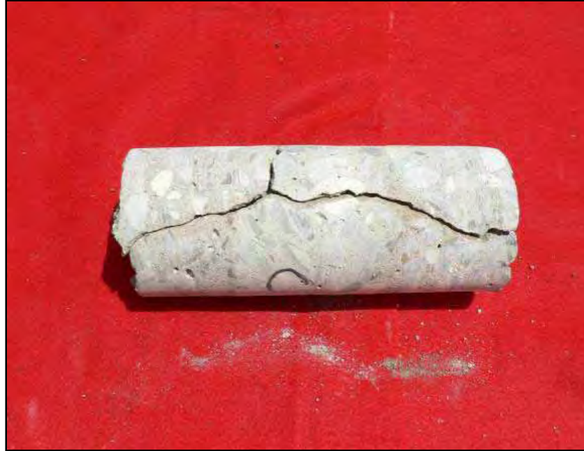
Figure 3.47: Core through Longitudinal Crack (1)
