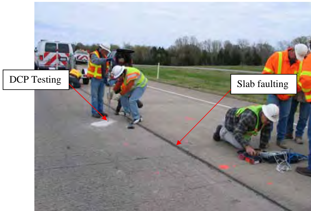
Figure 4.86: Sherman Slab 3 DCP Test Location
