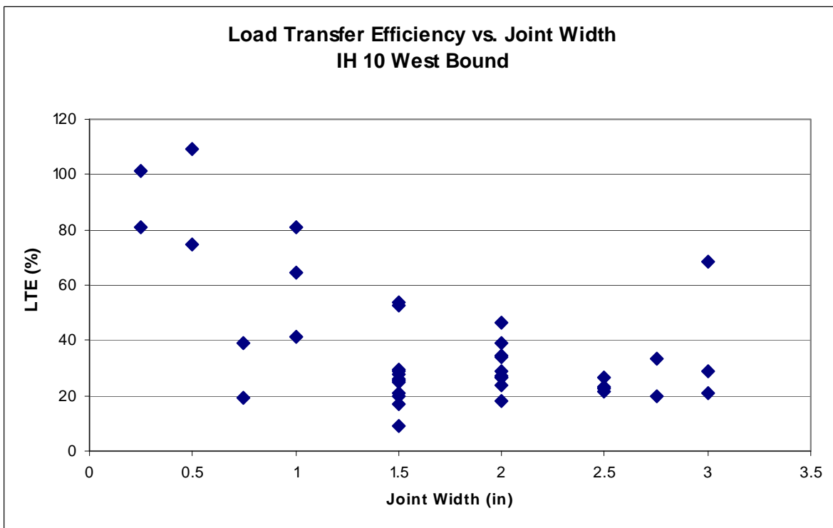
Figure 3.92: LTE vs. Joint Width (Westbound)
