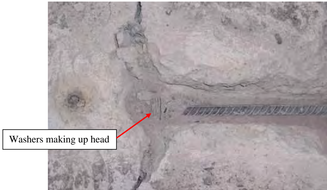
Figure 4.63: Exposed Head after Testing
