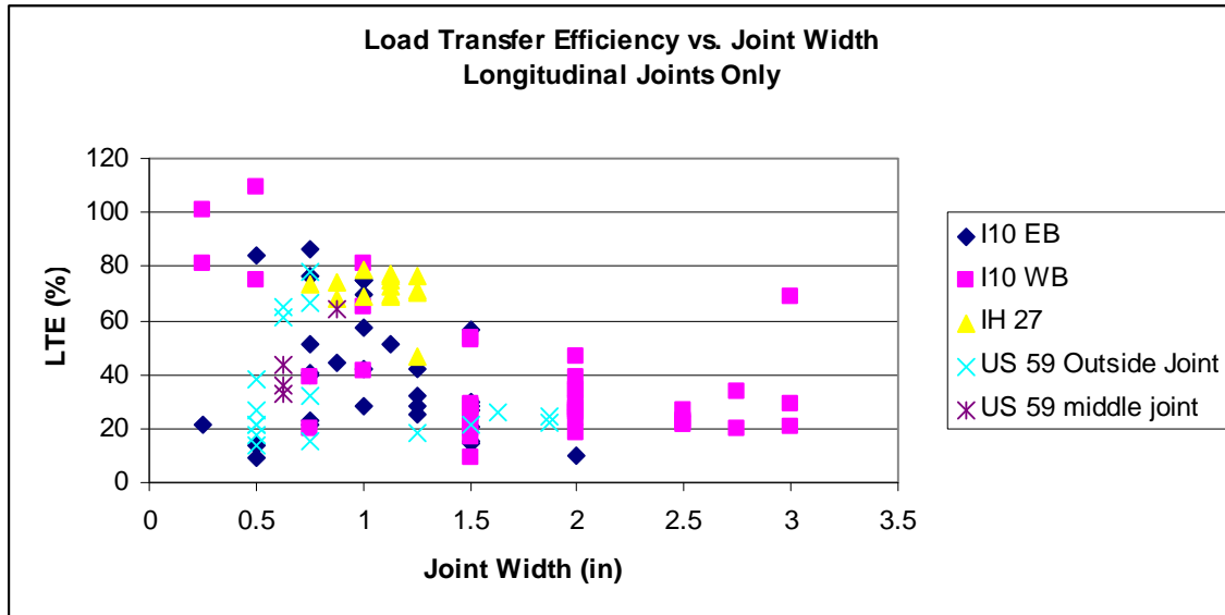
Figure 3.97: LTE vs. Joint Width
