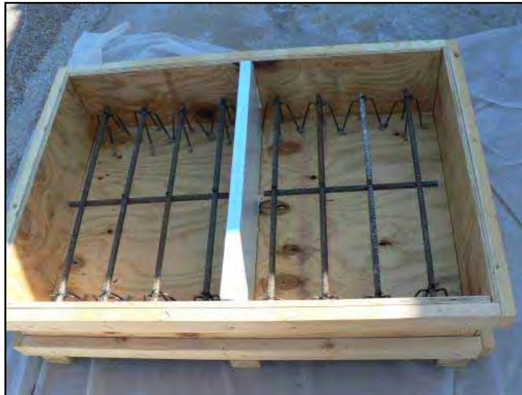
Figure 4.7: Cross Stitch Shear Specimen Before Casting
