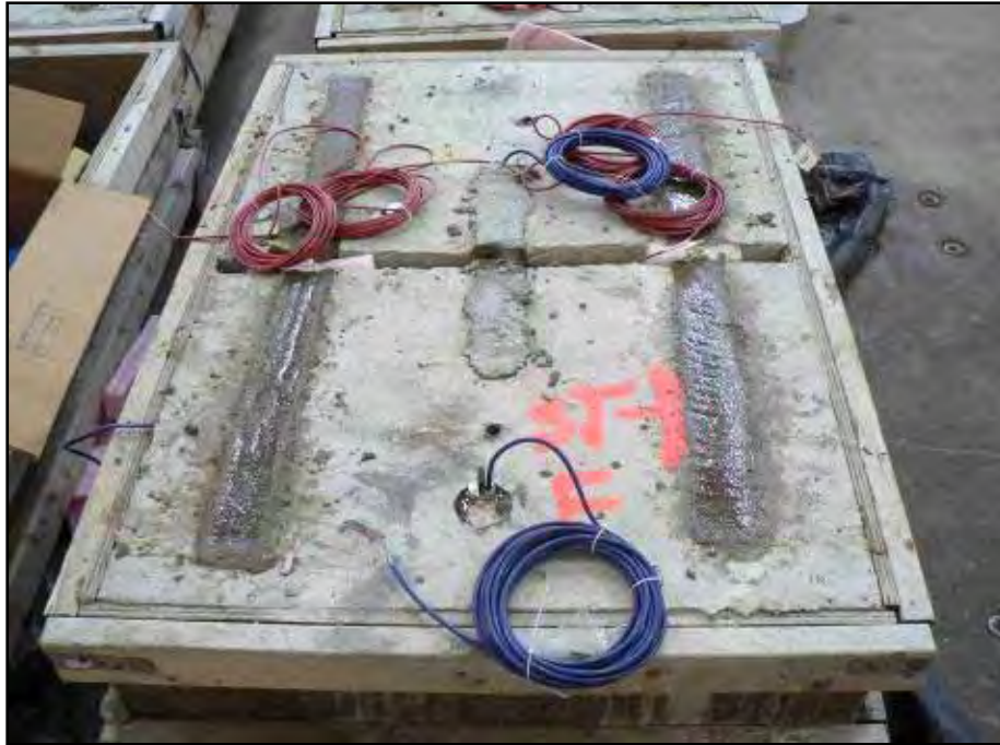
Figure 4.20: Staple Flexure Specimen After Casting
