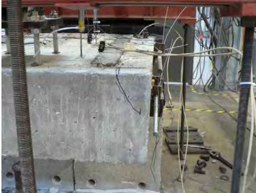
Figure 4.55: Left Side of Slot Stitch Specimen at Failure
