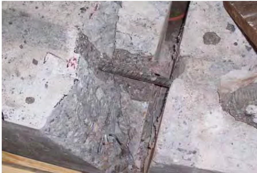
Figure 4.62: Headed Bar Specimen with Broken Concrete Removed
