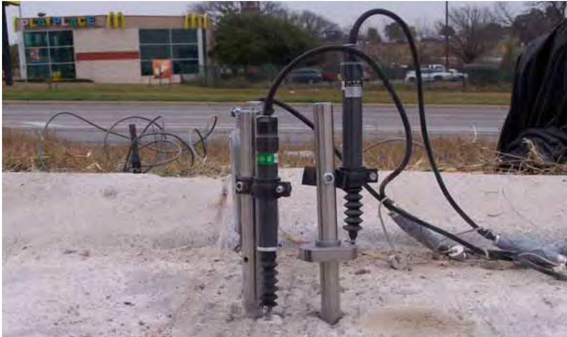
Figure 5.18: Field testing for curling measurement
