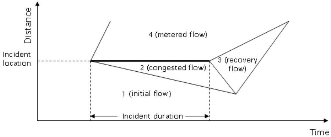
Figure 3.1: Idealized shockwave diagram for a stationary incident.
