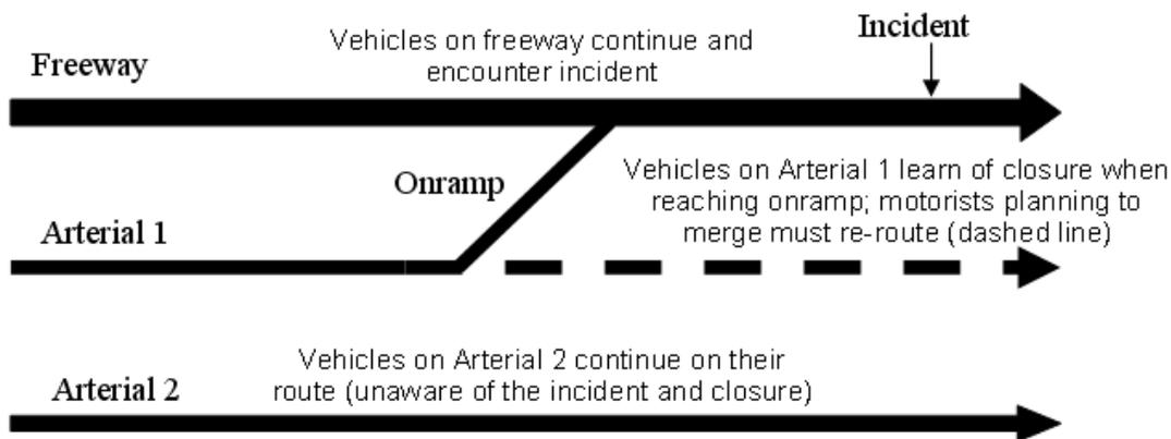
Figure 4.2: Diagram of rerouting behavior under information provision.
