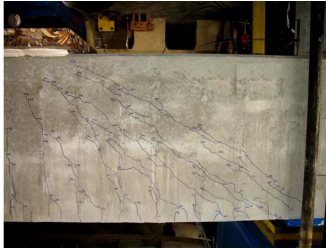
Figure 2.8: Combination of one and two-panel behavior ( a/d = 1.85 ).
