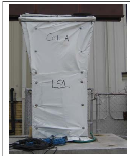
Figure 5.14: Burlene Wrap to hold in moisture.
