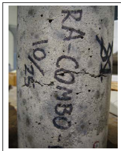
Figure 3.7: Concrete cylinder from heat cured RA1 Mix; surface drying and cracking after curing.
