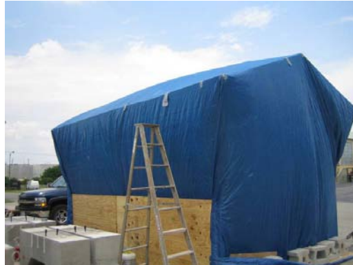
Figure 5.3: Heat curing enclosure for model columns
