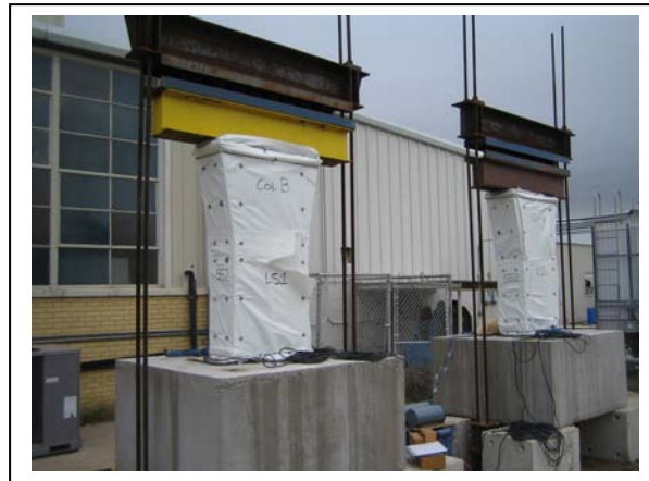
Figure 5.15: Post-tensioning system for simulating service load conditions.
