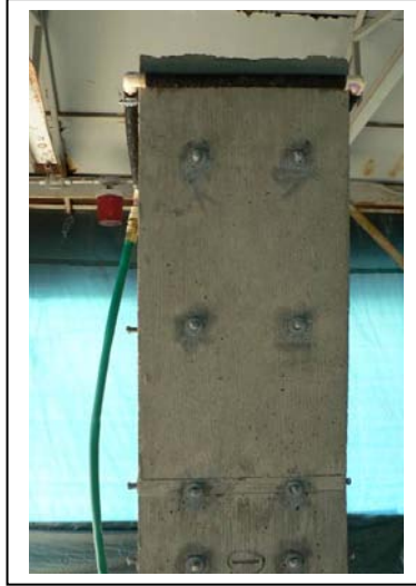
Figure 5.13: Soaker hose watering system.
