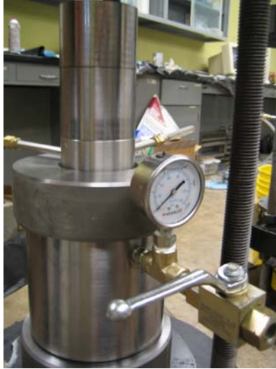
Figure 4.6: Hoek Cell inside Load Frame.
