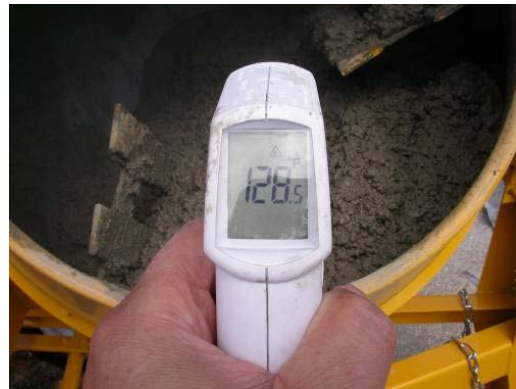
Figure 5.6: Temperature of concrete during mixing
