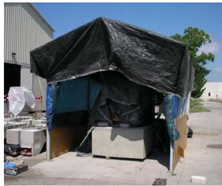
Figure 5.8: Tent enclosure wheeled over top of columns
