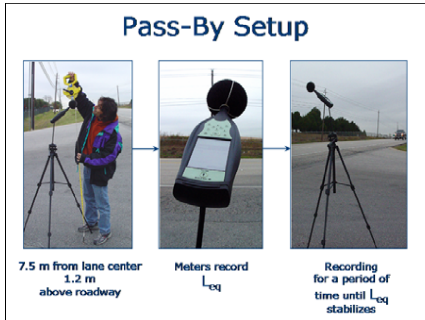
Figure 2.1: Pass-by noise measurements at roadside
