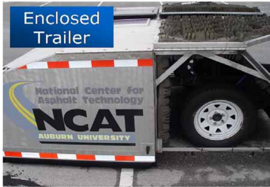
Figure 2.5: Typical enclosed CPX noise measurement trailer
