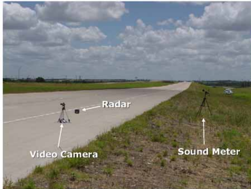
Figure 5.3: Equipment setup for traffic recording for pass-by tests
