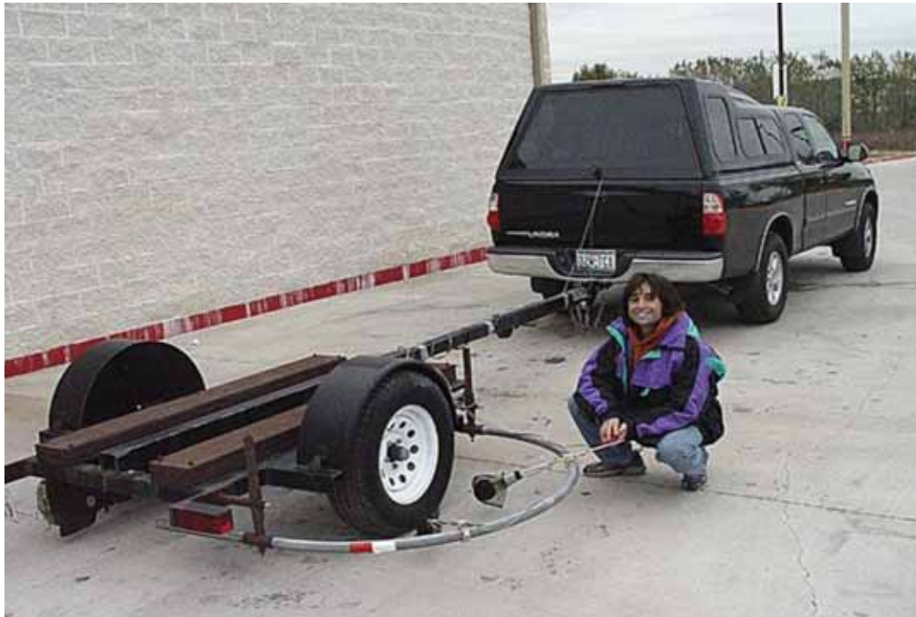
Figure 2.4: Free field CPX trailer system for pavement noise measurement
