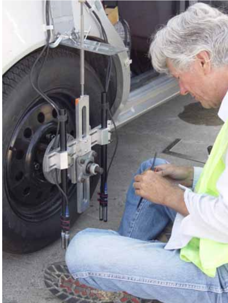
Figure 3.18: Transtec new OBSI rig for the Second Rodeo
