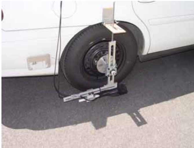
Figure 3.11: CTR and TxDOT OBSI fixture
