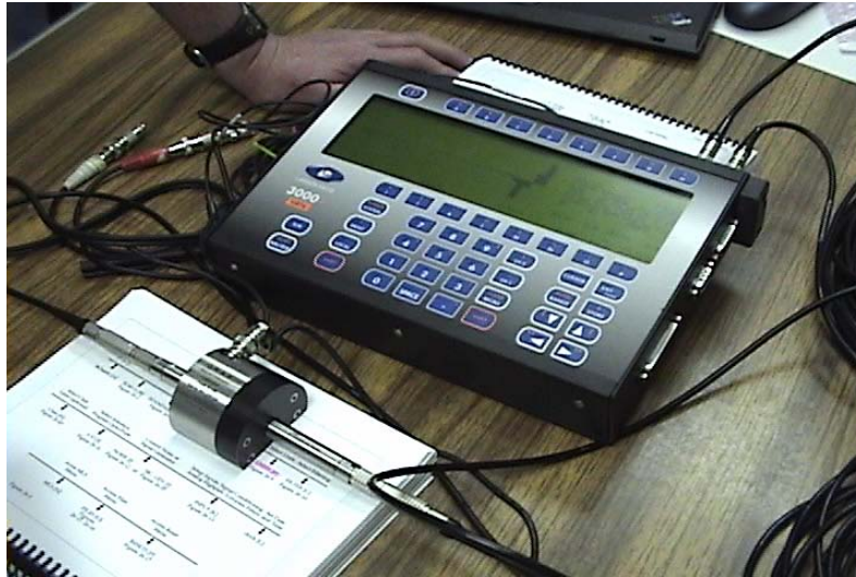
Figure 6.4: Phase comparisons between the two OBSI microphones
