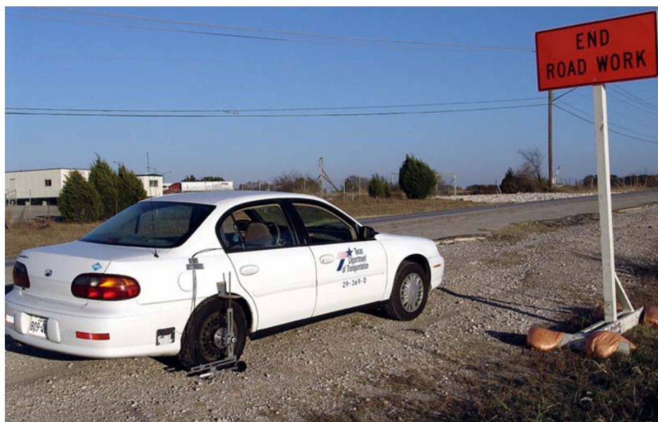
Figure 3.7: TxDOT vehicle with attached OBSI noise probe
