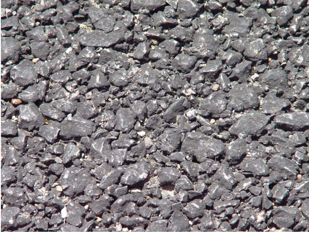
Figure 4.22: Texture of the new PFC overlay on IH-30 in Dallas
