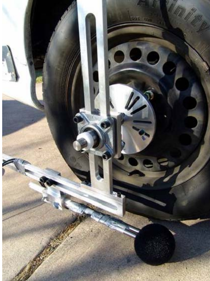
Figure 3.8: Close up view of assembled SI test probe on vehicle
