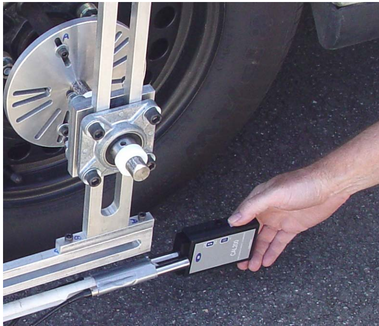
Figure 6.1: Field Calibration of OBSI microphones
