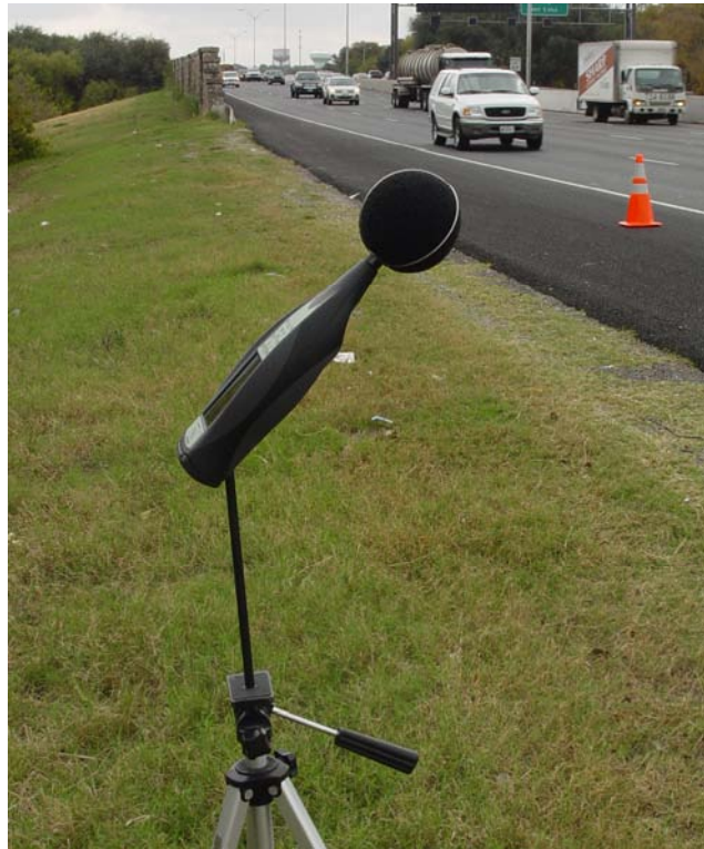
Figure 5.2: SPL meter on a tripod during pass-by test
