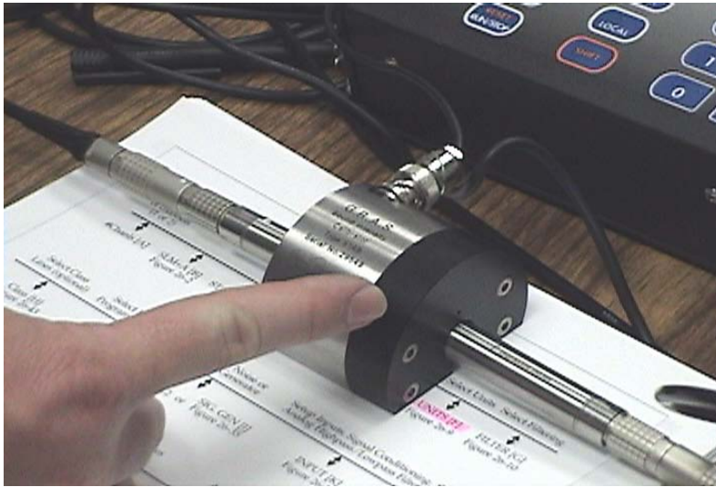
Figure 6.2: Checking phase and levels between SI microphones
