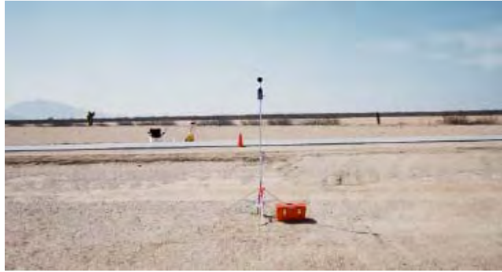
Figure 2.9. Field measurement set-up for wayside noise recording
