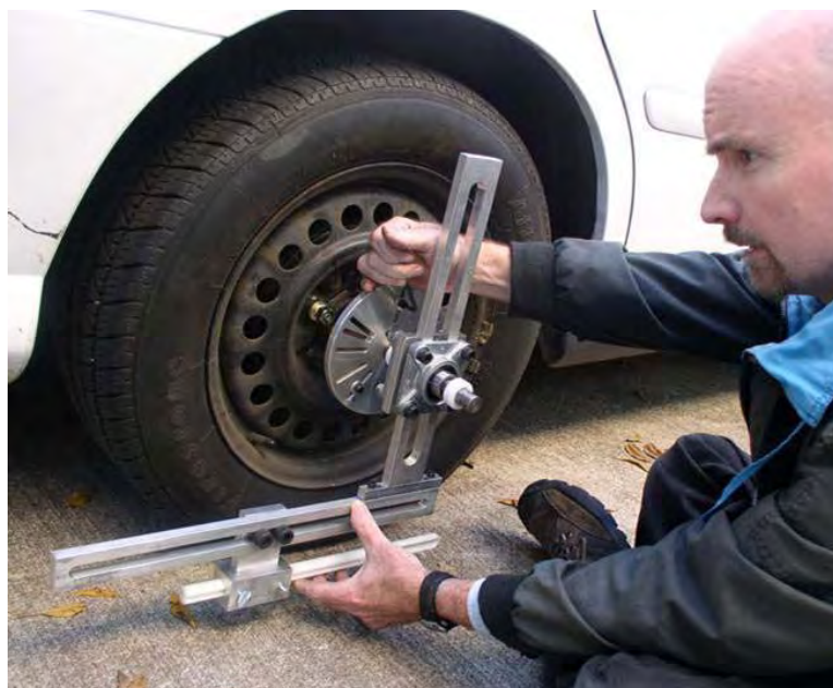
Figure 3.12. OBSI jig being attached to wheel hub on test vehicle
