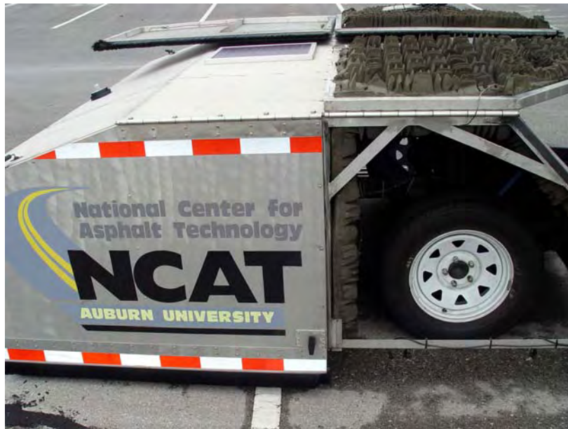
Figure 3.10. Enclosed wheel space and absorptive foam used in NCAT trailer
