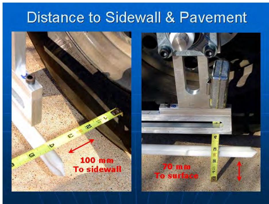
Figure 3.15. Checking the microphone holder distances
