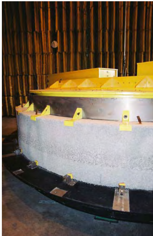
Figure 3. Slab of porous PCC mounted on the apparatus
