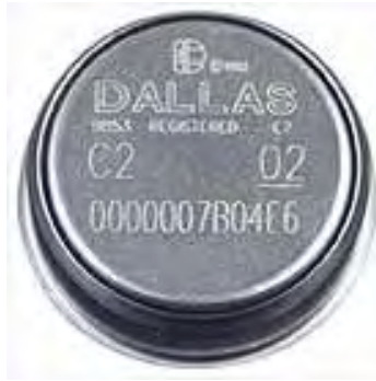
Figure 3.24. Themochron i-Button temperature logging device
