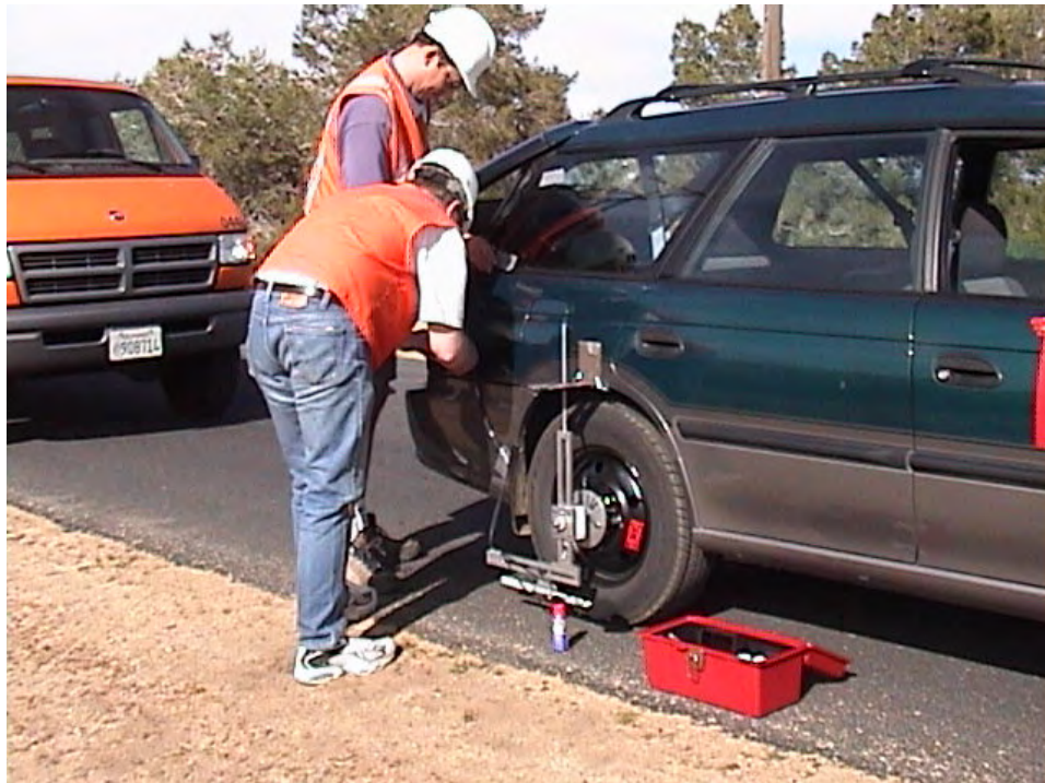
Figure 2.1. Sound intensity fixture being installed on test vehicle
