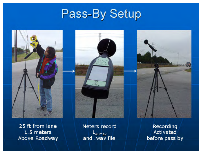
Figure 3.2. SPL Meter Setup for Roadside Measurement
