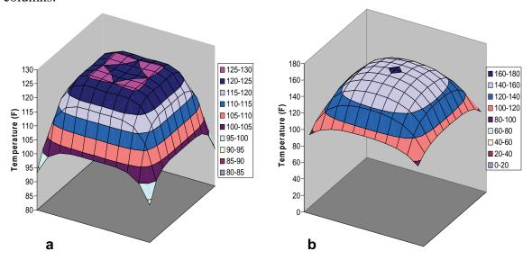
Figure 2.1 Examples of the temperature distribution in a horizontal cross section of a 7ft. by 7ft. column at 24 hours
