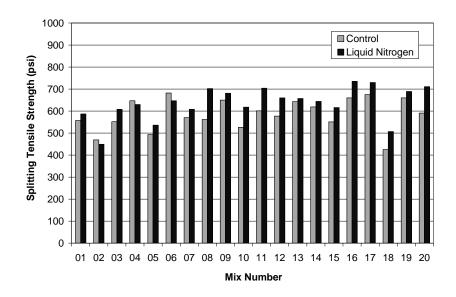
Figure 4.5 28-day splitting tensile strengths for laboratory-mixed concrete
