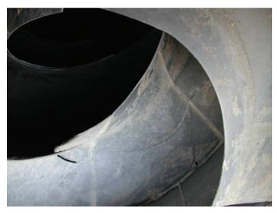
Figure 8.2 Cracking caused by liquid nitrogen dosing on a mixing drum fin
