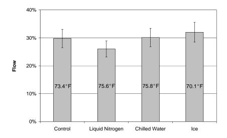
Figure 3.1 Flow of cement mortar containing no admixture
