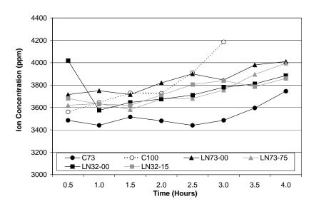
Figure 5.11 Potassium concentrations for six different cement paste mixtures
