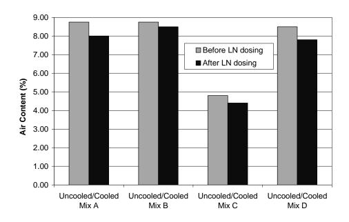
Figure 7.2 Fresh air contents for field-mixed concrete
