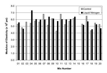
Figure 4.7 Modulus of elasticity comparison for control and liquid nitrogen mixes
