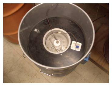
Figure 5.1 Semi-adiabatic calorimeter
