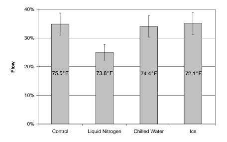
Figure 3.2 Flow of cement mortar containing Pozzolith 200N
