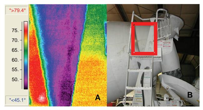
Figure 8.3 Thermal image (A) of a steel mixing drum during liquid nitrogen dosing. In B the area in red indicates the region of a mixing drum that the image is capturing.
