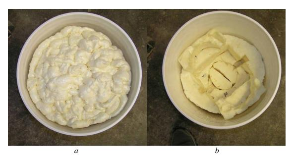
Figure 6.1 Insulating chambers made for set time specimens
