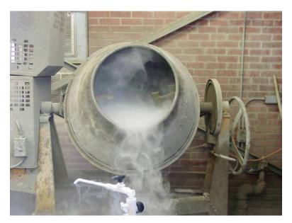
Figure 3.3 Vapor flows freely from the uncovered mixer
