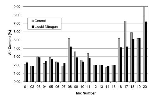
Figure 7.1 Fresh air contents for laboratory-mixed concrete
