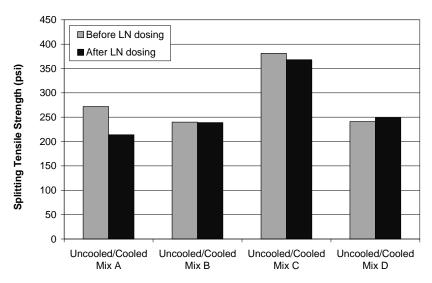
Figure 4.6 Splitting tensile strength for field-mixed concrete
