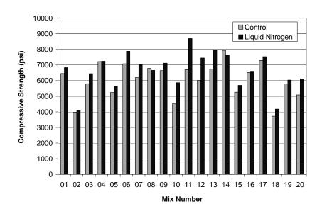
Figure 4.2 28-day compressive strengths for laboratory-mixed concrete
