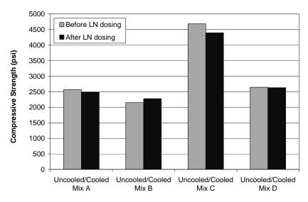
Figure 4.4 28-day compressive strengths for field-mixed concrete
