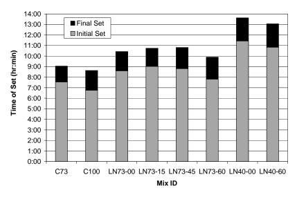
Figure 6.6 Initial and final set times for concrete mixtures delayed dosing mixtures
