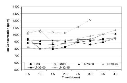
Figure 5.10 Sulfur concentrations for six different cement paste mixtures
