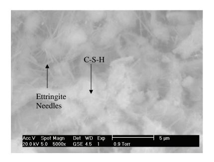
Figure 5.16 ESEM image of fractured cement paste surface from mixture LN32-00 after 24 hours of hydration
