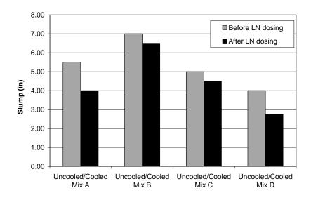
Figure 3.7 Slump results for field-mixed concrete
