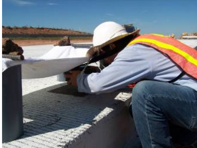
Figure 2.8: Surface temperature measurement within sun screen
