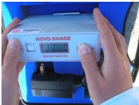
(c) Calibration of 100 percent reflectance
