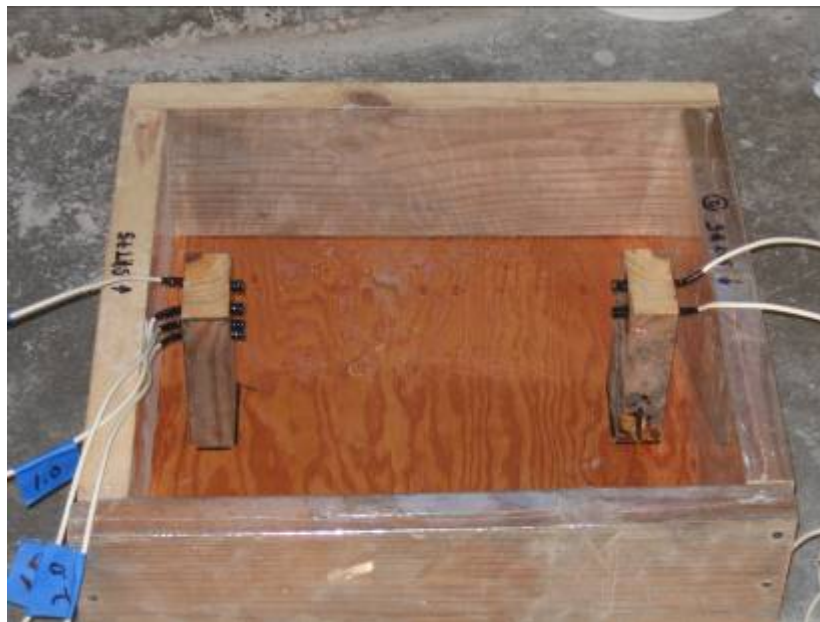
Figure 2.41: Concrete panel with relative humidity sensor
