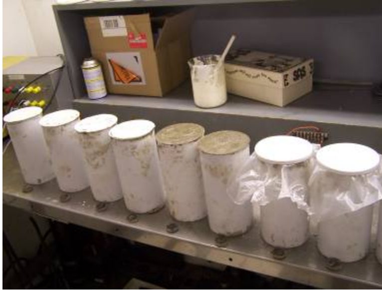
Figure 2.25: Cylinder specimens with different application time of curing compound
