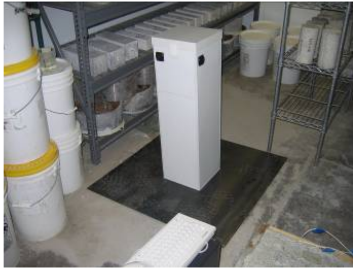
Figure 2.40: GPR unit (SPOT) with reference metal plate
