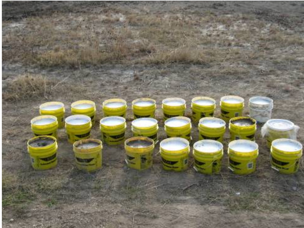
Figure 2.36: Concrete specimens with different application times of curing compound
