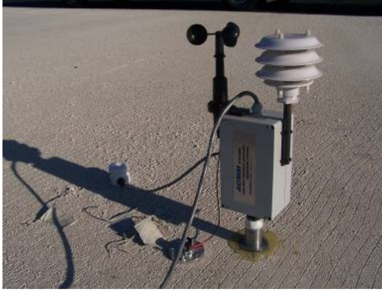
Figure 2.30: Comparison of hygrochron with dew point type humidity sensor (ACMM)
