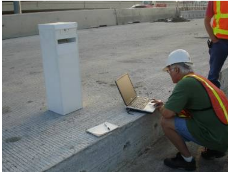
Figure 2.45: Field measurement on dielectric constant with SPOT
