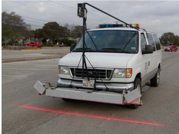
Figure 3.1 TxDOT Pavement Survey Vehicle
