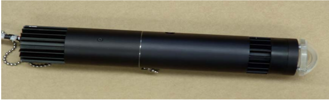
Figure 2.2 Laser Line Projector
