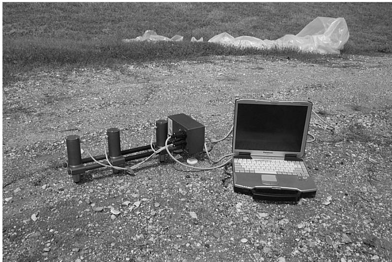
*Figure 2.15. PSPA components and data acquisition system.*
