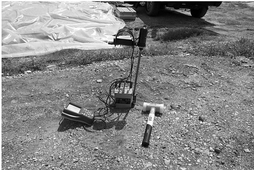
*Figure 2.3. The PANDA dynamic cone penetrometer*
