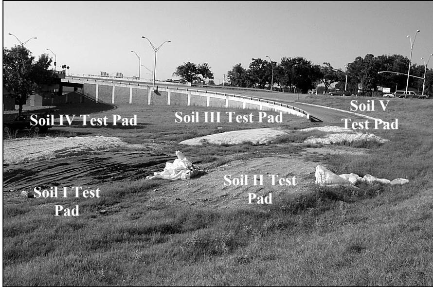
Figure 3.5. Compacted field test pads for Field Study 1
