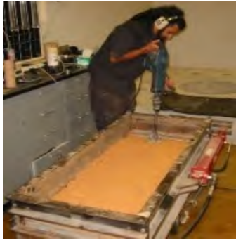
a) Compaction of soil in layers
