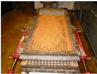
d) Soil compaction on top of the clamped geogrid
