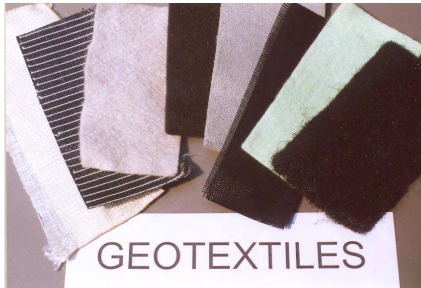
Figure 2.2: View of different types of geotextiles
