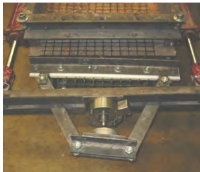
a) Load cell to measure pullout force
