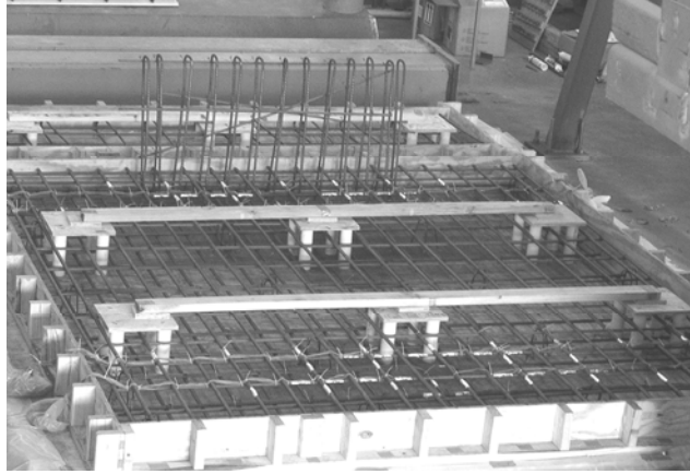
Figure 3.2: Reinforcement layout of the T203 bridge deck and cast-in-place barrier test specimens
