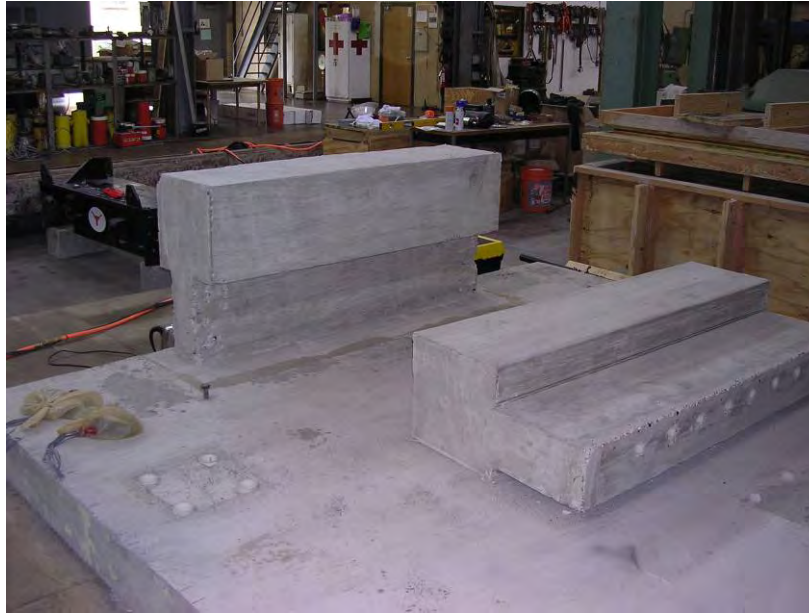
Figure 4.10: Cast-in-place and retrofit T203 bridge barrier specimens
