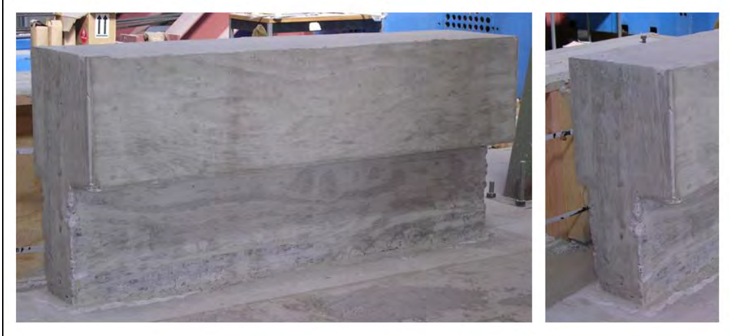
Figure 6.2: Cast-in-place laboratory specimen representing a segment of a TxDOT T203 barrier with continuous base and concrete parapet
