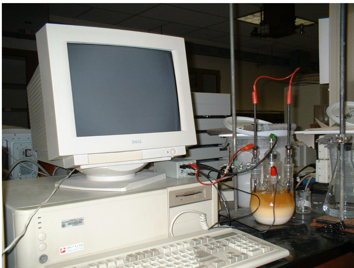
Figure C.2.2. Set-up for Electrochemical Tests showing steel in the winter-grade PuriNOx.
