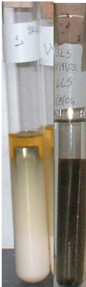
Figure C.2.1. Photograph of a steel specimen in summer-grade PuriNOx (left) and TxLED (right)
