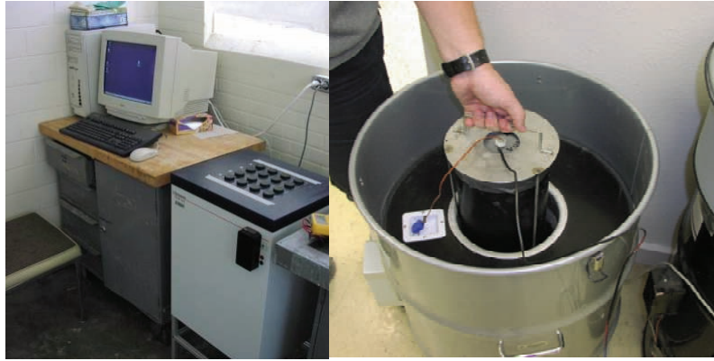
Figure 2.4 Isothermal Calorimeter (Left) and Semi-Adiabatic Calorimeter with Concrete Sample (Right)
