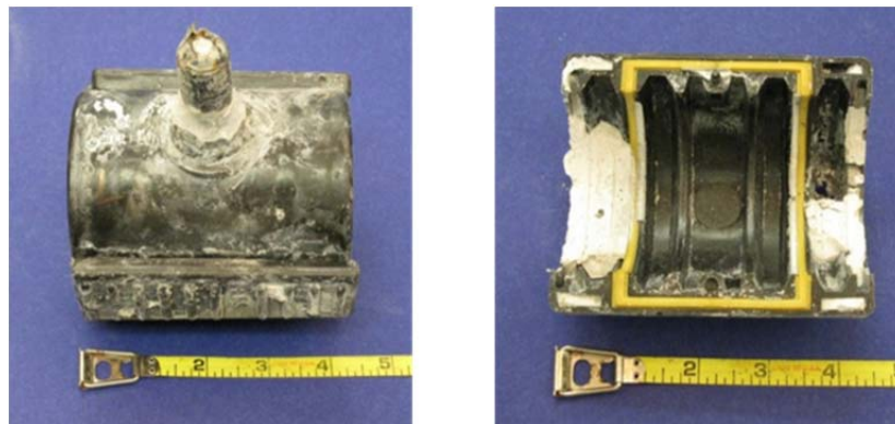
Figure 5.66: Specimen 4.2 Coupler Outer Surface (Left) and Lower Gasket Breach (Right)
