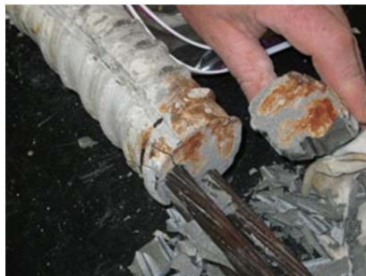
Figure 5.24: Corrosion Staining Within South Grout
