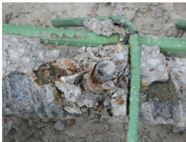
Figure 5.30: Specimen 2.2, Corrosion Staining Under North Grout Vein
