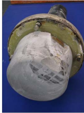
Figure 5.77: Specimen 7.1 Dead End Grout Cap Showing Grout Discontinuity
