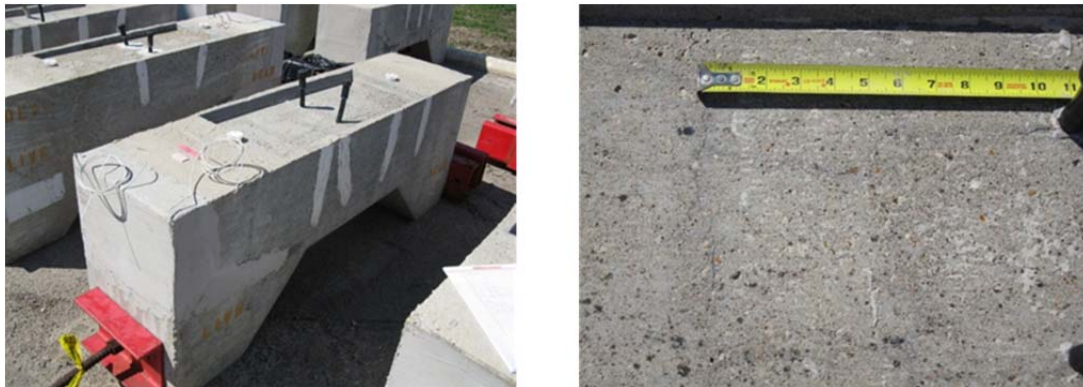
Figure 5.59: Specimen 3.4 Overall (Left) and Discoloration around Surface Cracks (Right)
