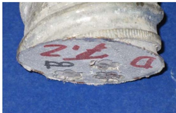
Figure 5.20: Specimen T.2, Debonded Strands in South Anchorage
