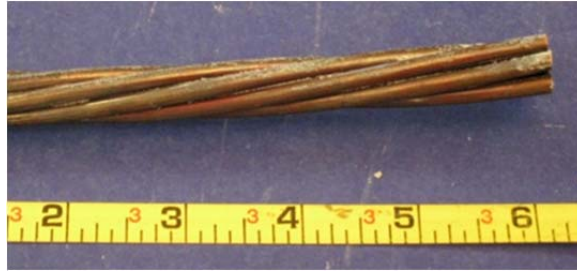
Figure 5.25: Specimen 1.2, Possible Dezincification
