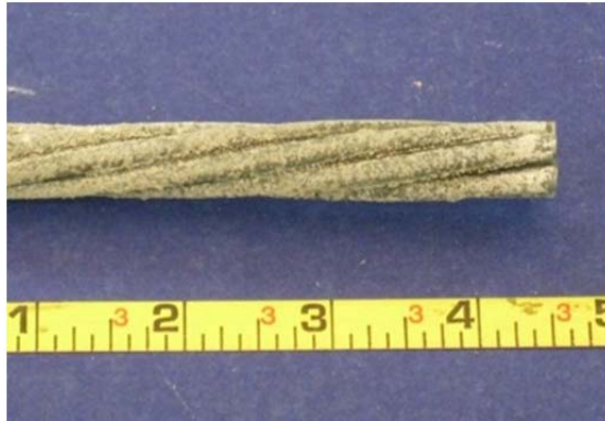
Figure 5.52: Specimen 3.2, Bubbles in Interstices of Galvanized Strand
