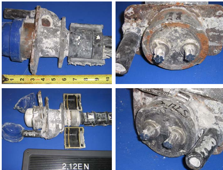
Figure 5.64: Beam 2.12 East End Anchorages (Dripped End)-South Duct Anchorage (Top, Left and Right), and North Duct Anchorage (Bottom, Left and Right)
