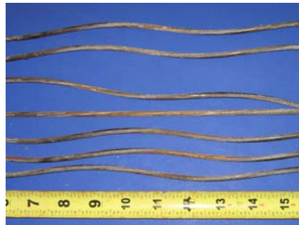
North Duct Strand
