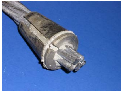
South Duct Strand with Wedges
