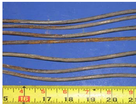
North Duct Strand
