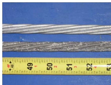
Figure 5.45: Autopsied Galvanized Strand (Bottom) versus New Galvanized Strand (Top)
