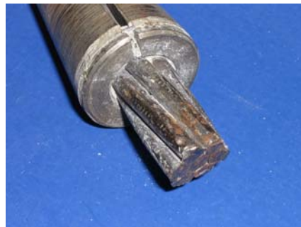
North Duct Strand With Wedges
