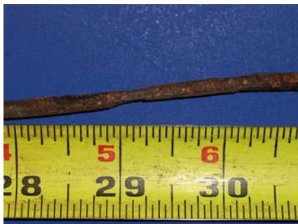
Single Wire from South Duct Strand
