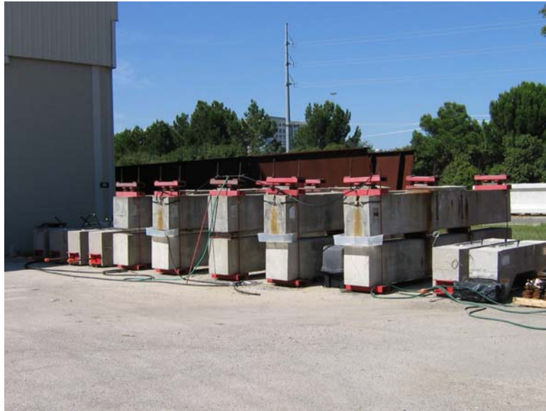
Figure 3.1: Phase II Beams under Exposure Testing
