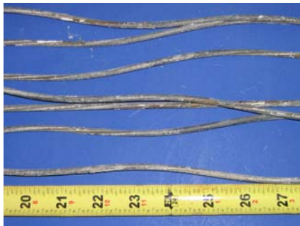
South Duct Galvanized Strand
