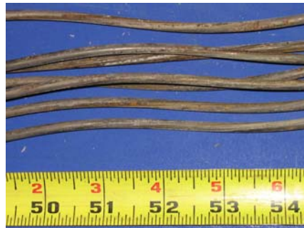
North Duct Strand
