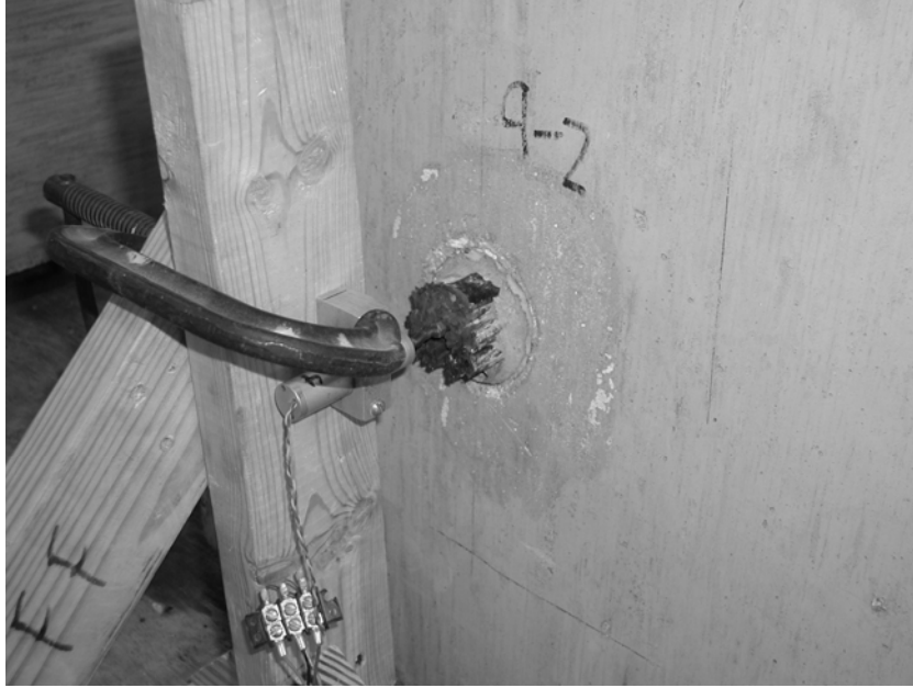
Figure 4-12 Dead End Linear Potentiometer Placement
