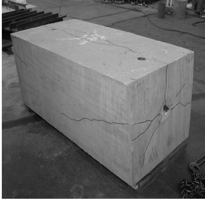
Figure 5-40 Profile of Specimen 2-GD-7.5°-1 after Testing
