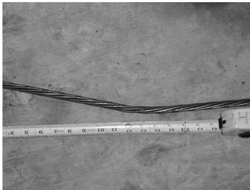
Figure 5-95 Sharp Kink in Strand after Friction Testing
