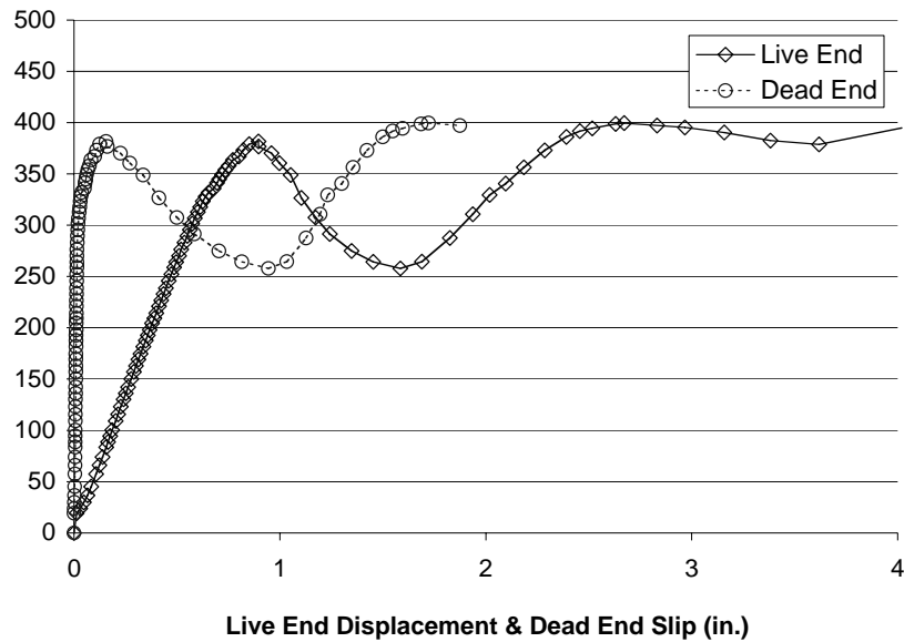
Figure 5-23 Live End Load-Displacement and Dead End Load-Slip Response for Specimen 0-GD-7.5°-1
