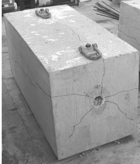
Figure 5-25 Profile of Specimen 0-GD-7.5°-1 after Testing
