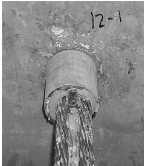
Figure 5-3 Live End of Specimen 0-SP-7.5°-1 after Testing
