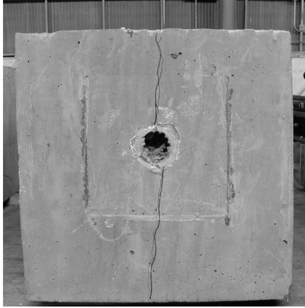
Figure 5-59 Dead End of Specimen 0-HD-7.5°-2 after Testing
