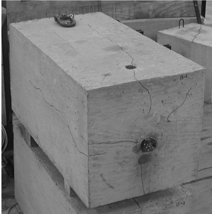
Figure 5-34 Profile of Specimen 1-GD-7.5°-1 after Testing
