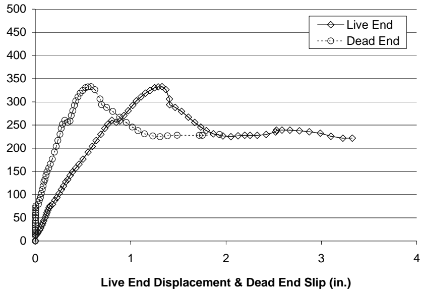
Figure 5-82 Live End Load-Displacement and Dead End Load-Slip Response for Specimen 1*-HD-7.5°-2
