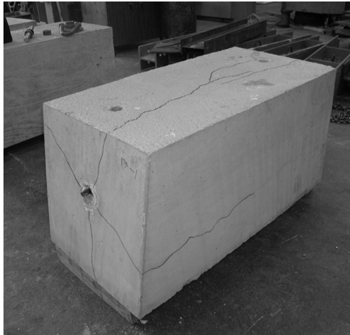
Figure 5-72 Profile of Specimen 2-HD-7.5°-1 after Testing
