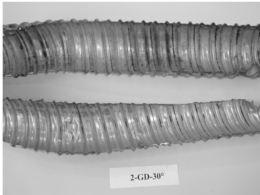
Figure 5-102 Duct from Specimen 2-GD-30° after Testing
