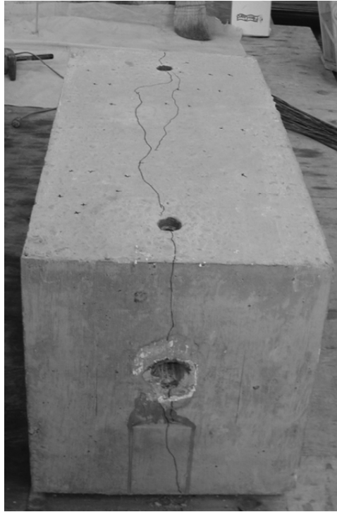
Figure 5-28 Photo of Specimen 0-GD-7.5°-2 after Testing
