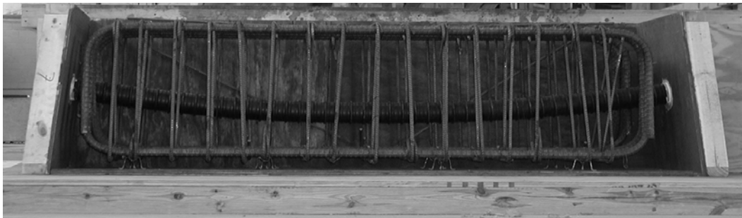
Figure 4-5 Assembled Specimen Cage, Duct, and Formwork
