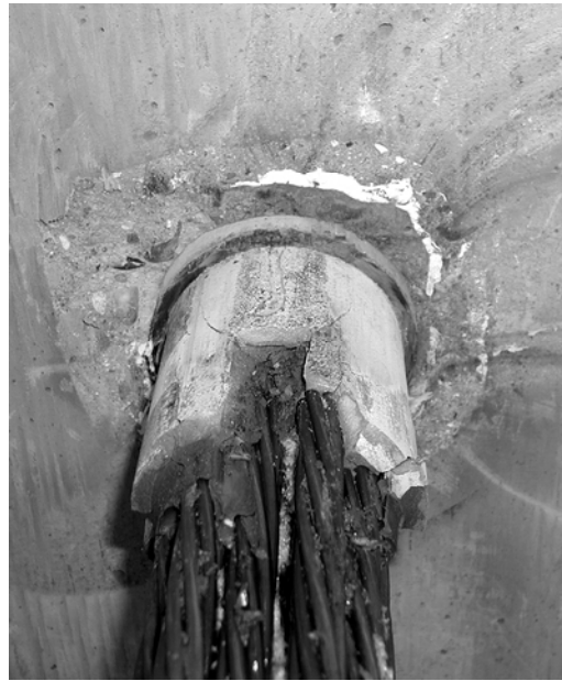
Figure 5-16 Live End of Specimen 1-SP-7.5°-2 after Testing
