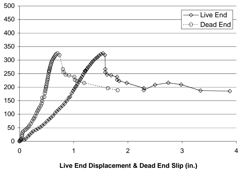
Figure 5-67 Live End Load-Displacement and Dead End Load-Slip Response for Specimen 1-HD-7.5°-2
