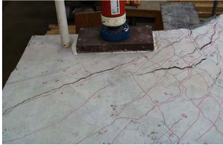
Figure 7.10 Failure of simulated 0° skewed UTSE overhang: Top view of slab, facing north
