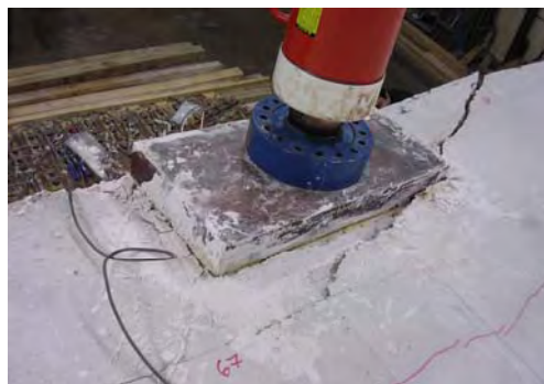
(a) 6-in. top reinforcement spacing
