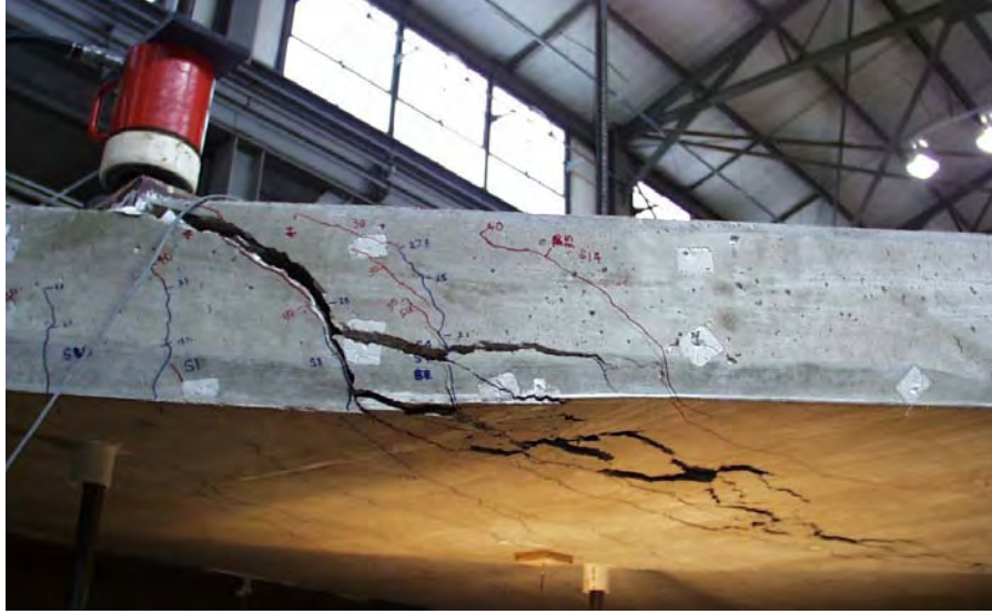
Figure 6.1 Shear failure: IBTS detail, positive-moment test, 45° skew
