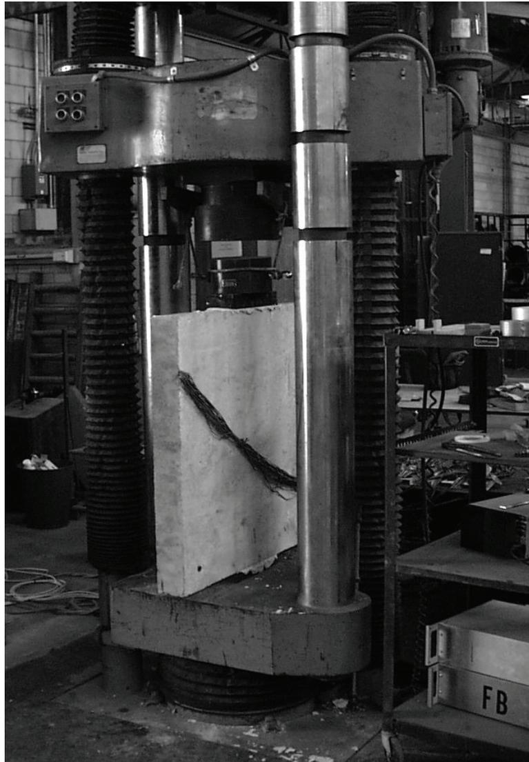
Figure 3-3: Testing of an isolated strut specimen
