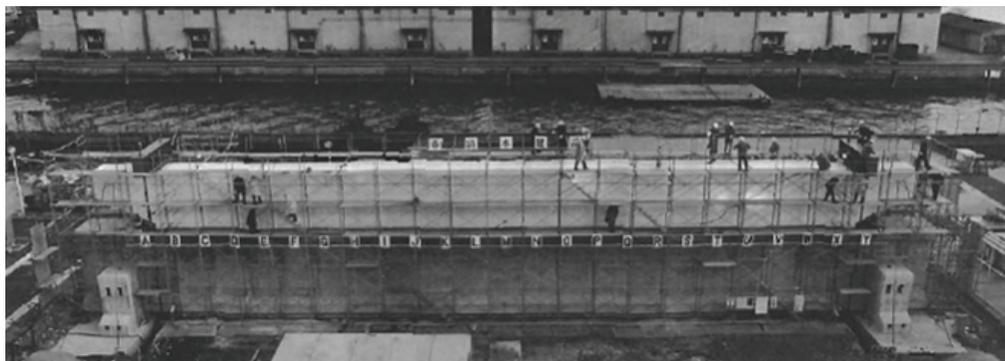
Figure 5-5: Photograph of the largest beam test by Shioya ( $d = 118$  in.)
