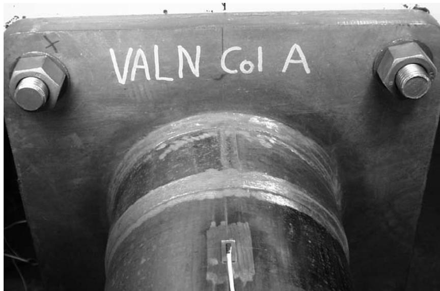
Figure 3.8 External Collar Stiffened Specimen
