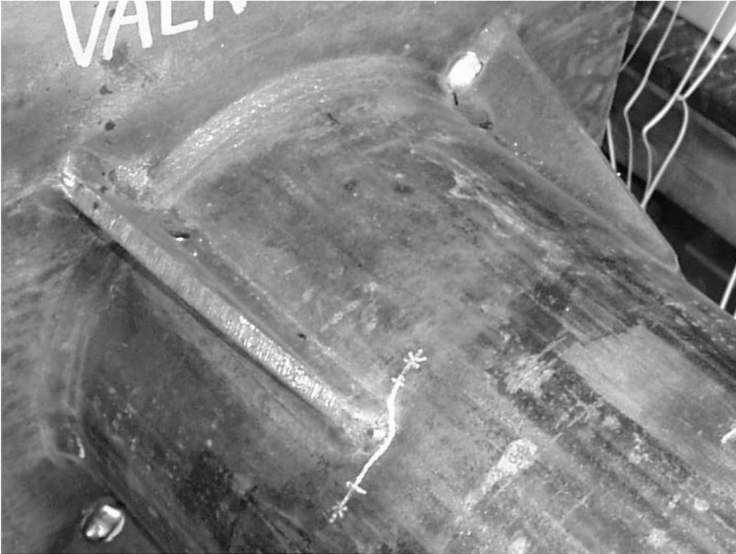
**Figure 7.11 Failure of VALN 6x3/8@45 Specimen – Painted line indicates extent of visible cracking, specimen tested at 6 ksi stress range**
