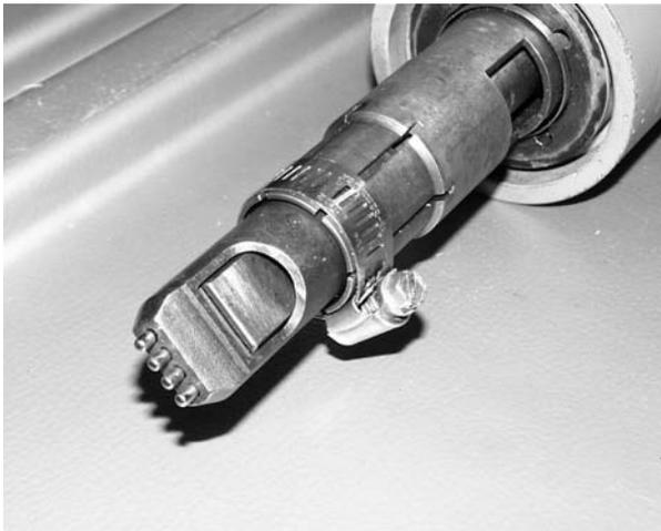
**Figure 10.4 View of Pins on UIT Tool Head**
