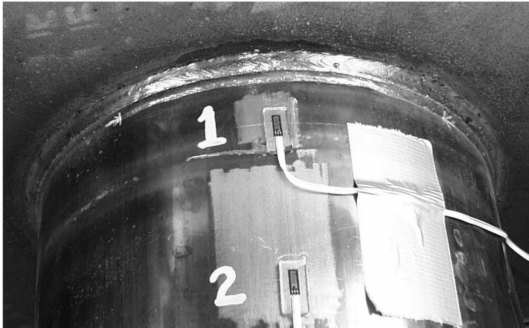
**Figure 7.31 Failure of Full-Penetration Welded Connection Detail Specimen – Paint arrows indicate extent of visible cracking**
