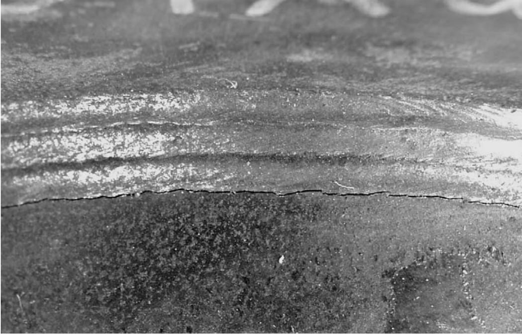
**Figure 7.1 Failure of Socket Weld Connection Specimen**
