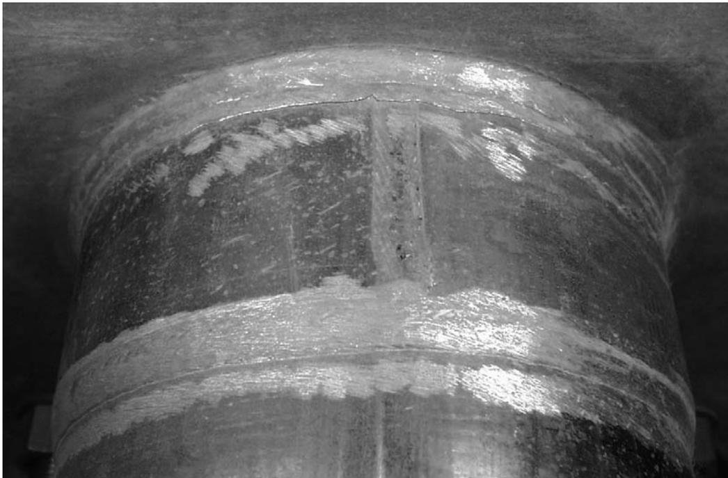
**Figure 7.27 Failure of Externally Stiffened Collar Specimen**
