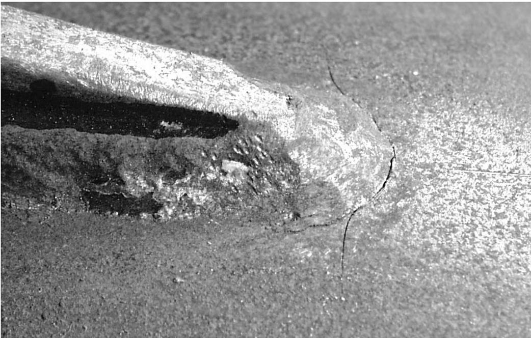
**Figure 7.5 Failure of VAL 6x3/8 Specimen**
