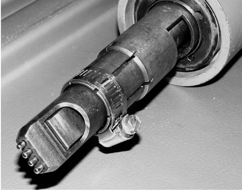
**Figure 6.15 UIT Treatment Tool Head**
