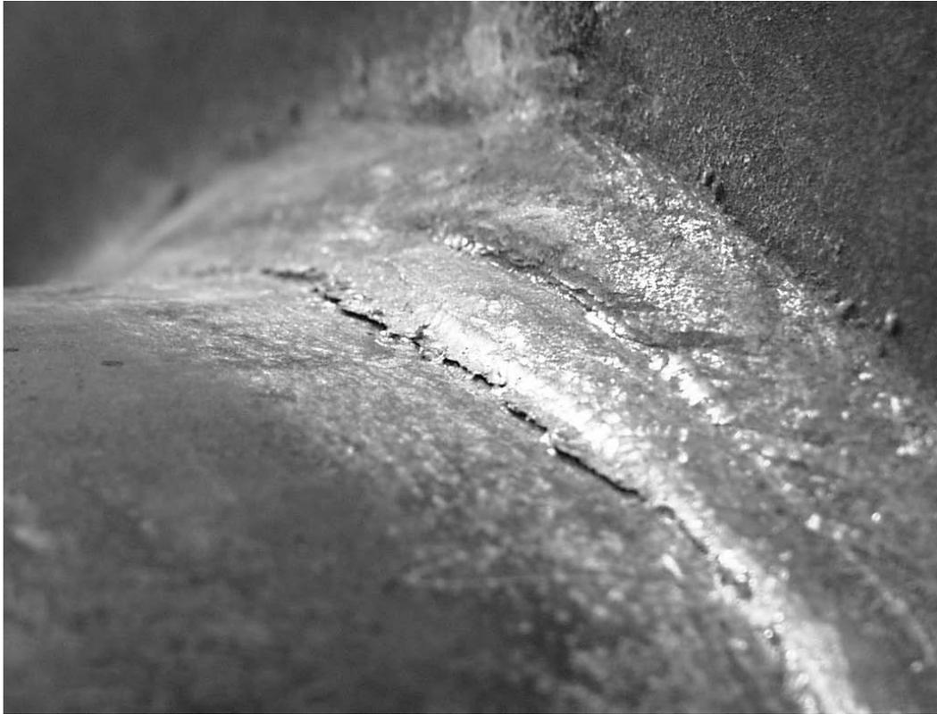
**Figure 7.15 Failure of UIT Treated Socket Connection Specimen**
