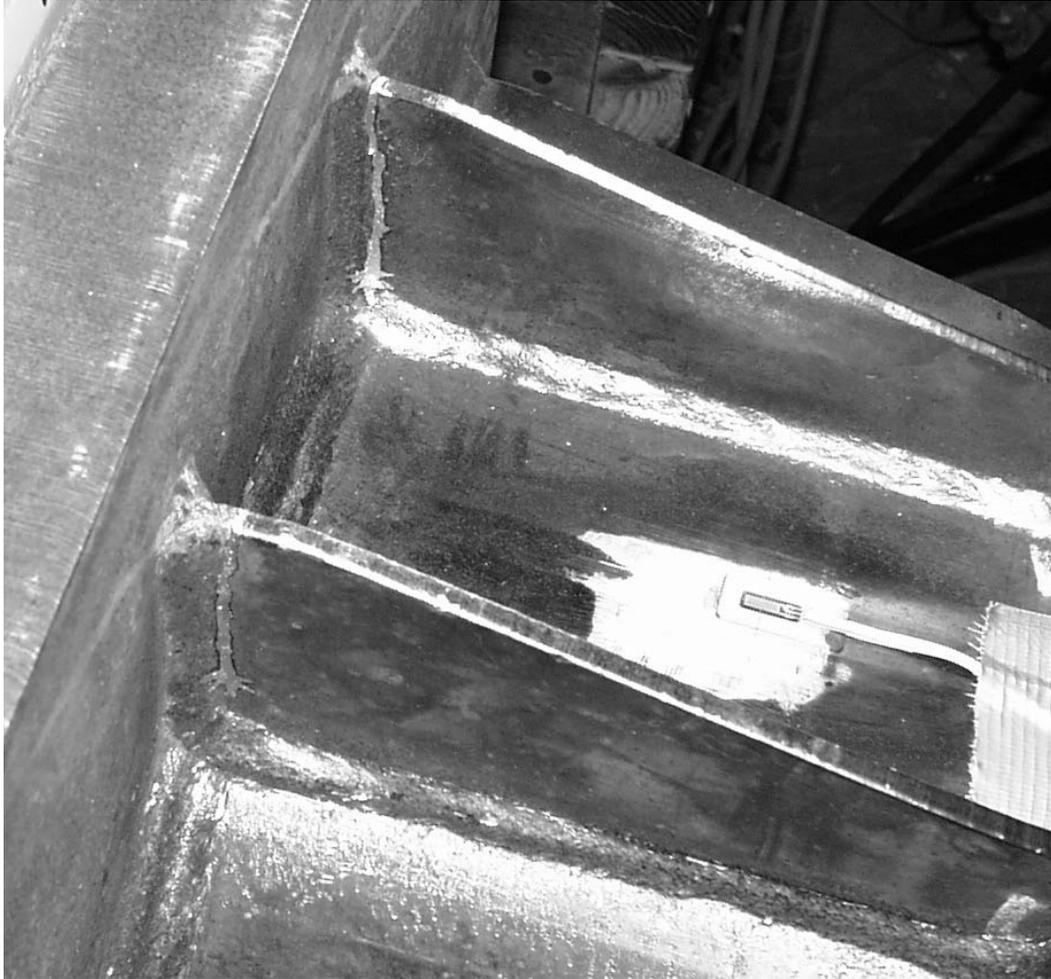
**Figure 7.24 Failure of U-Rib Stiffened Specimen – Note: Painted lines represent extent of visible cracking**
