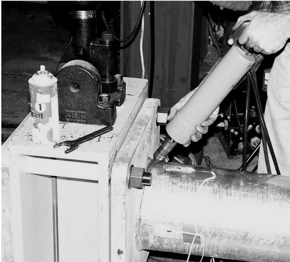
**Figure 6.16 UIT Treatment in Progress**
