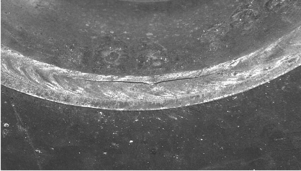
**Figure 7.28 Crack Observed in Interior Weld of External Collar Stiffened Specimen**
