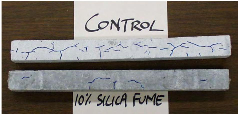
*Figure 3 - ASTM C 1260 Specimens Showing the Ability of Silica Fume to Control Cracking*
