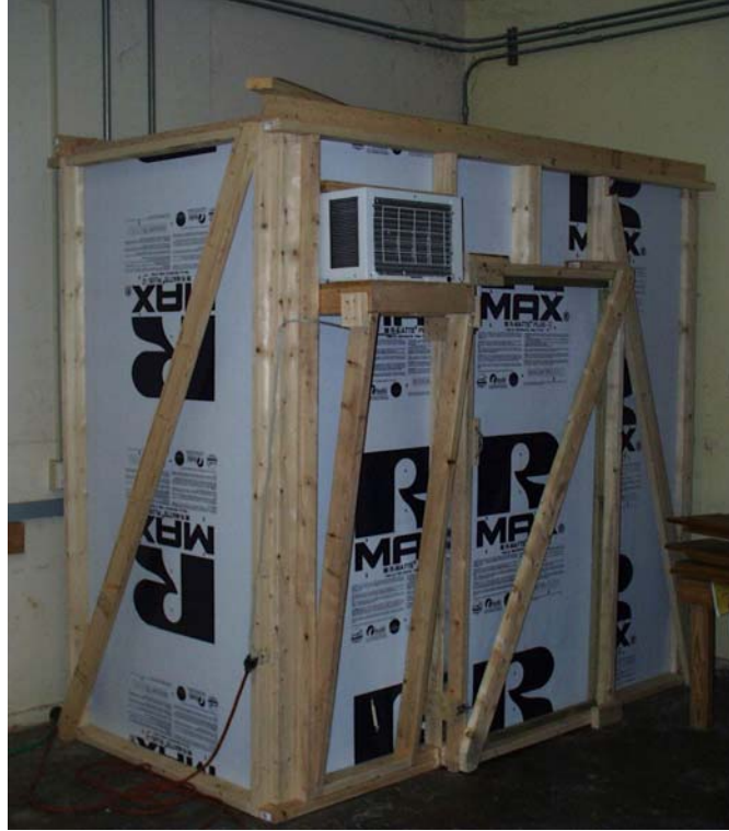
Figure 4.8 Environmental chamber used in controlled pilot tests
