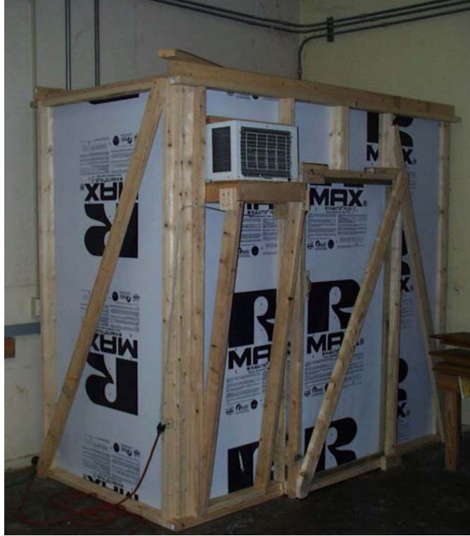
Figure 3.8 Environmental chamber used in controlled pilot tests
