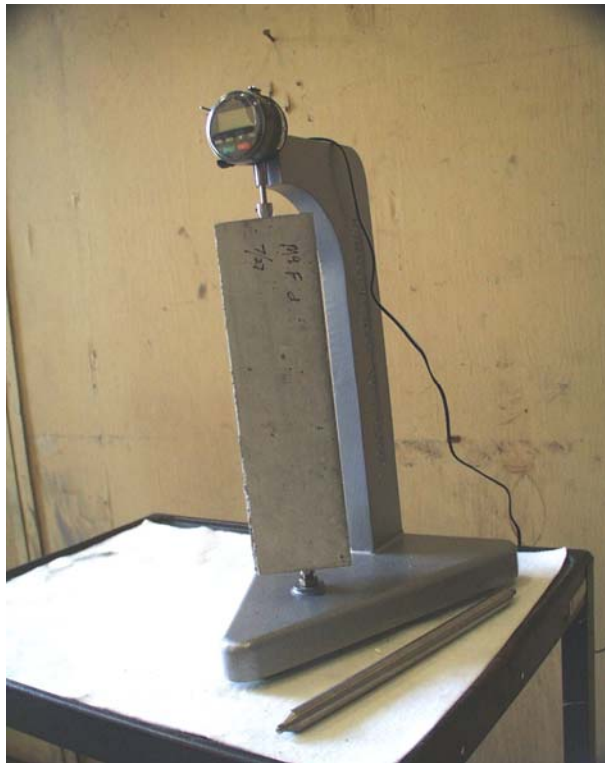
Figure 3-2 Length reading taken with length comparator
